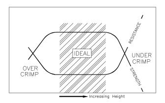
The figure above illustrates the relationship between crimp height and two important terminal parameters: electrical resistance and mechanical (tensile) strength. As crimp height decreases, electrical resistance goes down while tensile strength goes up. At some point, both parameters level off showing that further crimping doesn't make the joint any better. Continued reduction in height will eventually upset the strands too much. Strength goes down and electrical resistance starts to go up.
