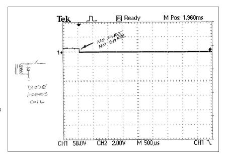
Common practice for years has been to place a diode across the contactor's coil that would conduct heavily and stop this spike from propagating out to the rest of the system. Here's what happens when you add the diode. Here I used one of our plain-jane toggle switches to control the contactor. Notice in the figure above that nothing noteworthy happens when the switch opens. Voltage across the coil falls to zero and stays there. No fire, no spike.
