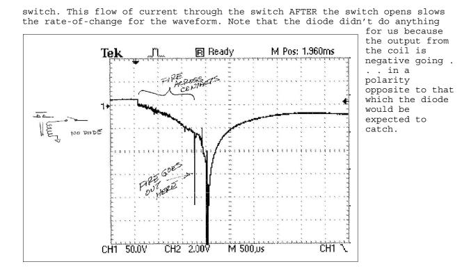
Hmmmm . . . just for grins, let's take the diode off completely and leave the toggle switch in place. Here's what we get:
