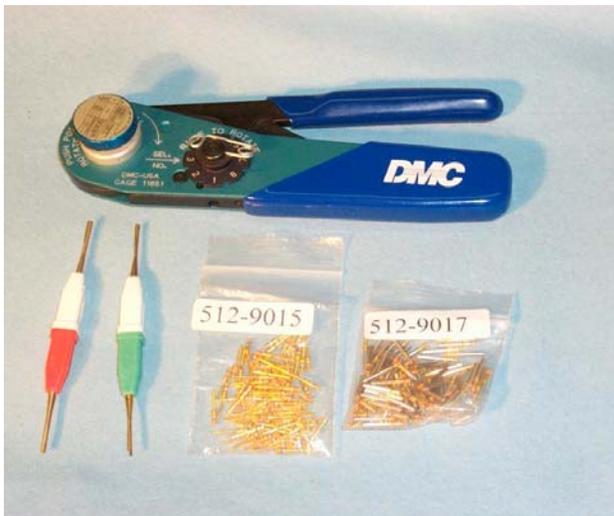
***Daniels and others make some fine tools . . . most conform to industry and military specifications for the installation of machined pins for d-sub, AMP circular***
