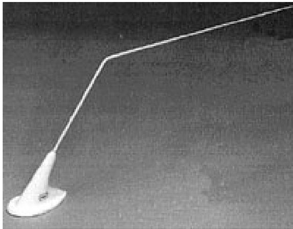
The antenna shown above is the AV17 from Aircraft Spurce and is commonly seen on Van's designs.
