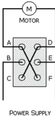
Pitch, Roll and Flap motors can be connected directly to the powerboard at the terminals provided. Pitch and Roll trim are 12 volts regulated at up to 10 Amps and is suitable for using 12 volt MAC servos (or similar) in 12 or 24 volts systems. The Flap circuit uses ship's power and assumes the flap motor is the same voltage as the airplane's battery.
