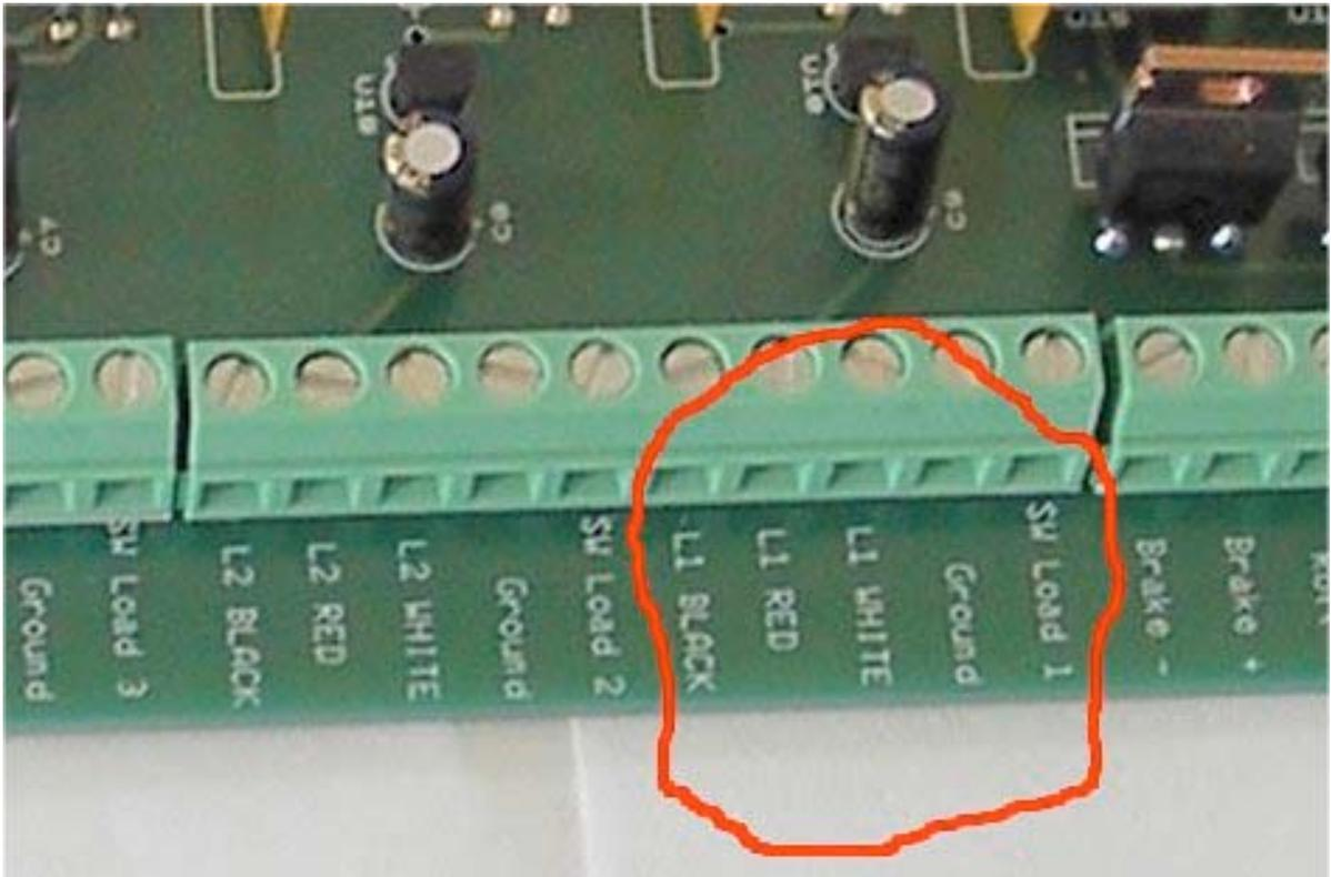
The circled area shows Switched Load 1, which is labeled SW Load 1 and Ground.
