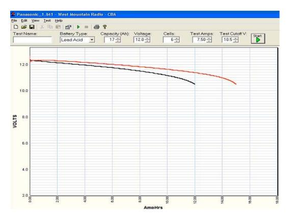
First at 4A (48 watts) and then at 7.5 amps (92 watts). Curves for these two tests are shown here.
