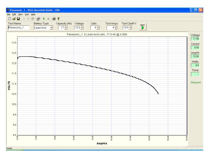
As you can see here, when discharged to simulate a 4A e-bus load, the ol' beast trudged along for 15 a.h. worth of output. Given that it's rated for 17 a.h. under a 20 hour rate, it seems that this battery might still be performing at or near new specifications for capacity in spite of disappointing value of source impedance.
