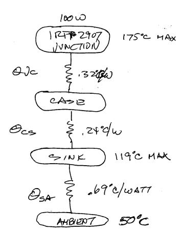
degrees C or a rise of 35C above ambient. 35/92 yields .38 degrees C per watt and the last thermal study says we only need 1.22 degrees C/W. Plenty of headroom. Can we do this with one IRFP2907 transistor? Let's see.
