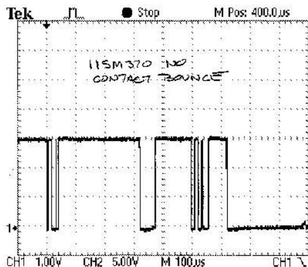
Figure 3. Contact Bounce in SM Series Microswitch
