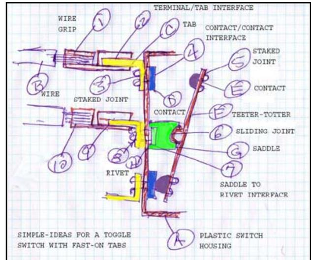
Figure 5. Parts-Count for Electron Flow Through Switch
