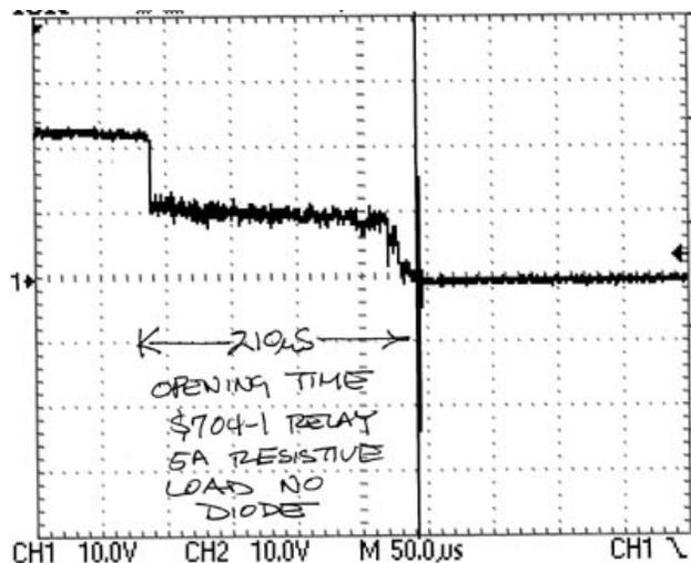
Figure 7. Exemplar Arc Duration No Diode
