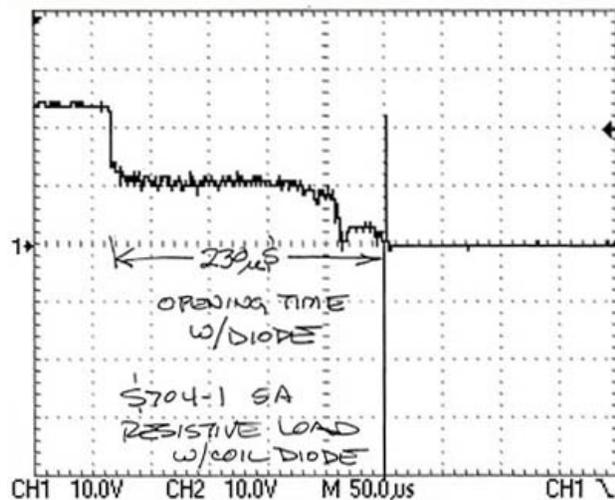
Figure 8. Exemplar Arc Duration with Diode
