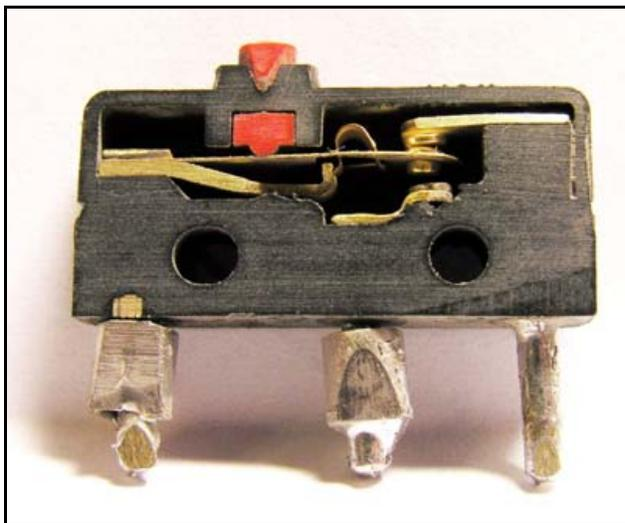
Figure 4. SM Microswitch Cutaway
