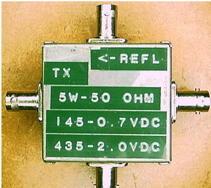
Directional coupler with detectors and DC-output.
