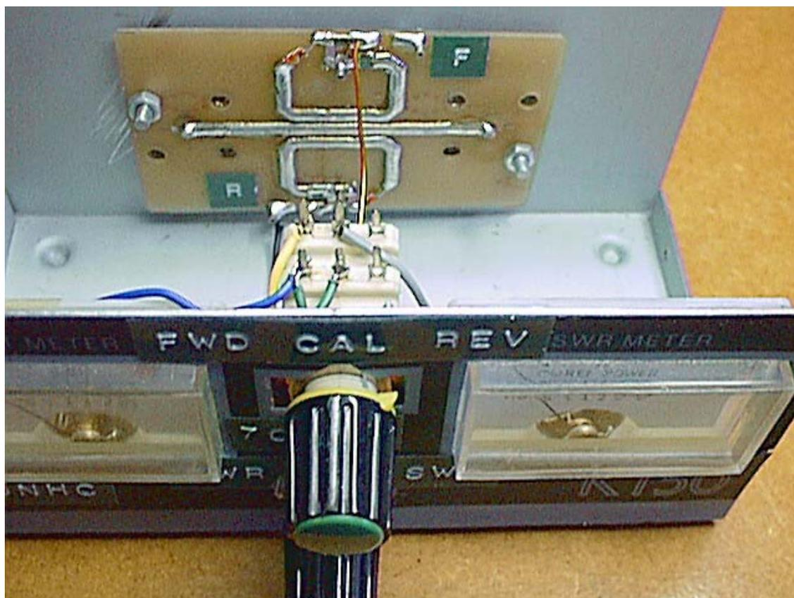
Directional coupler with detectors and DC-output,
