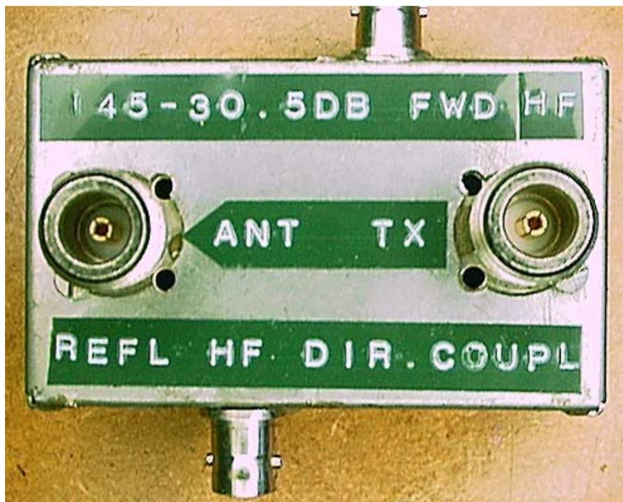
Directional coupler with HF-output, [-30,5dB @ 145MHz](#), [-20dB @ 435MHz](#).
