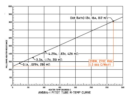
nested in a wad of Fiberglas. This is a relatively small value which I can attribute to the large surface area of the pitot tube. The same experiment in a vacuum would have produced a Theta (heater-to-ambient) value 5 to 10 times larger.
