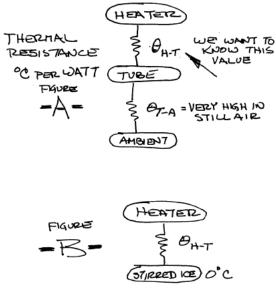
Electrical resistance is quantified in OHMS wherein 1-ohm produces 1 volt of drop when a current of 1 amp flows through the resistor. Thermal resistance in many discussions is given the symbol Theta, a character in the Greek alphabet. Theta is quantified in temperature differential across the resistance when impressed with a known energy flow. In our case, we're going to discuss "degrees-C per watt."
