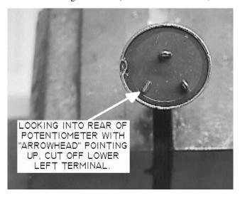
core) to attach wires to terminals on the control potentiometer. Hook wires over the terminals and solder. After joints cool, slide heatshrink pieces over the joints and shrink them down.
