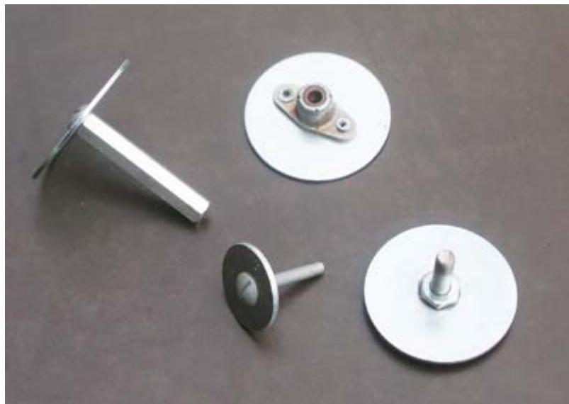
When it's necessary to space a bundle or tube off the surface you can fabricate bonded 'spacer-studs'. One end of an internally threaded stud is attached to the washer and bonded with JB Weld. The components to be suspended are attached to the other end. Consider this process for installing a nut plate where riveting directly to the composite sandwich is problematic.
