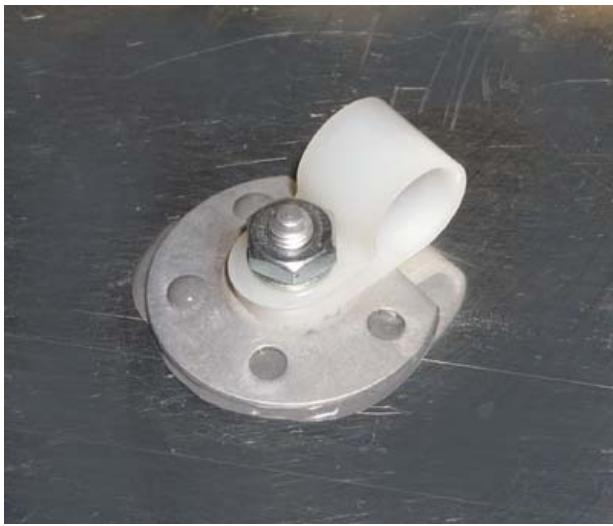
While browsing through a manufacturer's salvage outlet store some years back I discovered a part that consisted of a 10-32 stud welded to a perforated flange about 1" in diameter. With the Click Bond products in mind I purchased a handful and conducted some tests with a variety of off-the-shelf adhesives. The first experiment with JB Weld on thick aluminum produced a very strong bond.
