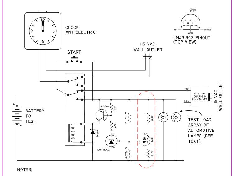
I. THE TEST FIXTURE DESCRIBED ABOVE USES A LATCHING RELAY CONFIGURED TO TEST A BATTERY WITH A LOAD THAT APPROXIMATES THE AIRCRAFT'S BATTERY ONLY ENDURANCE REQUIREMENTS. AN ARRAY OF AUTOMOTIVE LAMPS ARE COMBINED TO ACHIEVE THE DESIRED TEST CURRENT.
