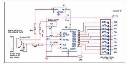
moves up and down with each degree of vane rotation). The lower trimpot is an offset adjustment. This moves the span position (bottom green display element turn on). This bottom LED should be on when the aircraft is in straight and level flight. The upper red light should turn on at the stall angle for your particular aircraft and wing design; a range of between 15 to 40 degrees for most aircraft types.
