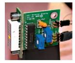
located on the Delrin mount sleeve. The output voltage is used to drive a panel-mounted 10-segment multicolor bar graph display. The display LEDs change position and color from green to yellow to red as the angle of attack increases.
