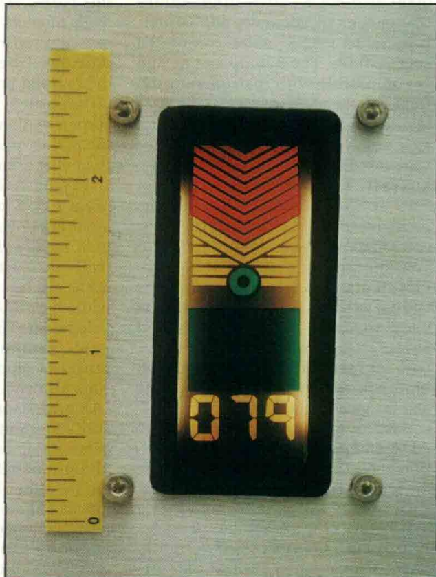
Proprietary Software System's display during an optimum approach with the gear down and an AOA of 7.9 units.
