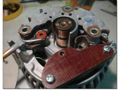
(Left) The mounting block is ¼-inch thick and replaces the regulator after being cut to shape. It's made from two ½-inch thick pieces of canvas Bakelite, epoxied together and holding the nut. (Right) The mounting block attached to the alternator. Put one fiber washer where the left-hand brush-holder terminal was attached.
