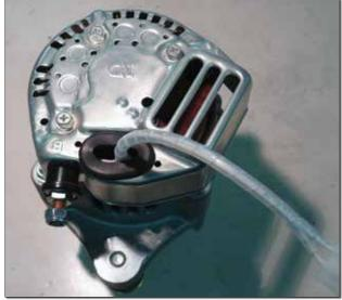
(Left) The brush holder mounted on the alternator with the right-hand new wire under the brush-holder lug. This keeps the brush holder precisely level and only a tiny fraction higher than the original position. (Right) Alternator with terminal shroud reinstalled and wires threaded through a rubber grommet fitted to the rear cover.
