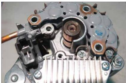
(Left) The brush holder is held in place with two screws. (Right) The alternator after removing the brush holder.
