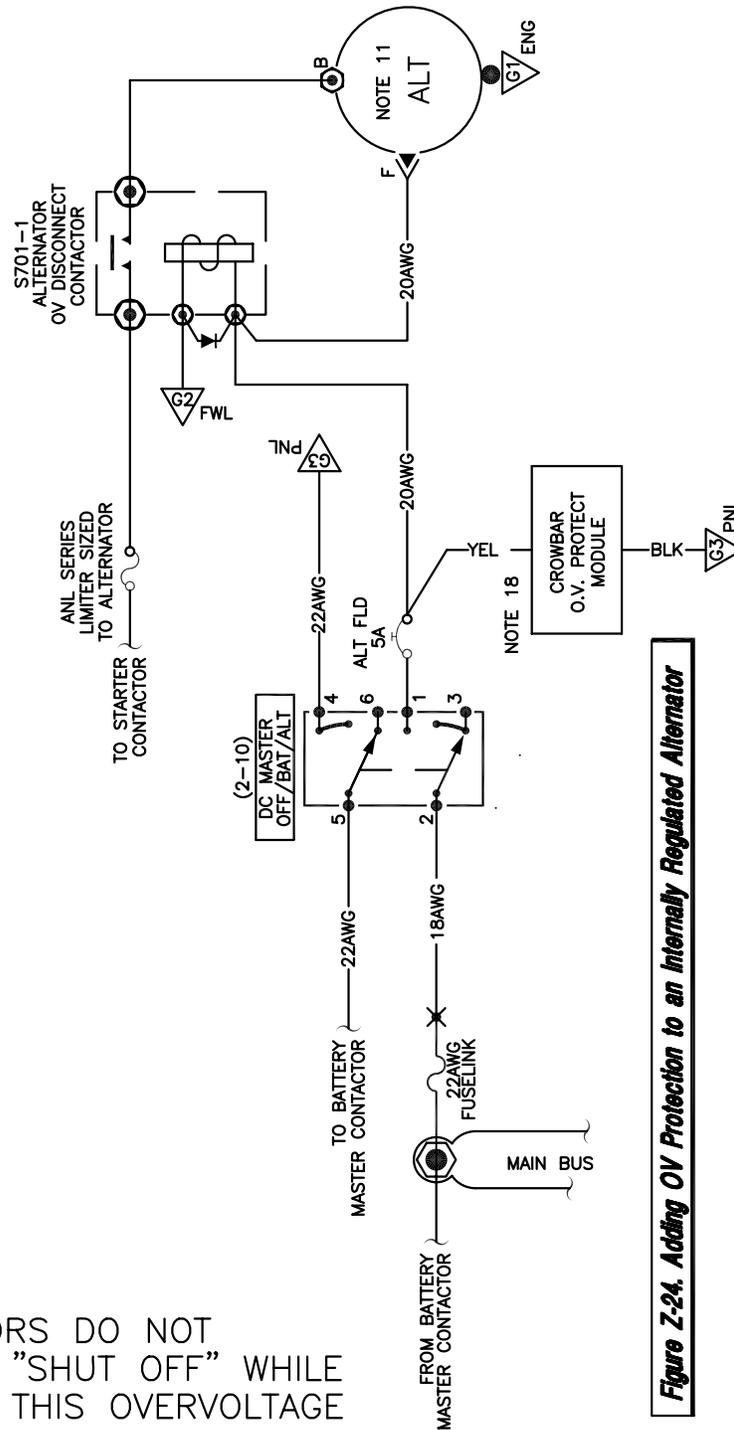
**Figure Z-24. Adding OV Protection to an Internally Regulated Alternator**
