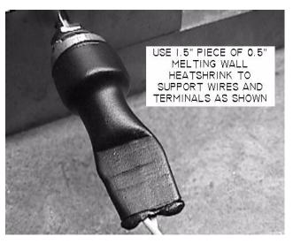
potentiometer... when the heatshrink has reduced to approx 1/4", lightly "squash" the hot tubing with a pair of needle nose pliers so as to close the tube down on the wires. An internal melting sealant will ooze out of the end. Work the end down to fully encase the wires and flatten the tubing as it cools.
