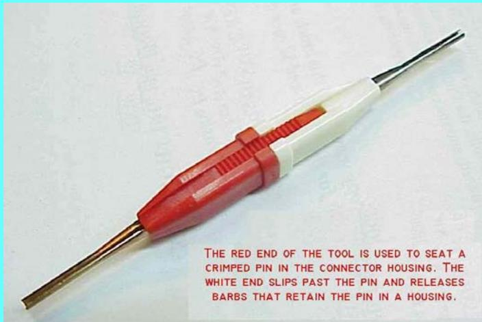
THE RED END OF THE TOOL IS USED TO SEAT A CRIMPED PIN IN THE CONNECTOR HOUSING. THE WHITE END SLIPS PAST THE PIN AND RELEASES BARBS THAT RETAIN THE PIN IN A HOUSING.
