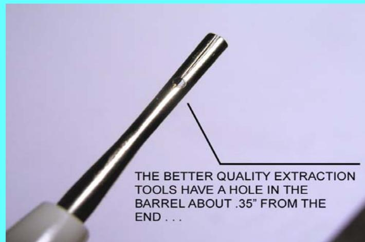
THE BETTER QUALITY EXTRACTION TOOLS HAVE A HOLE IN THE BARREL ABOUT .35" FROM THE END . . .
