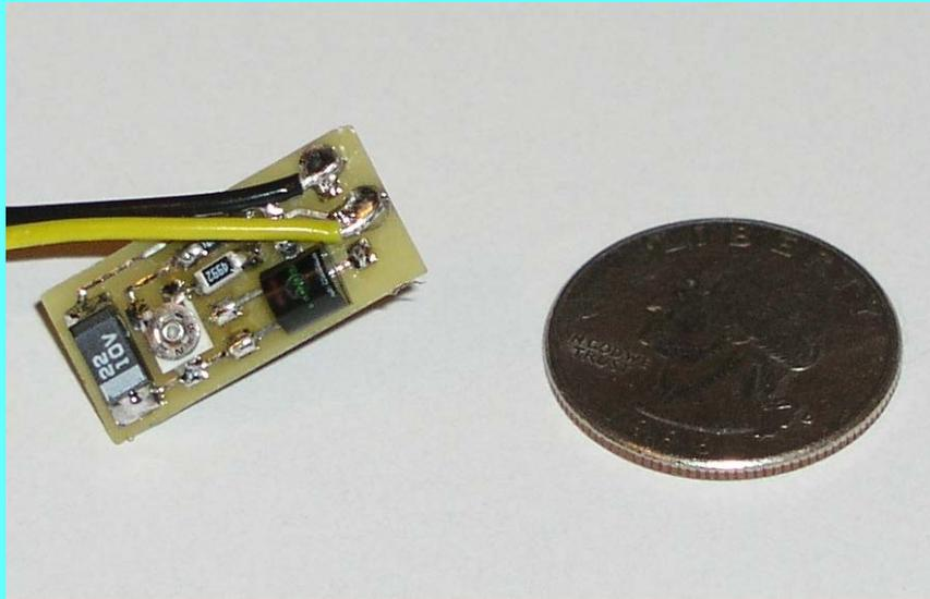
**This is a “Crowbar” OV Protection module offered by AeroElectric Connection and B&C for over 15 years.**
