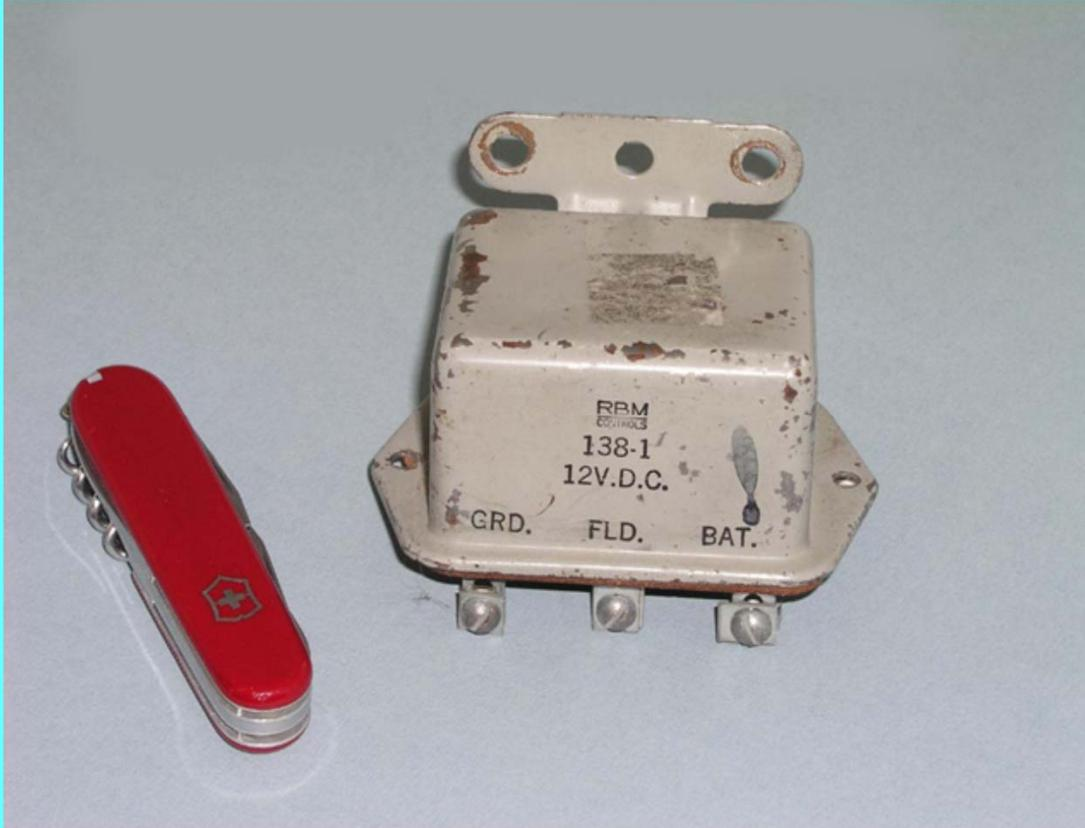
**This device by RBM Controls was the best we knew how to do for Over Voltage protection in 1975.**
