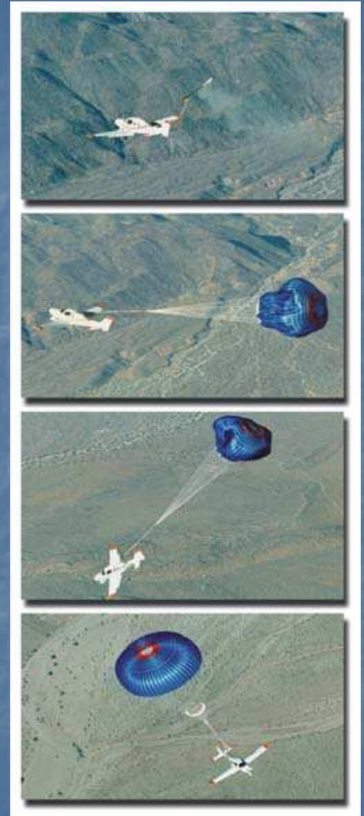
Simplest designs used combinations of springs to eject a drogue which in turn dragged a canopy from the canister on the tail of the aircraft.
