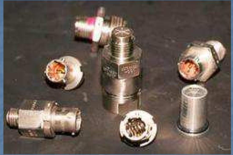
In fact, the energy required to melt a bridge wire in the modern initiator is similar to that required to open a 1A fast blow fuse.
