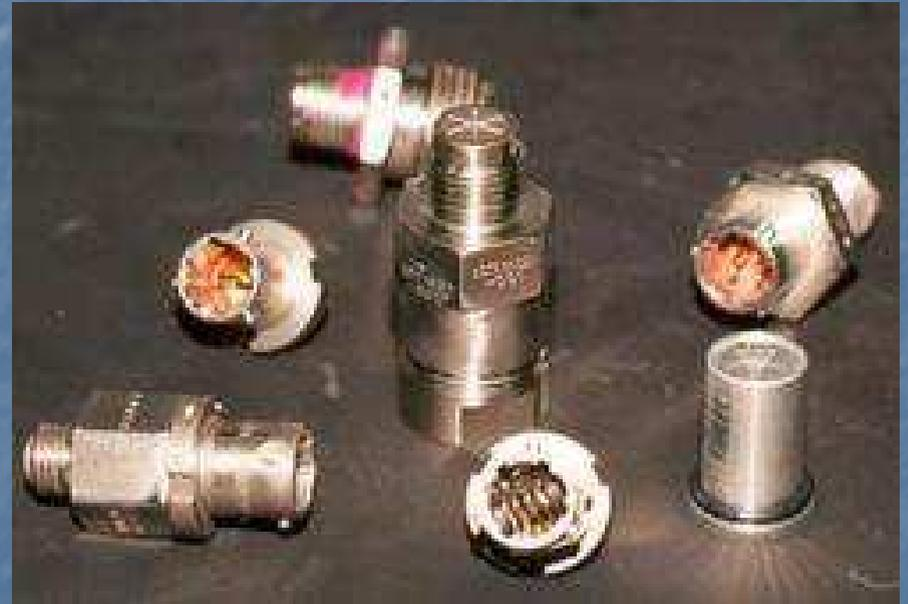
On Premier EEDs were used to initiate ignition of high power gas generator that deployed the parachute from the canister.
