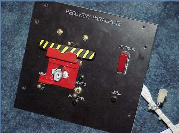
Pilot controls for the parachute system include
