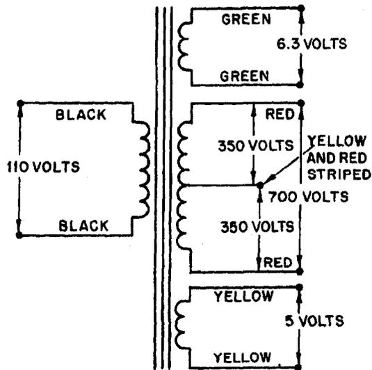
Figure 5-12.—Schematic diagram of a typical power transformer.
