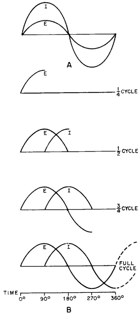
**CAPACITANCE IN AC CIRCUITS**—A capacitor in an ac circuit opposes any change in voltage just as it does in a dc circuit.
