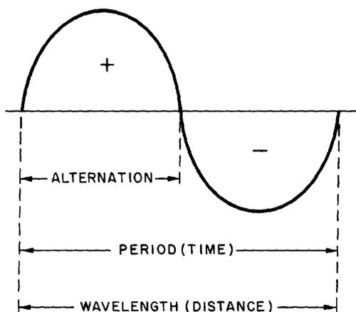
**PEAK AND PEAK-TO-PEAK VALUES**—The maximum value reached during one alternation of a sine wave is the peak value. The maximum reached during the positive alternation to the maximum value reached during the negative alternation is the peak-to-peak value. The peak-to-peak value is twice the peak value.
