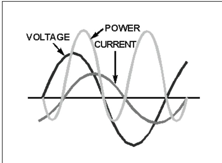
**POWER FACTOR**—The portion of the apparent power dissipated in a circuit is called the power factor of the circuit. It can be expressed as a decimal or a percentage. The formulas for power
