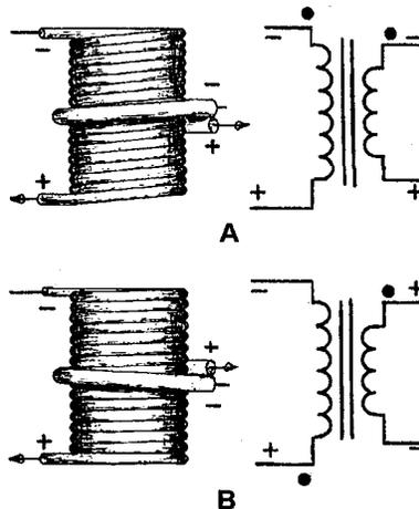
**TURNS RATIO**—The **TURNS RATIO** of a transformer is the ratio of the number of turns of wire in the primary winding to the number of turns in the secondary winding. When the turns ratio is stated, the number representing turns on the primary is always stated first. For example, a 1:2 turns ratio means
