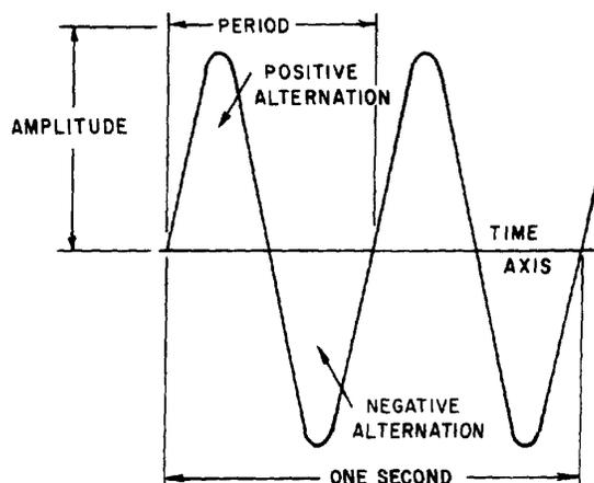
**WAVELENGTH**—The period of a sine wave is defined as the time it takes to complete one cycle. The distance the waveform covers during this period is referred to as the wavelength. Wavelength is indicated by lambda ( $\lambda$ ) and is measured from a point on a given waveform (sine wave) to the corresponding point on the next waveform.
