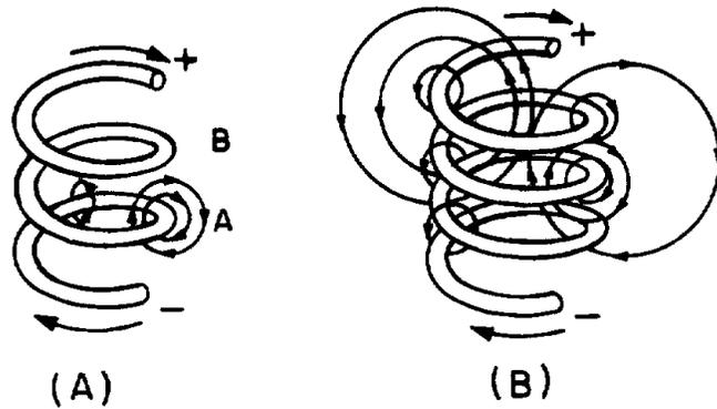
**FACTORS AFFECTING COIL INDUCTANCE**—The inductance of a coil is entirely dependent upon its physical construction. Some of the factors affecting the inductance are:
