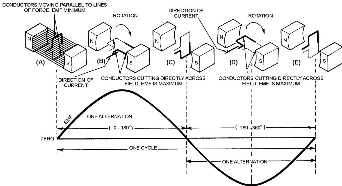
**FREQUENCY**—The number of cycles of ac per second is referred to as the FREQUENCY. AC frequency is measured in hertz. Most ac equipment is rated by frequency as well as by voltage and current.
