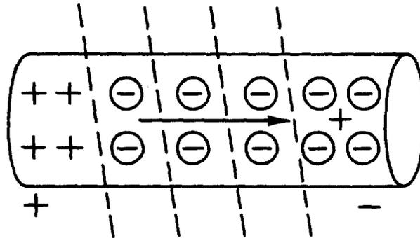
The difference between the charges in the conductor is equal to a difference of potential (or voltage). This voltage caused by the moving magnetic field is called electromotive force (emf).
