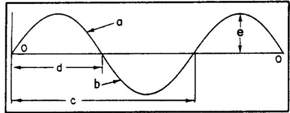
Figure 1C.—Components of a sinewave.
