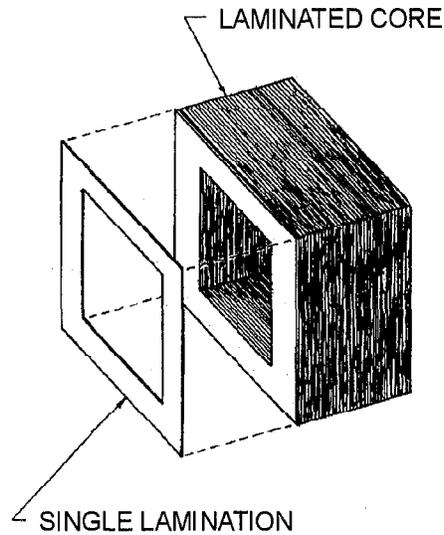
Figure 5-2.—Hollow-core construction.
