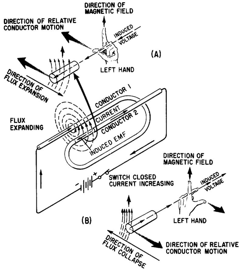
**INDUCTANCE OF A COIL**—The property of inductance can be further increased if the conductor is formed into a coil. Because a coil contains more loops, more of the conductor can be affected by the magnetic field. Inductors (coils) are classified according to core type. The core material is normally either air or soft iron.
