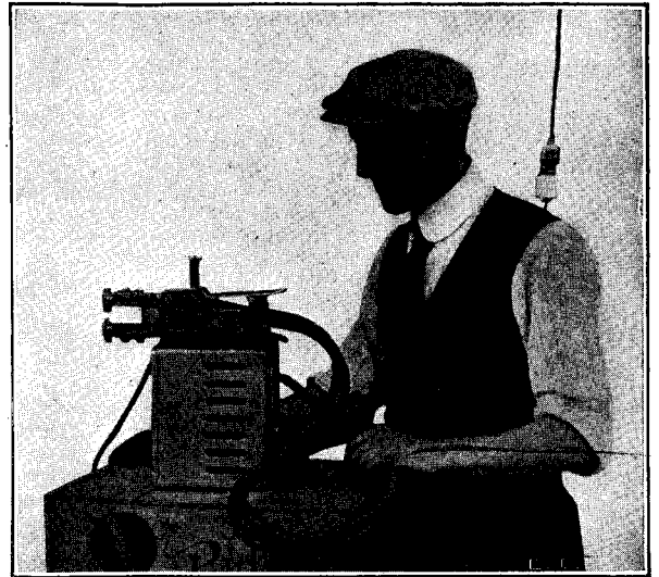
Portable Electric Welder Useful in Sealing Binding Wires on Cases, Barrels, Etc.
