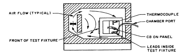
FIGURE 2d. Typical chamber installation.
