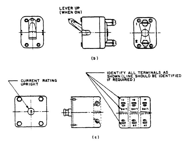
FIGURE 1. Terminal identification.
