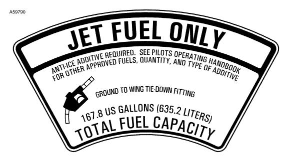
13. Adjacent to each inboard fuel tank filler cap (when installed):
