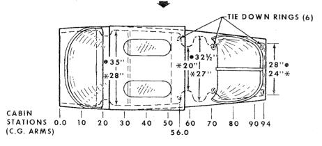
Figure 6-5. Internal Cabin Dimensions
