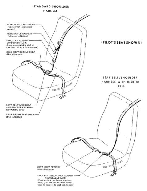
Figure 7-4. Seat Belts and Shoulder Harnesses
