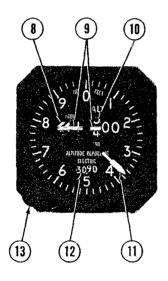
Figure 1. Cessna 400 Transponder and Encoding Altimeter Operating Controls (Sheet 1 of 2)
