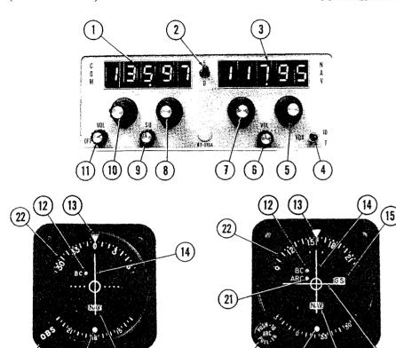
1. COMMUNICATION OPERATING FREQUENCY READOUT (Third-decimal-place is shown by the position of the "5-0" switch).
