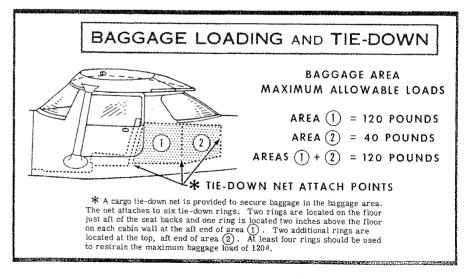
Figure 6-4. Baggage Loading and Tie-Down
