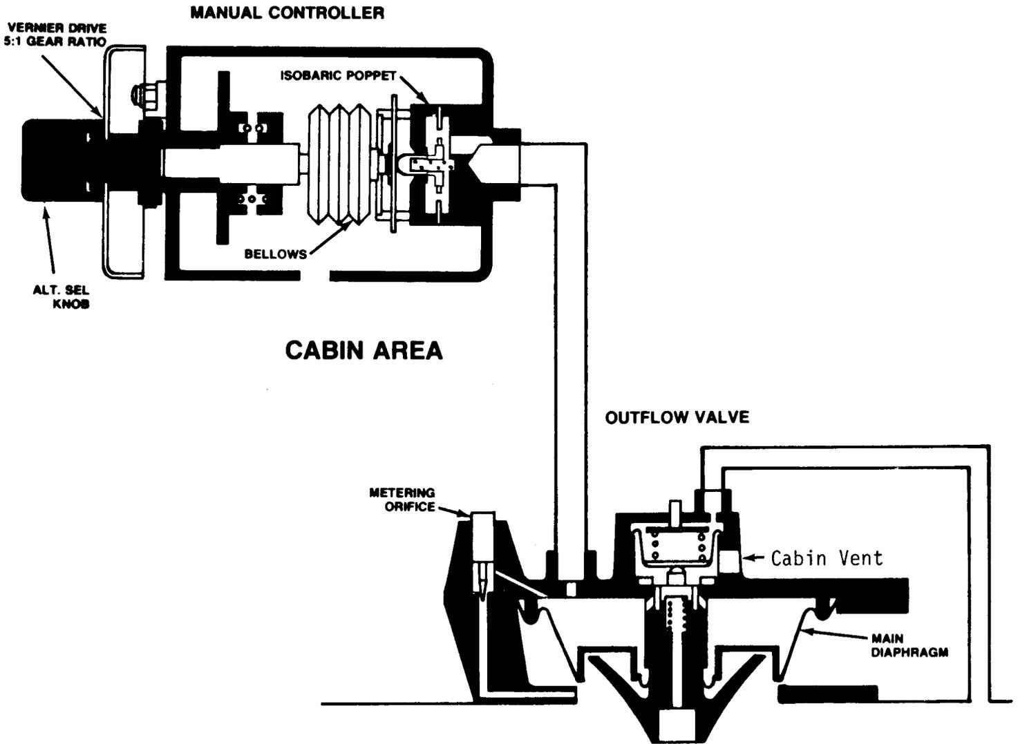
OUTFLOW VALVE AND CONTROLLER SYSTEM
