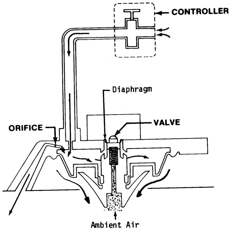
OUTFLOW VALVE - INCLUDING DIFFERENTIAL VALVE
