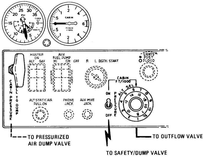
PRESSURIZATION SYSTEM CONTROLS AND INSTRUMENTS
