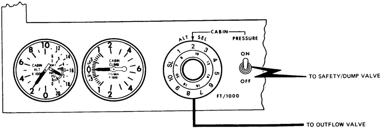
PRESSURIZATION SYSTEM CONTROLS AND INSTRUMENTS
