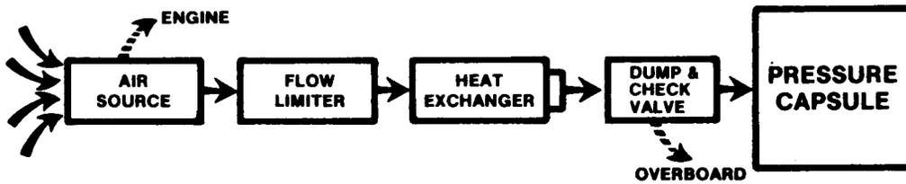
inside the core of the heat exchanger, and cool compressed air is allowed to enter the cabin. An air scoop in the lower forward left side of the nose structure, and an exhaust scoop located in the lower side cowl panel assures a high volume of ambient airflow through the heat exchanger.
