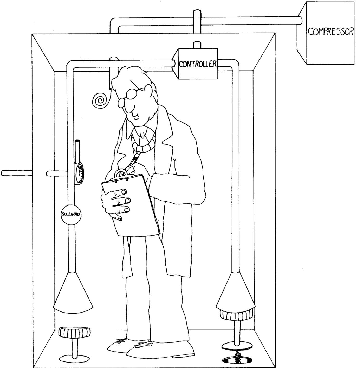
We can monitor the pressure inside our capsule by the use of a DIFFERENTIAL PRESSURE GAUGE. It would be referenced to the INSIDE pressure as well as the OUTSIDE pressure, so it would indicate the difference between the two references and thus show cabin differential pressure.
