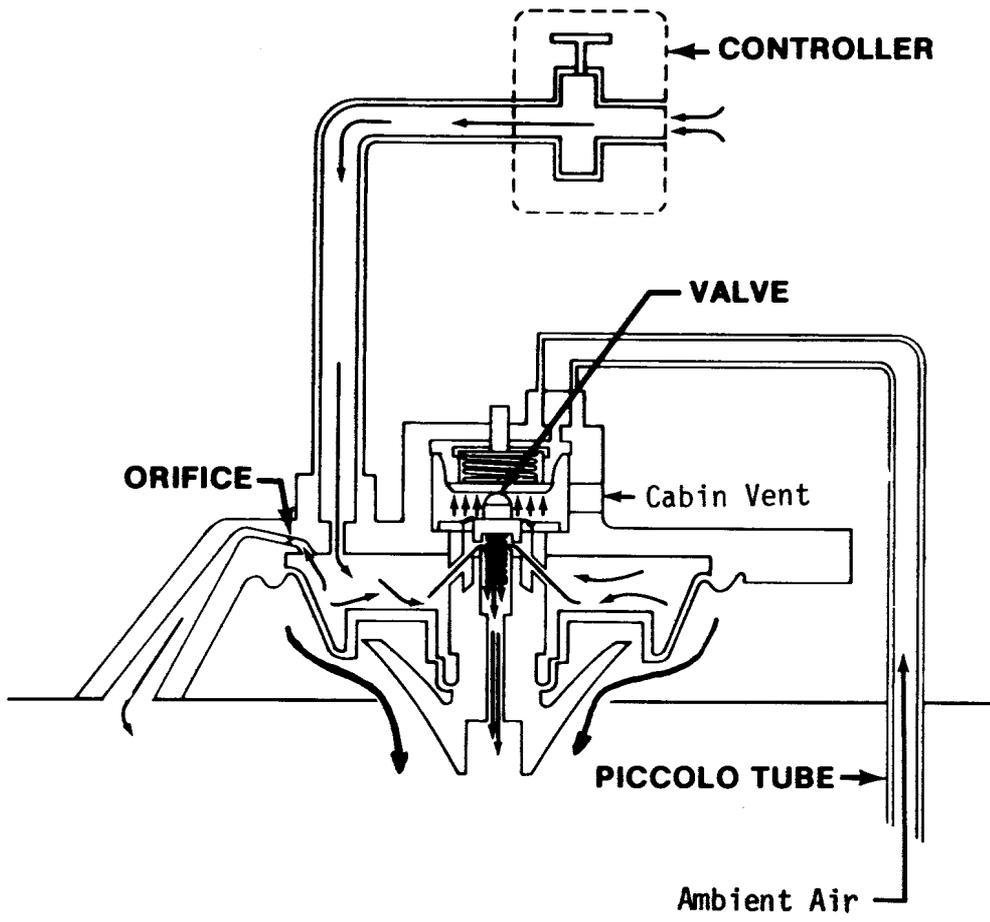
OUTFLOW VALVE WITH COMPLETE DIFFERENTIAL PRESSURE REGULATOR
