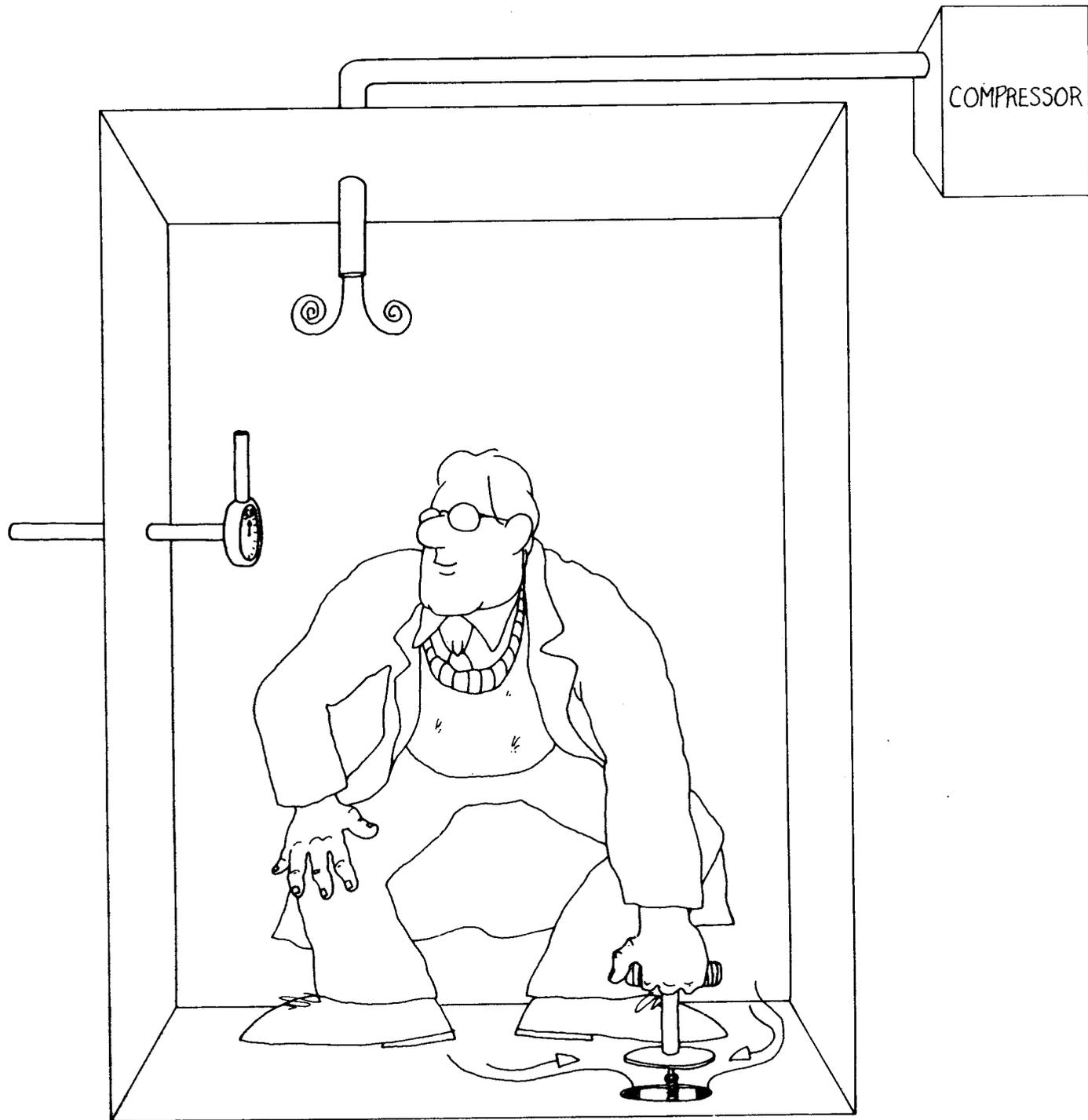
One solution would be to provide the person inside the capsule with supplemental oxygen. However, this is only a short term remedy. When the oxygen supply is exhausted, the crew member once again suffers from hypoxia.
