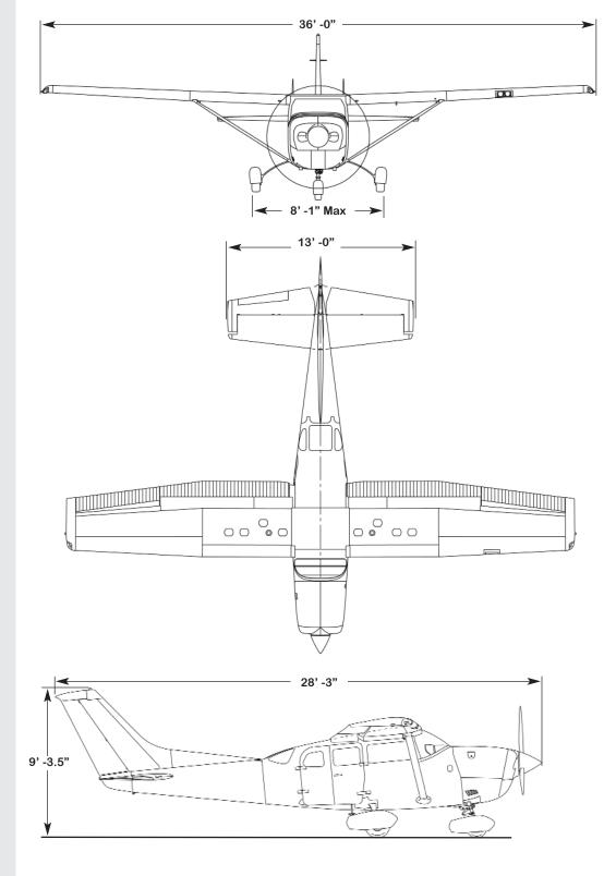
FIGURE I — STATIONAIR EXTERIOR DIMENSIONS
