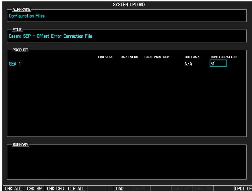
**Figure 2-29. CONFIGURATION UPLOAD Page (GDU software version 7.01 or later)**
