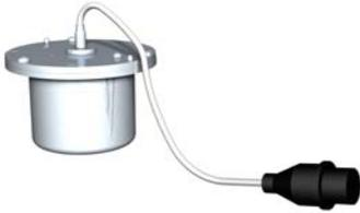
**GMU 44:** The GMU 44 magnetometer senses magnetic field information. Data is sent to the GRS 77 ARHS for processing to determine aircraft magnetic heading. This unit receives power directly from the GRS 77 and communicates with the GRS 77 using RS-485 digital interface.
