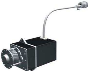
**GSA 81 & GSM 85:** The GSA 81 servo actuator is an electromechanical LRU that provides automatic control of pitch, roll, and pitch trim. It also provides manual electric trim functionality. The GSA 81 contains a motor-control and monitor circuit board, as well as a solenoid and a brushless DC motor. The GSA 81 receives serial RS-485 data packets from the GIA 63Ws.
