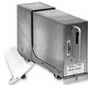
**GDL 90** The GDL 90 is a remote-mounted product that contains a GPS/WAAS receiver and a Universal Access Transceiver. The GDL 90 will transmit “ownership” data via the UAT data link. It will receive data from other UAT-equipped aircraft as well as FIS-B weather – the received data may be output to an appropriate display.
