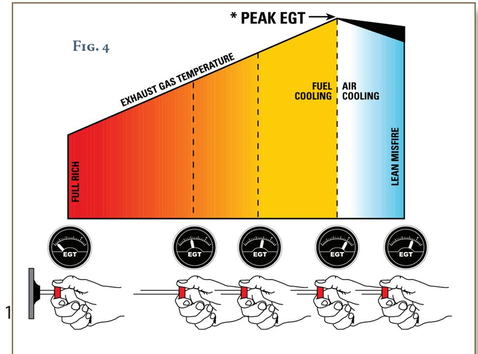
**REMEMBER:** When using the EGT method of mixture control, all mixture settings are made relative to peak EGT.
