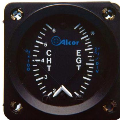
Simply remember to select the leanest cylinder, normally the one with the highest EGT for all mixture control settings, and then "scan" the other cylinders when convenient or when there is any concern for their health, such as a "feel" of roughness. Rely on Alcor's EGT/CHT to monitor your engine and minimize fuel and maintenance costs.
