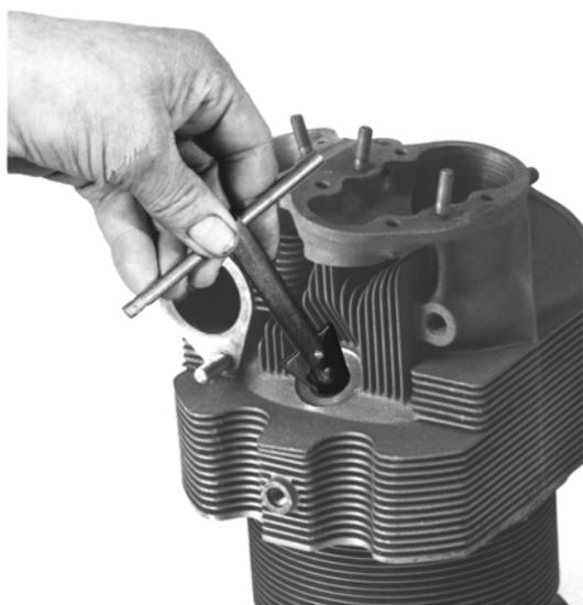
**FIGURE 16-8. REMOVING SPARK PLUG HOLE HELICAL INSERT**
