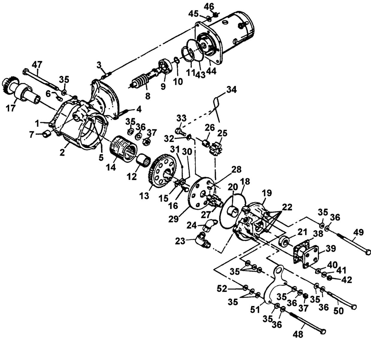
FIGURE 6-8. OPTIONAL STARTER ADAPTER ASSEMBLY (TSIO-360-RB)
