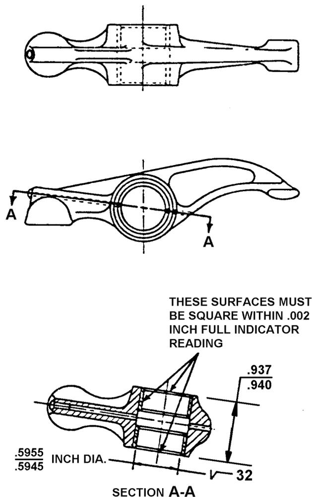
**FIGURE 16-11. ROCKER ARM BUSHING REPLACEMENT**
