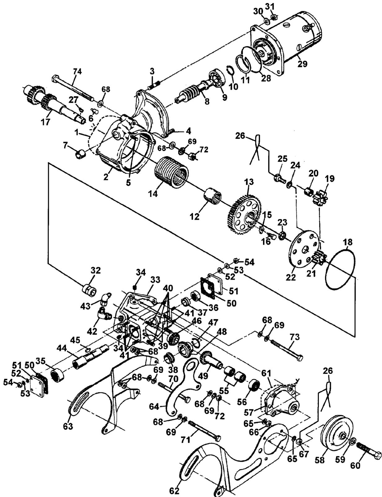
FIGURE 6-5. COMPRESSOR MOUNTING COMPONENTS, STARTER AND STARTER ADAPTER ASSEMBLY (TSIO-360-RB)
