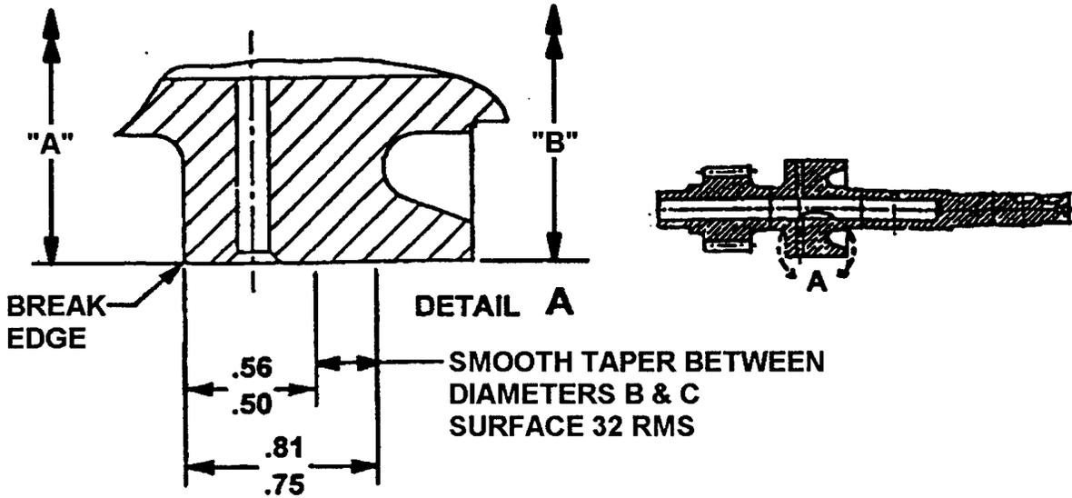
FIGURE 11-2B. SHAFTGEAR DRUM DIMENSIONS
