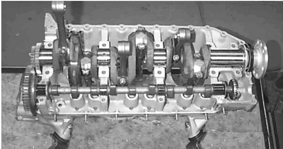
**FIGURE 19-1. CRANKCASE AND SHAFTS ASSEMBLED ON STAND**
