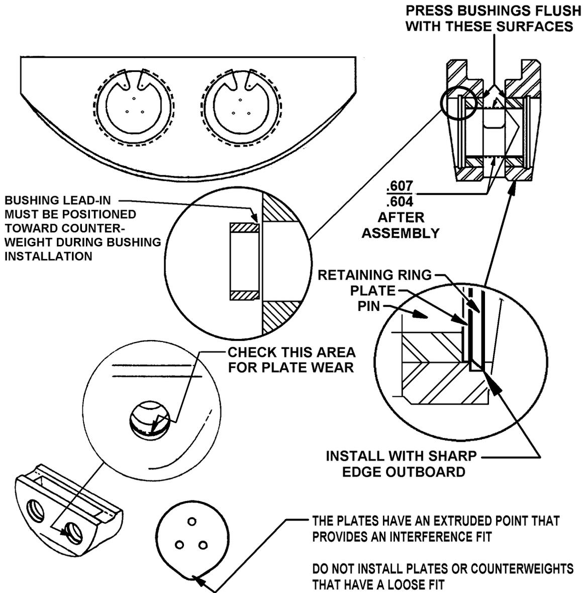
**FIGURE 18-4. COUNTERWEIGHT INSPECTION, REPAIR AND INSTALLATION**
