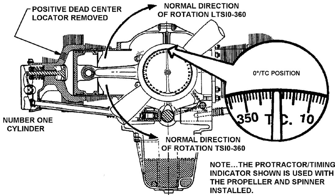
**FIGURE 19-23. TIMING POSITION STEP FOUR**
