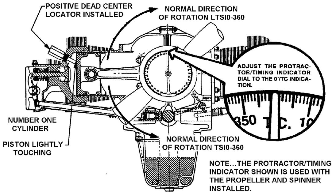
FIGURE 19-20. TIMING POSITION STEP ONE
