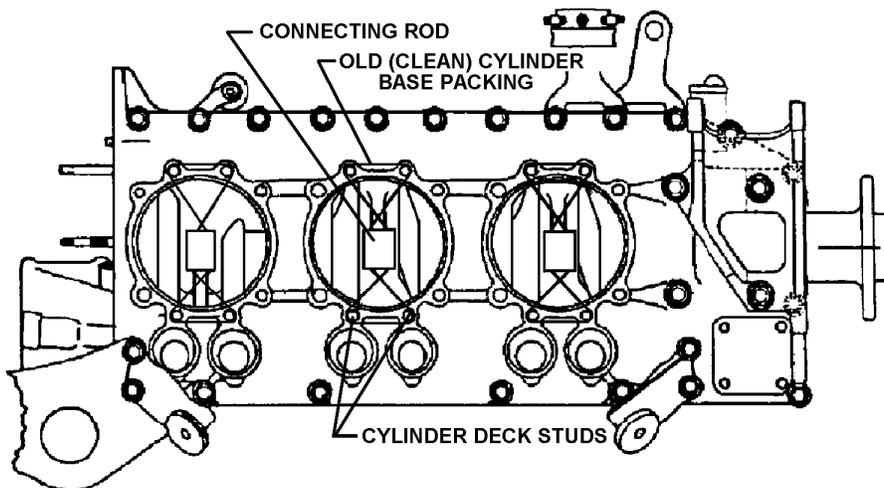
FIGURE 6-15A. CONNECTING ROD SUPPORT
