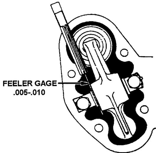
**FIGURE 19-17. CHECKING ROCKER ARM SIDE CLEARANCE**
