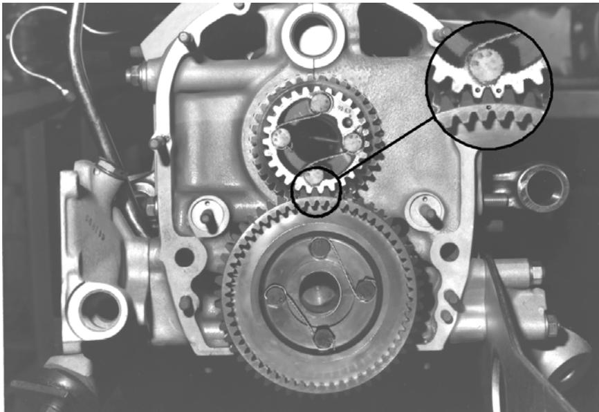
**FIGURE 19-2. ALIGNMENT OF TIMING MARKS**
