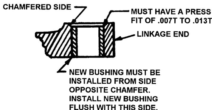
FIGURE 9-6. GENERAL LEVER BUSHING REPLACEMENT
