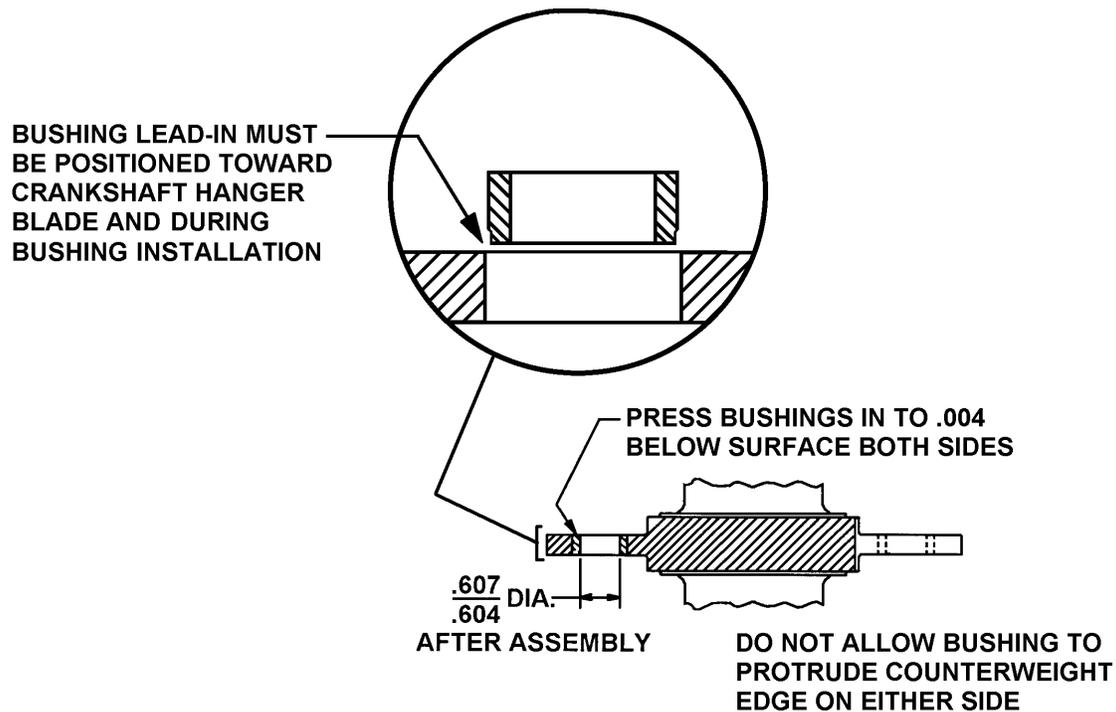
**FIGURE 18-3. CRANKSHAFT HANGER BLADE BUSHING REPLACEMENT**
