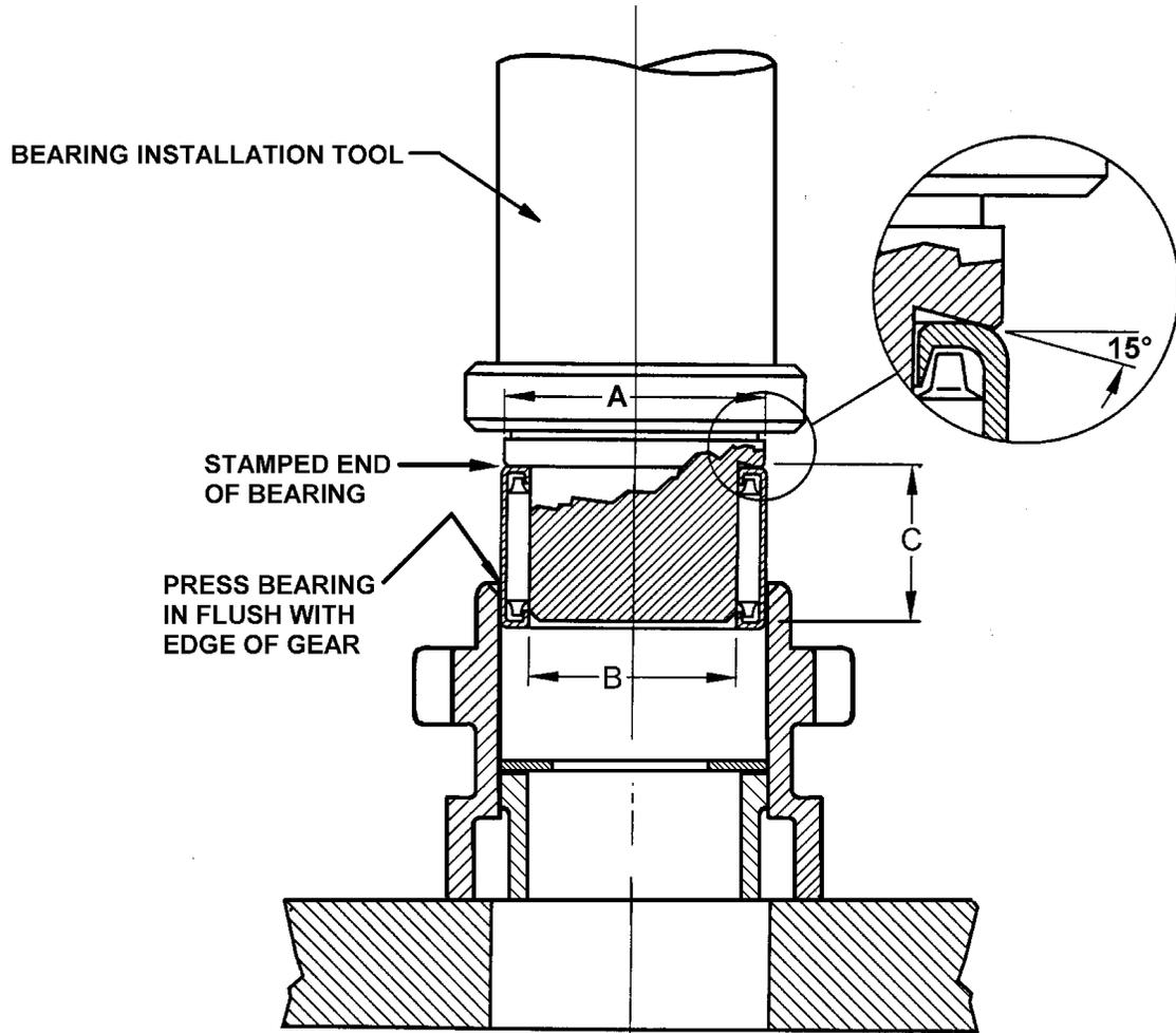
**FIGURE 8-3. NEEDLE BEARING INSTALLATION**
