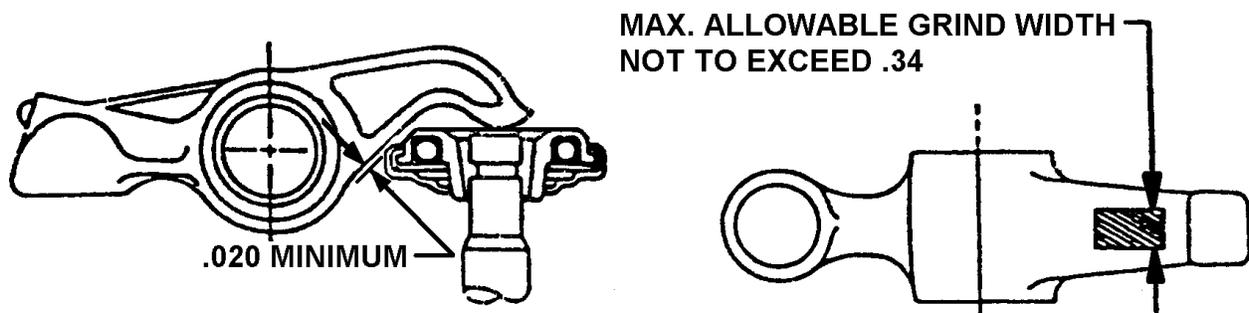
**FIGURE 16-12. ROCKER ARM TO ROTOCOIL CLEARANCE**
