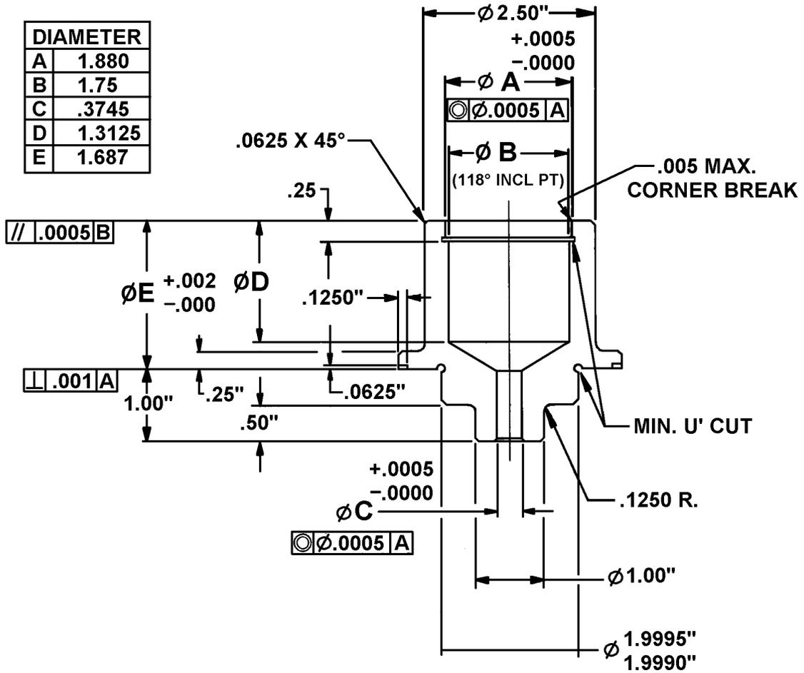
FIGURE 16-14. VALVE GAUGE LINE INSPECTION FIXTURE
