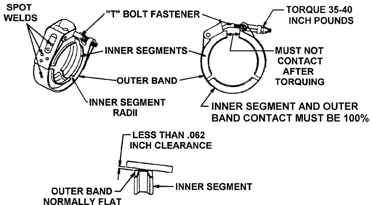
FIGURE 19-19. MULTI-SEGMENT "V" BAND CLAMP
