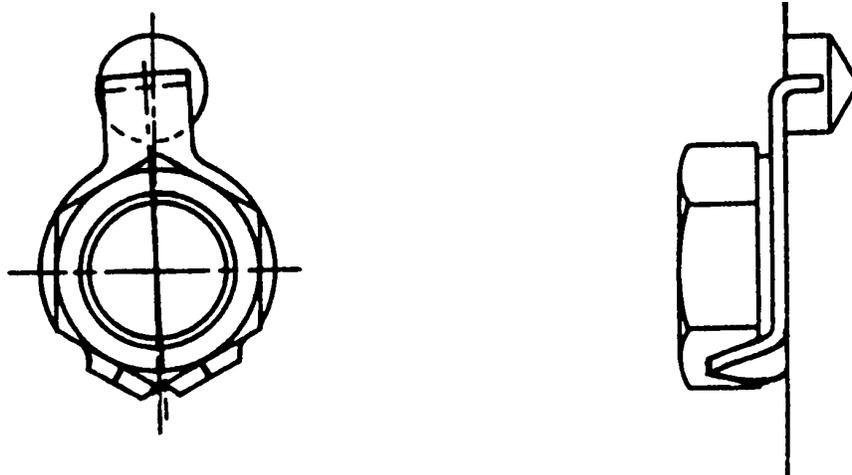
**FIGURE 4-3 GENERAL TAB WASHER INSTALLATION PROCEDURE**
