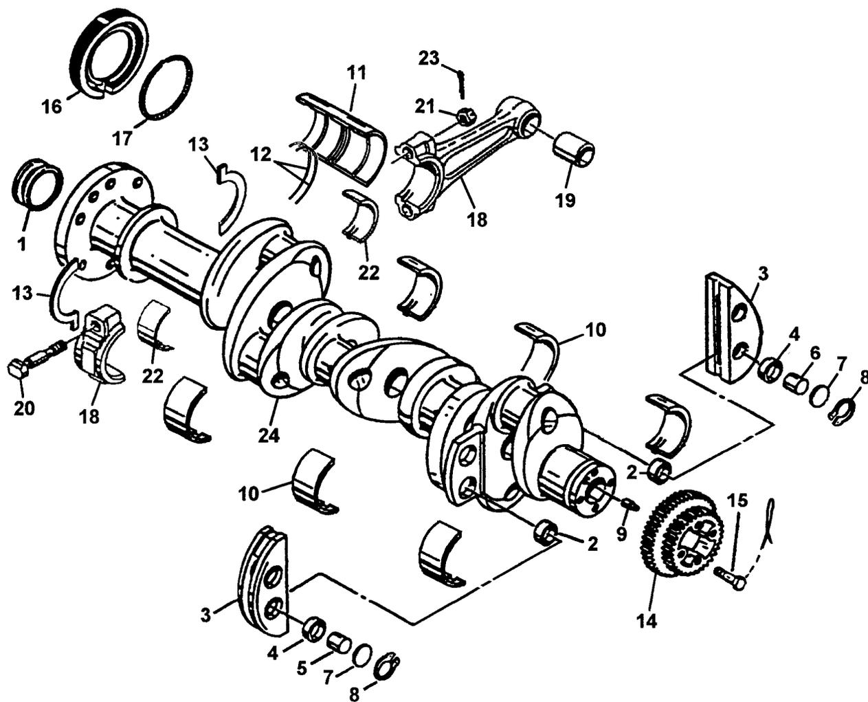
**FIGURE 6-19. CRANKSHAFT ASSEMBLY**
