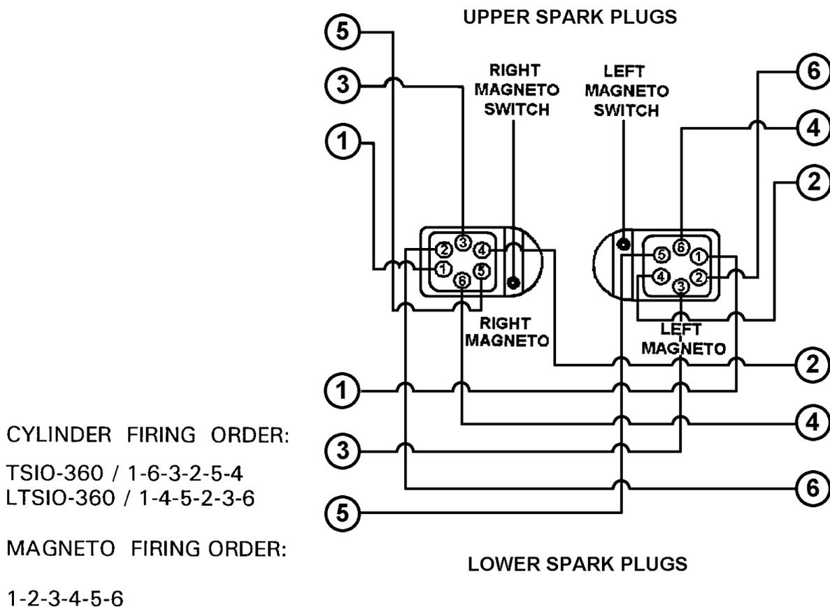
**FIGURE 19-26. IGNITION WIRING DIAGRAM**
