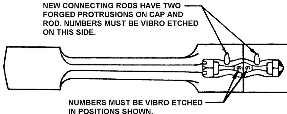
**FIGURE 18-9. CONNECTING ROD POSITION NUMBER**
