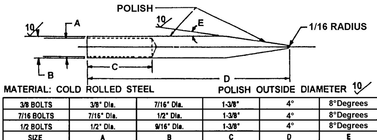
**FIGURE 19-4. O-RING INSTALLATION TOOL**
