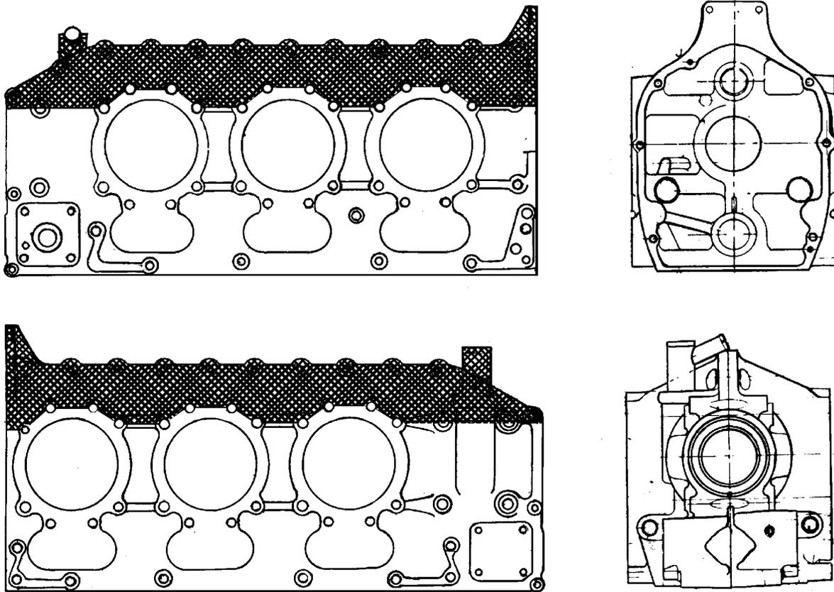
**FIGURE 17-2. INSPECTION OF CRANKCASE CRITICAL (WHITE) AND NON CRITICAL (SHADED) AREAS**
