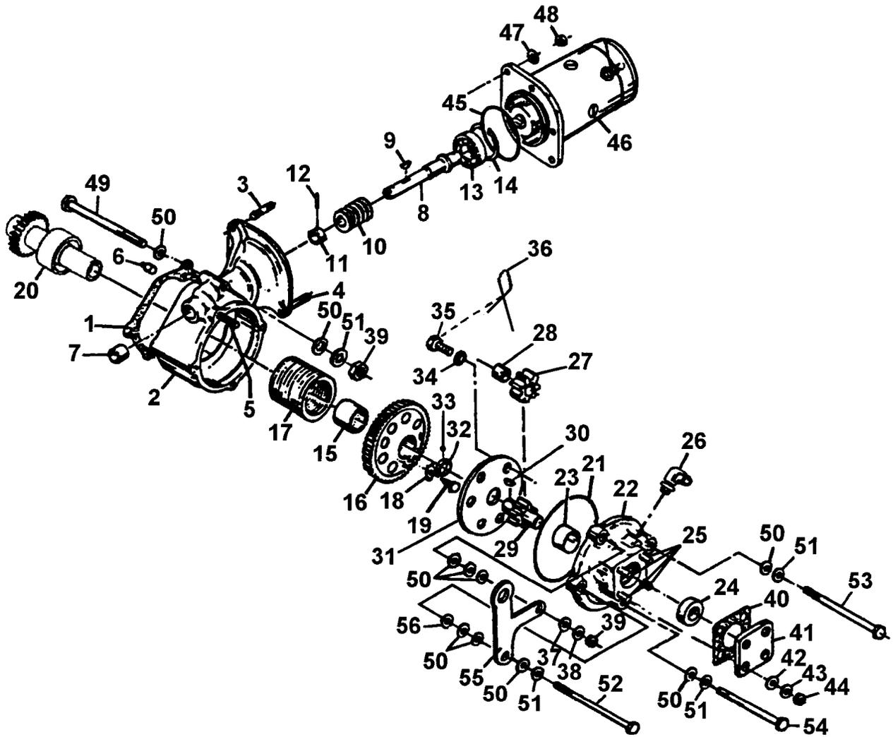
FIGURE 6-9. STARTER ADAPTER ASSEMBLY (LTSI0-360-RB)
