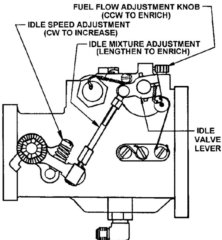
FIGURE 20-3. FUEL SERVO ADJUSTMENTS
