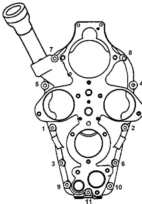
**FIGURE 19-12. ACCESSORY CASE TORQUING SEQUENCE**
