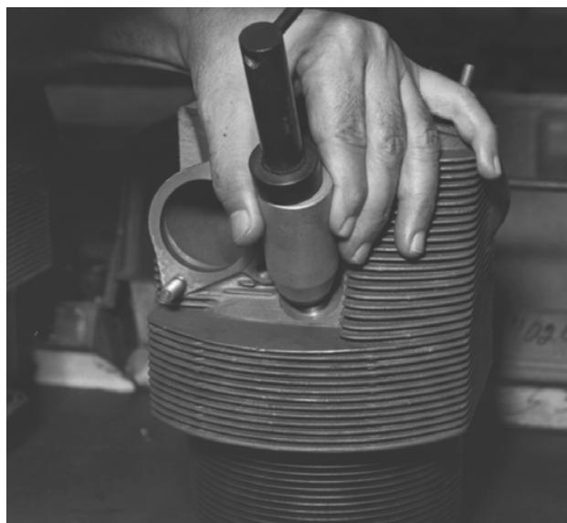
**FIGURE 16-9. INSTALLING SPARK PLUG HELICAL COIL**
