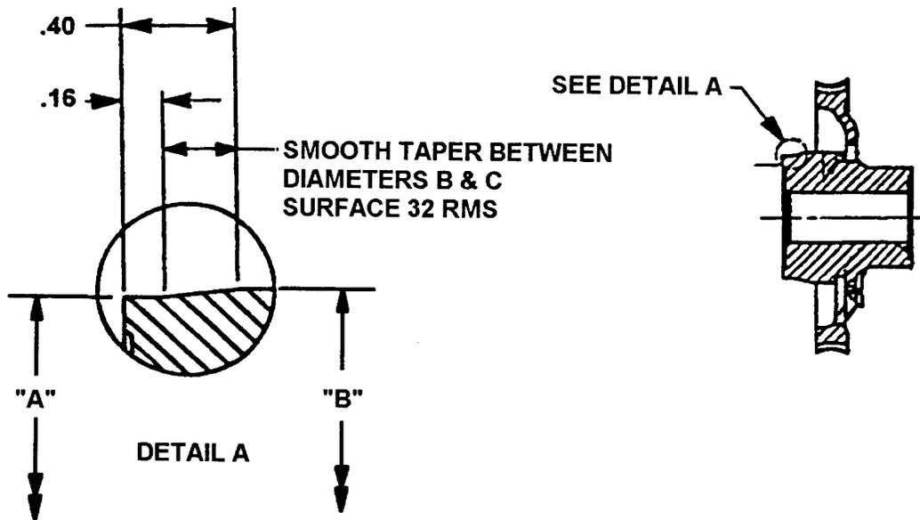
FIGURE 11-2C. WORM WHEEL DRUM DIMENSIONS
