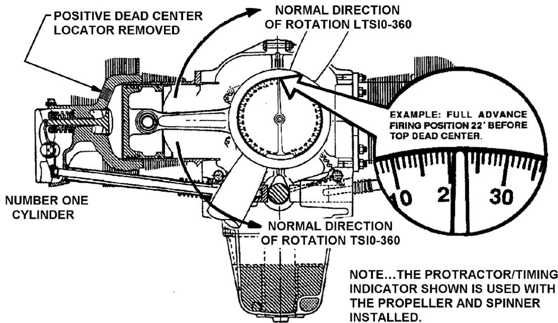
**FIGURE 19-24. TIMING POSITION STEP FIVE**
