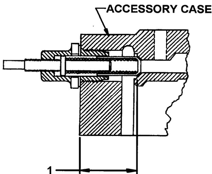
**FIGURE 14-2. OIL PRESSURE RELIEF VALVE FITS AND LIMITS**
