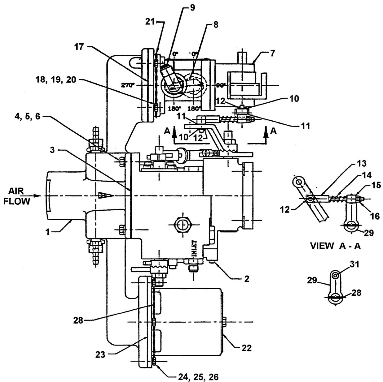
FIGURE 9-3. AIR THROTTLE ADAPTER, FUEL SERVO, CONTROLLER AND OVERBOOST VALVE
