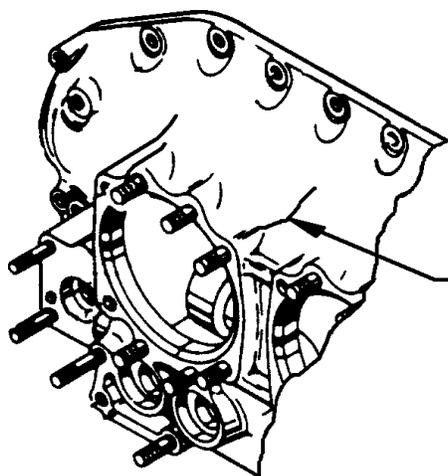
**Cracks less than two inches in length and located in shaded areas as illustrated in Figure 17-2.**
