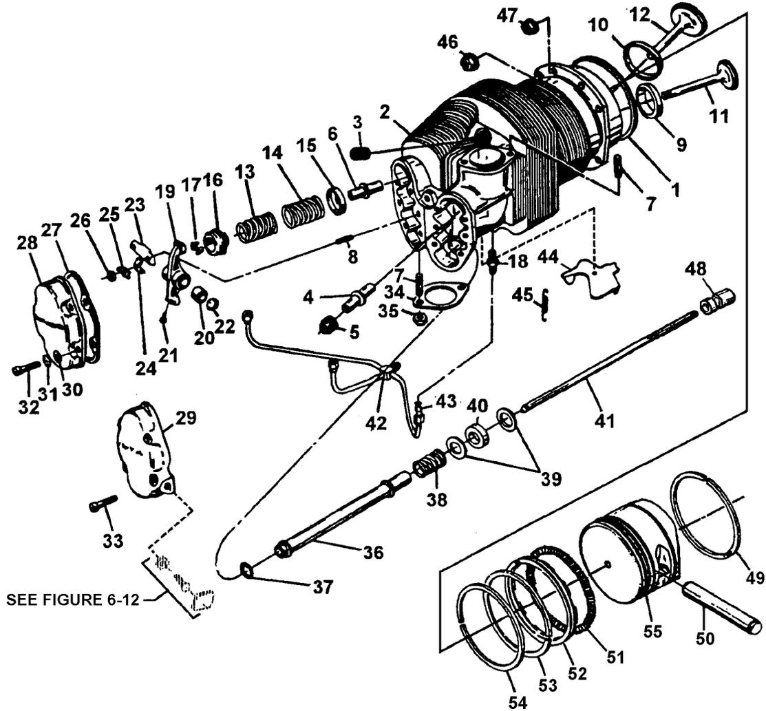
FIGURE 6-15. CYLINDER AND PISTON ASSEMBLY
