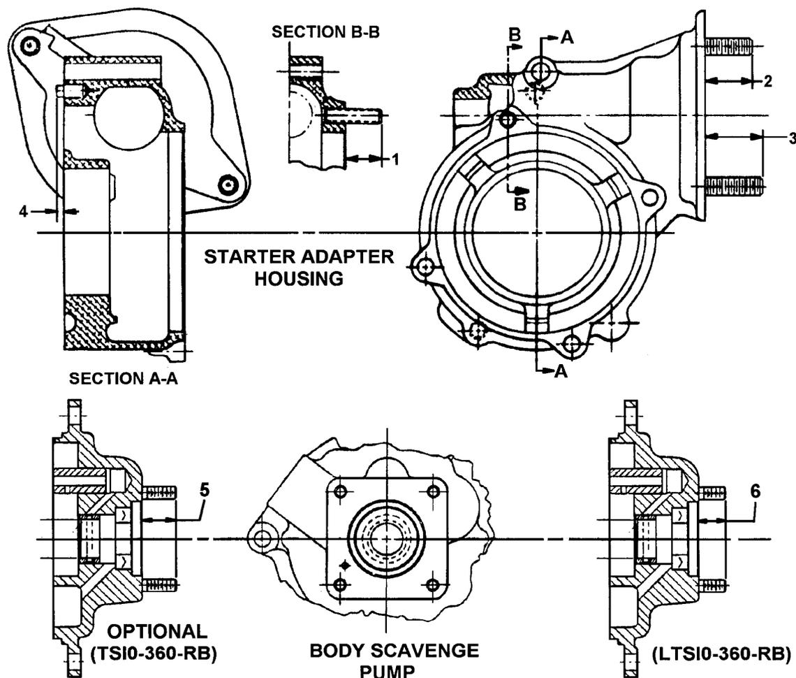
FIGURE 13-2. STARTER ADAPTER STUD SETTING HEIGHTS
