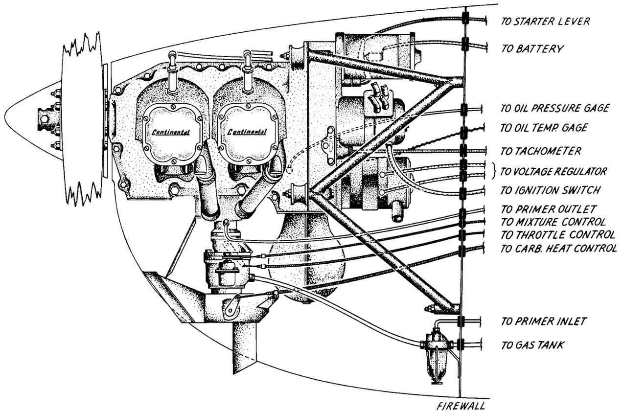
Figure 12. Typical Installation Diagram for -12, -14 & -16 Models, Side View.
