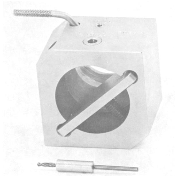
Figure 23. Drill Fixture
