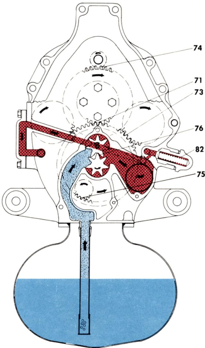
REAR VIEW (-12 ENGINE) SHOWING OIL PRESSURE RELIEF VALVE AND OIL COOLER MOUNTING PAD
