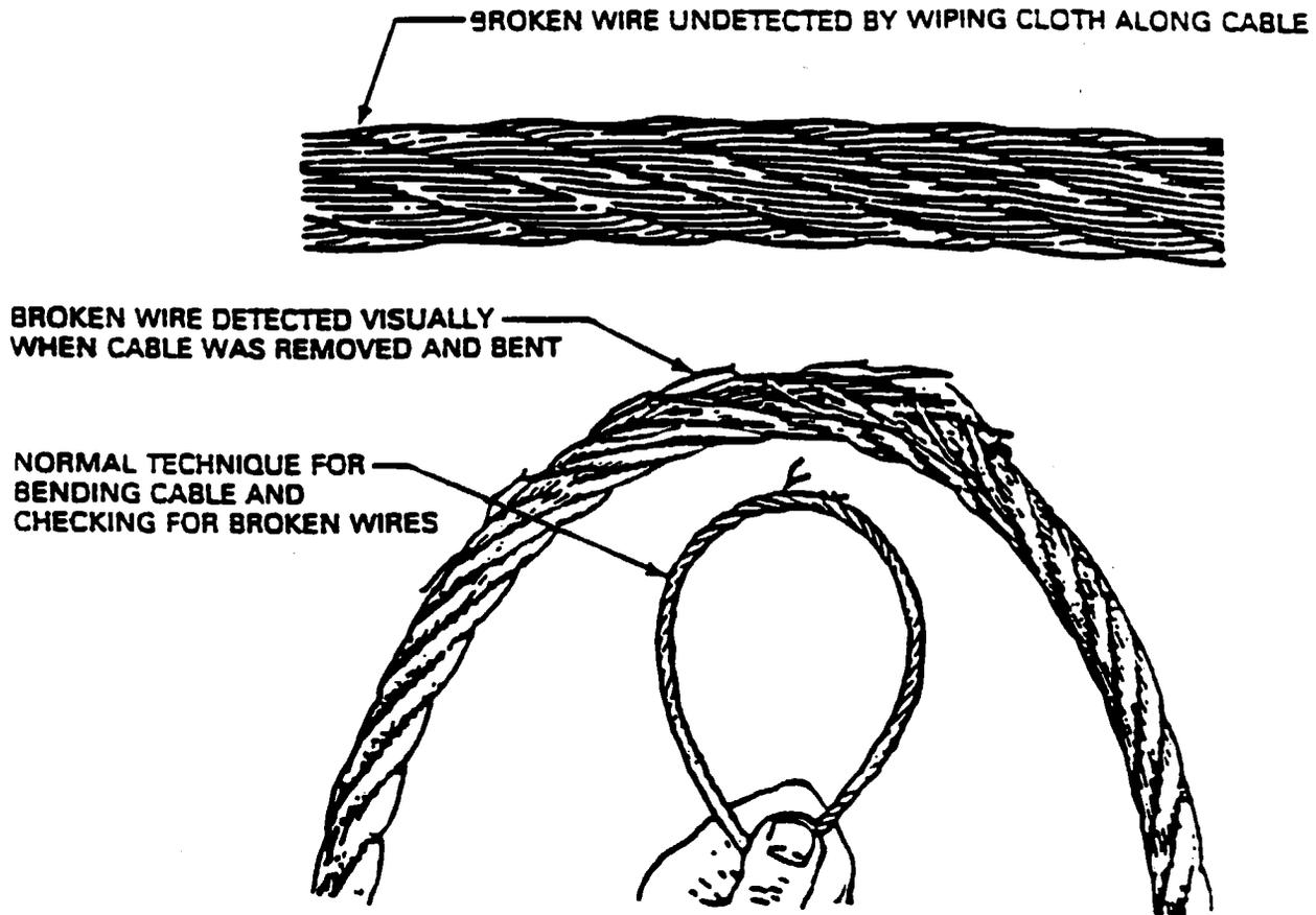
**DO NOT BEND INTO LOOP SMALLER THAN 50 CABLE DIAMETERS**
