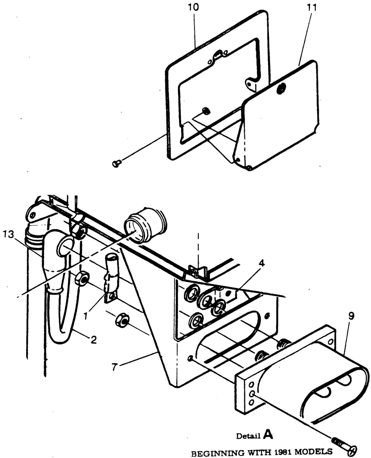
Figure 16-3. Ground Service Receptacle Installation (Sheet 2 of 2)
