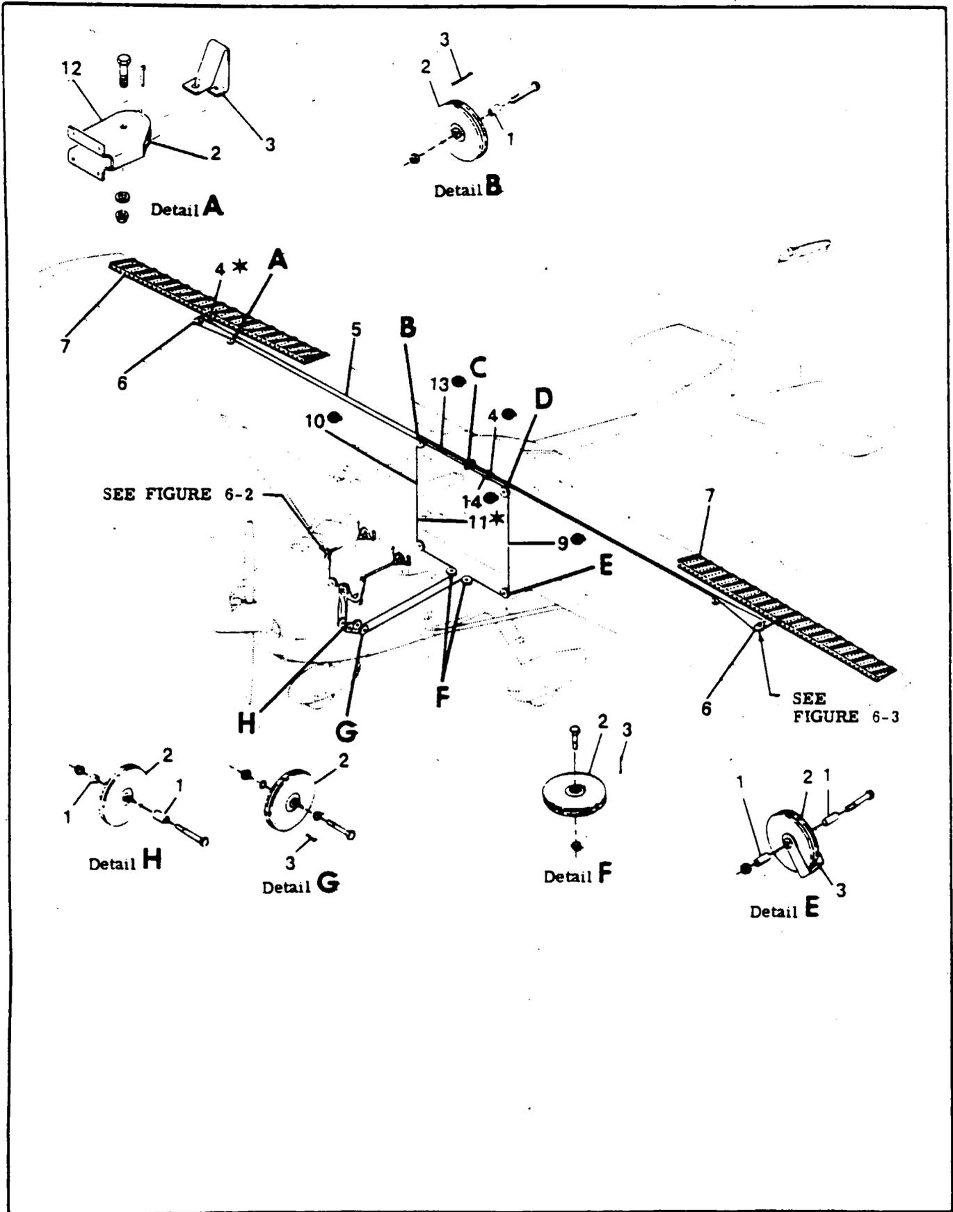
Figure 6-1. Aileron Control System (Sheet 1 of 2)
