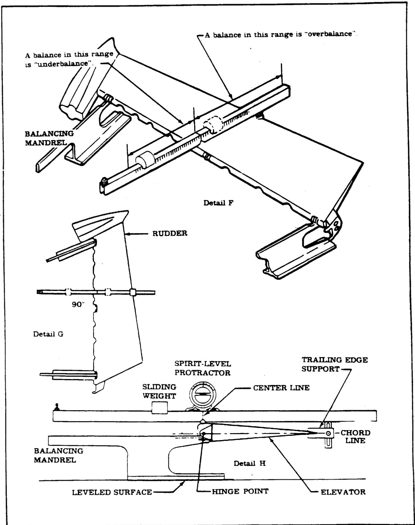
Figure 18-3. Control Surface Balancing (Sheet 3 of 5)
