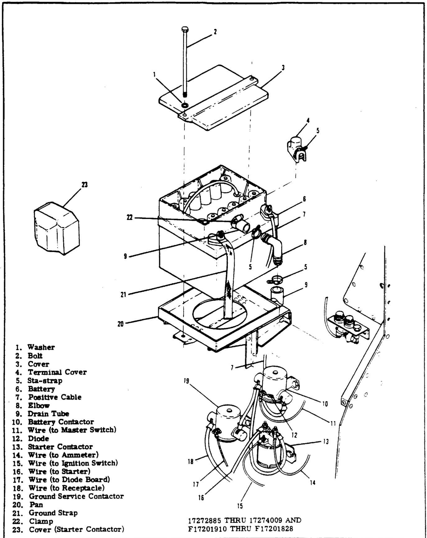
Figure 16-2. Battery and Electrical Equipment Installation (Sheet 4 of 7)
