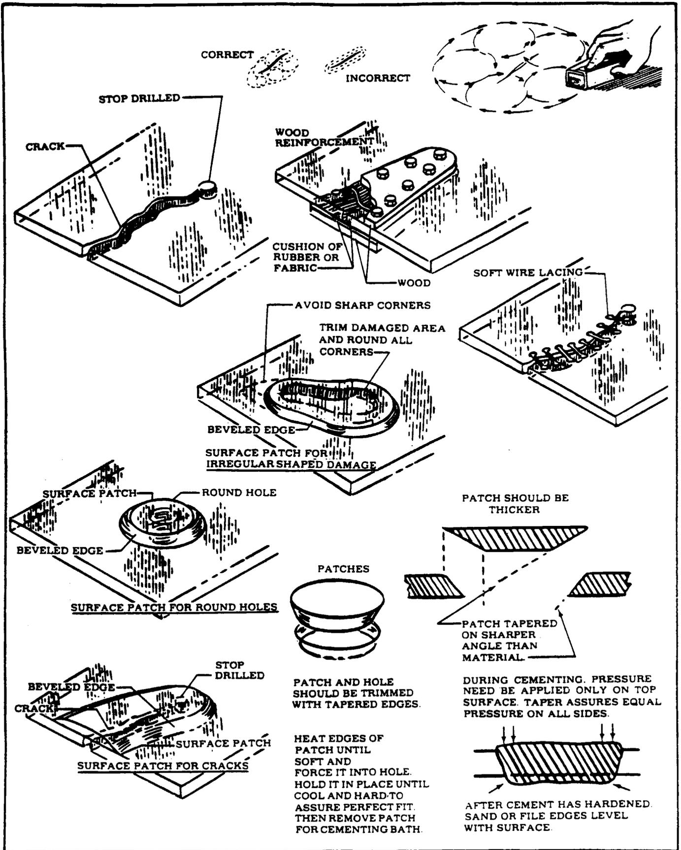
Figure 3-2. Repair of Windshield and Windows
