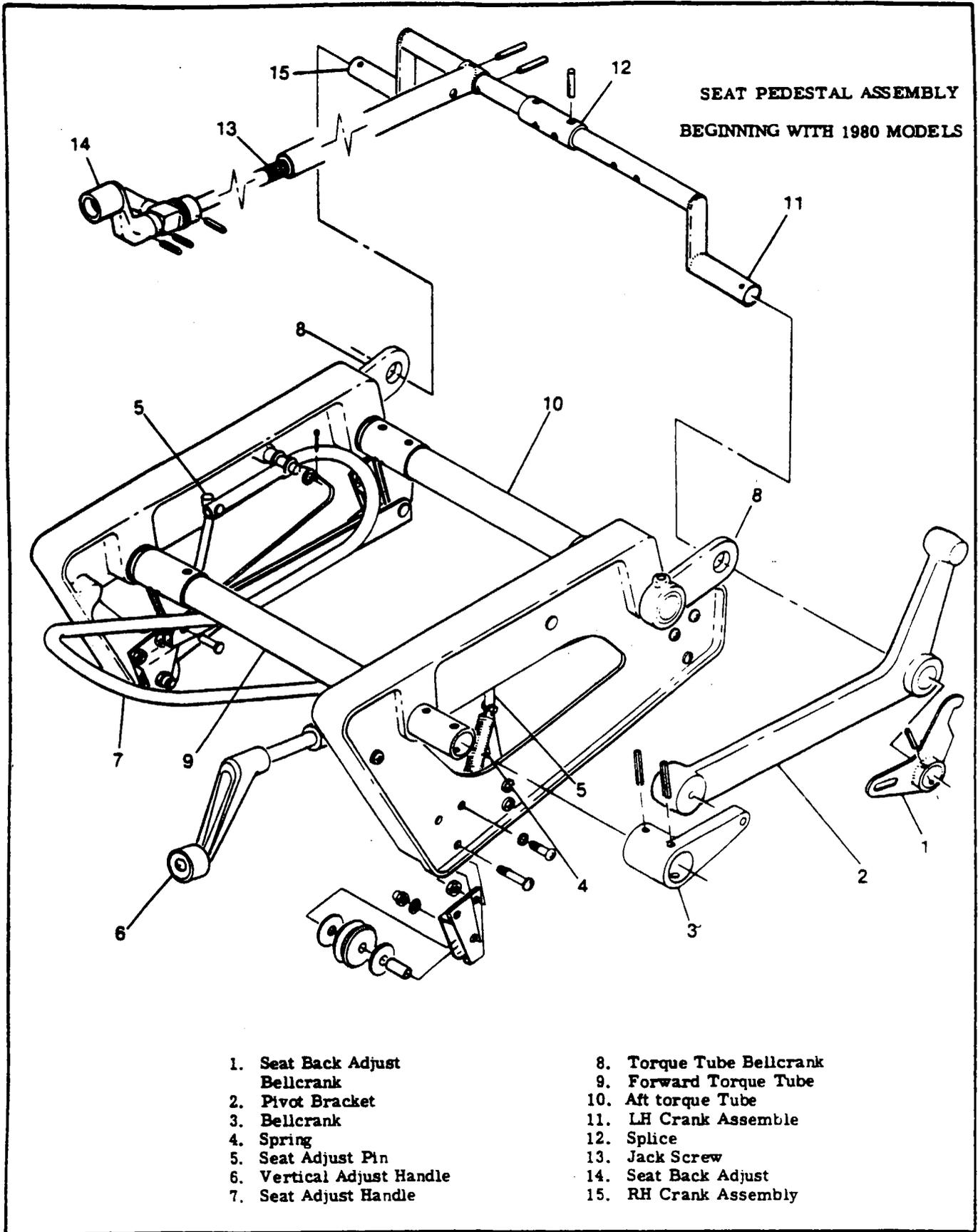
**Figure 3-6. Seat Installation (Sheet 6 of 11)**
