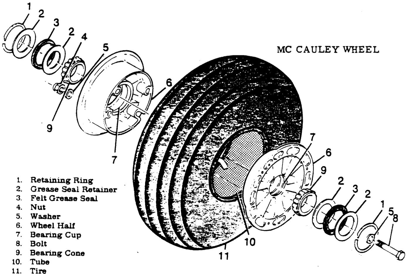
Figure 5-9. Nose Wheel and Tire (Sheet 1 of 2)
