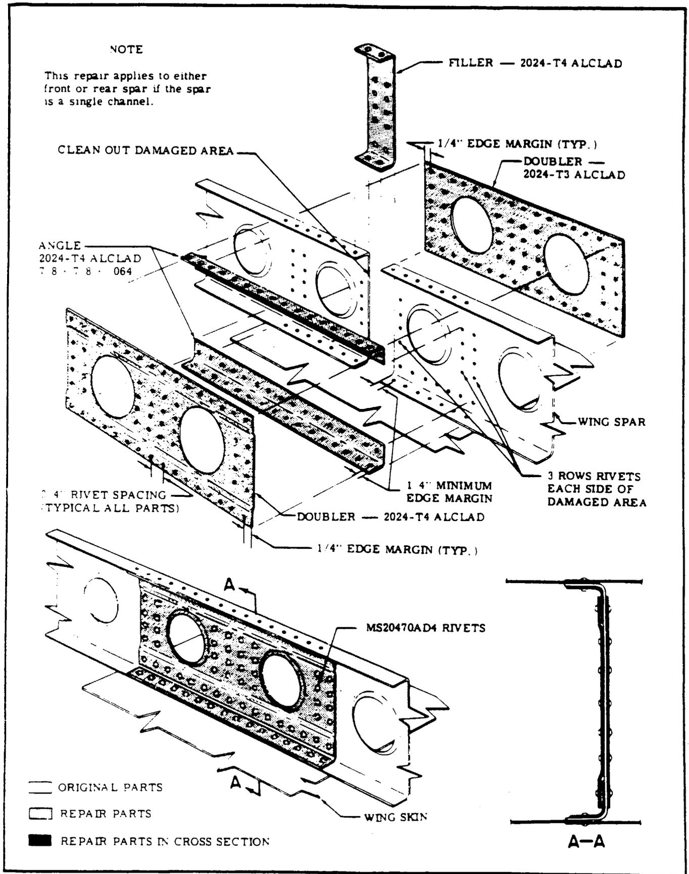
Figure 18-7. Wing Spar Repair (Sheet 2 of 3)
