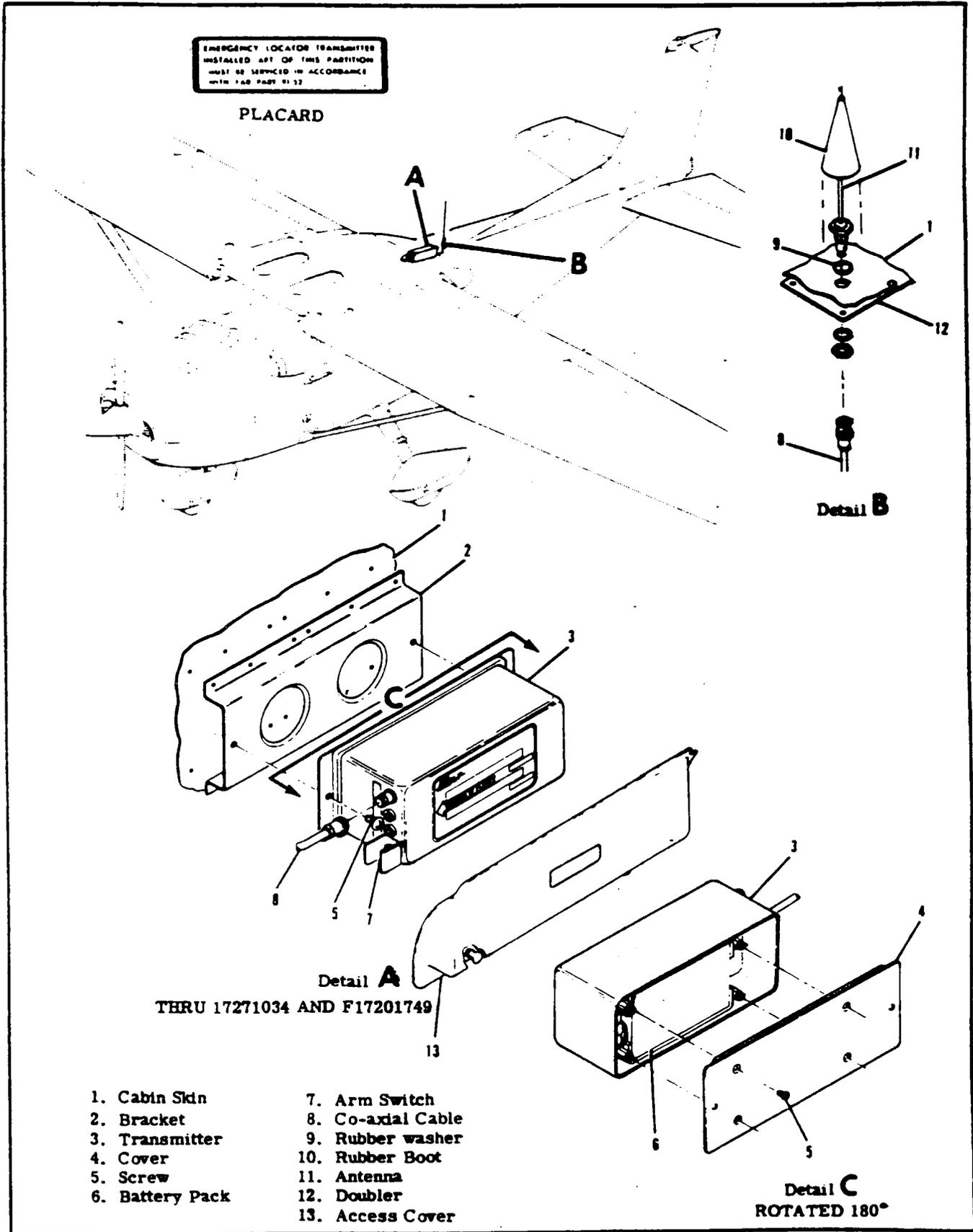
Figure 16-17. Emergency Locator Transmitter Installation (Sheet 1 of 3)
