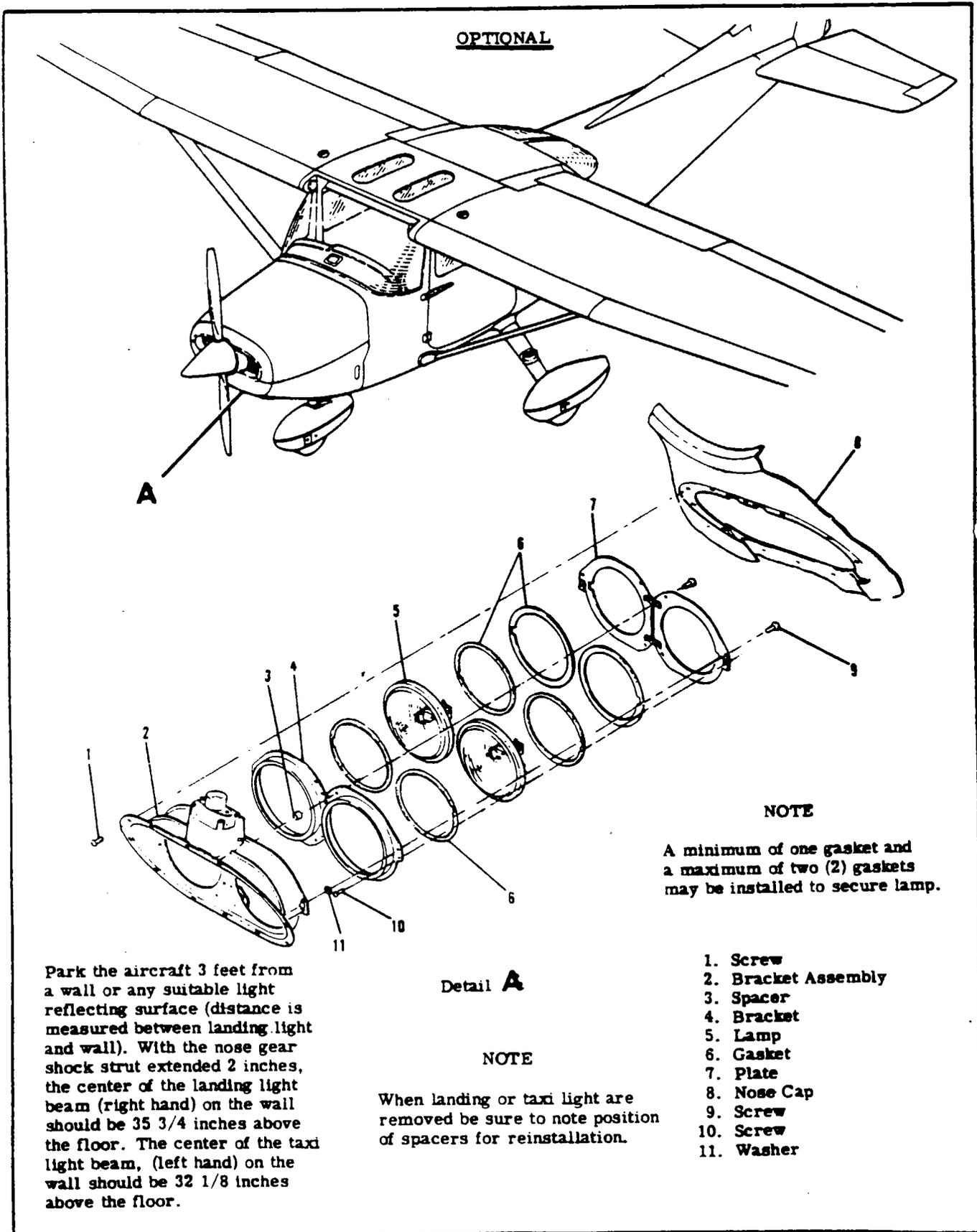
Figure 16-6. Landing and Taxi Light Installation (Sheet 2 of 3)
