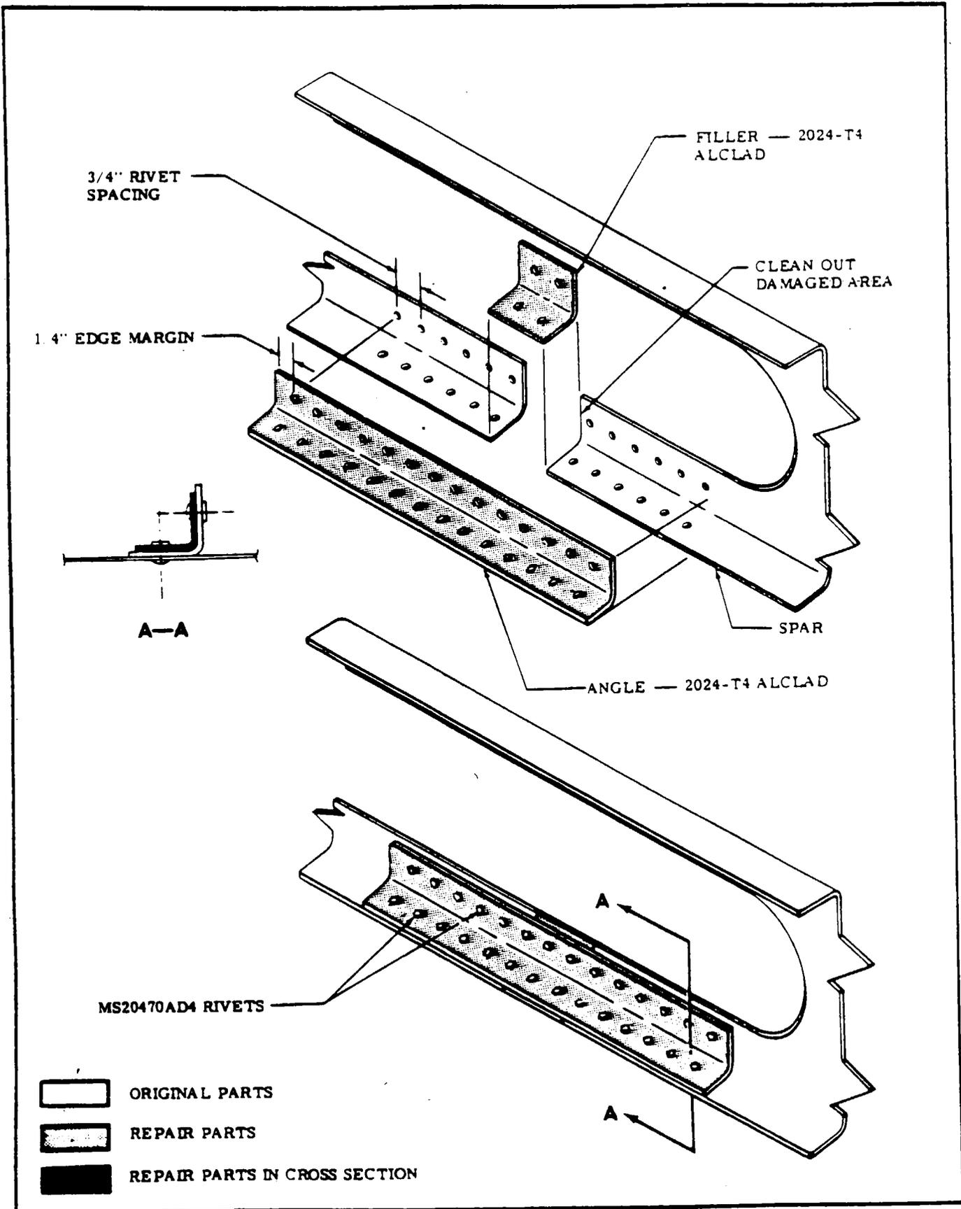
Figure 18-7. Wing Spar Repair (Sheet 3 of 3)
