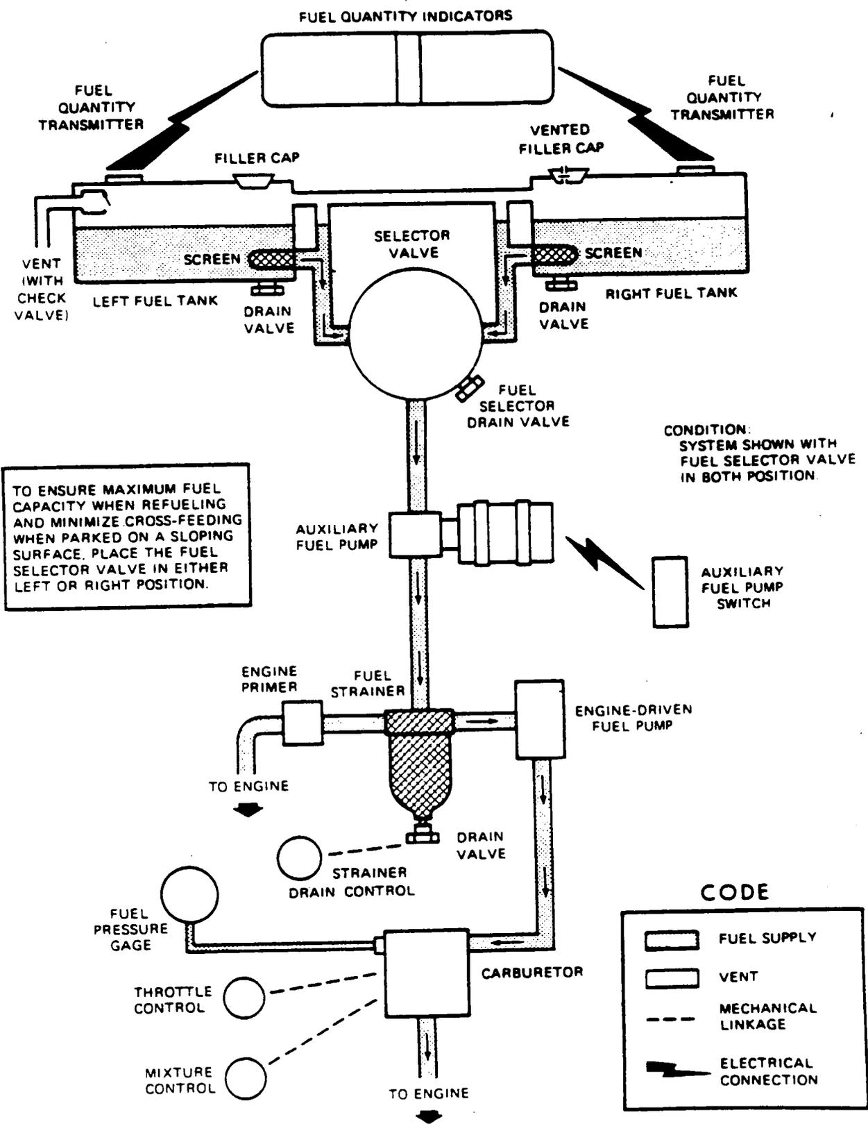
TO ENSURE MAXIMUM FUEL CAPACITY WHEN REFUELING AND MINIMIZE CROSS-FEEDING WHEN PARKED ON A SLOPING SURFACE, PLACE THE FUEL SELECTOR VALVE IN EITHER LEFT OR RIGHT POSITION.
