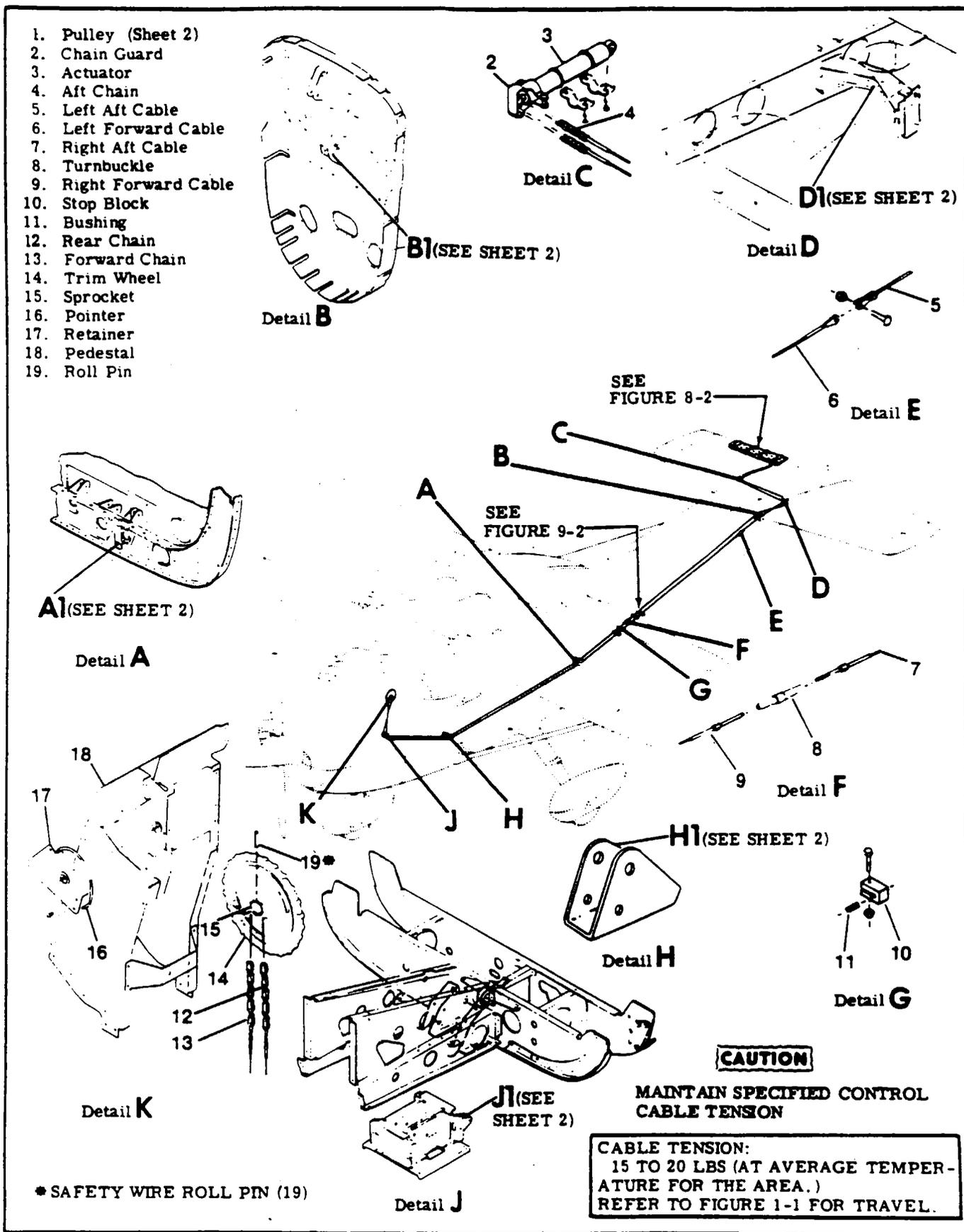
Figure 9-1. Elevator Trim Tab Control System (Sheet 1 of 2)
