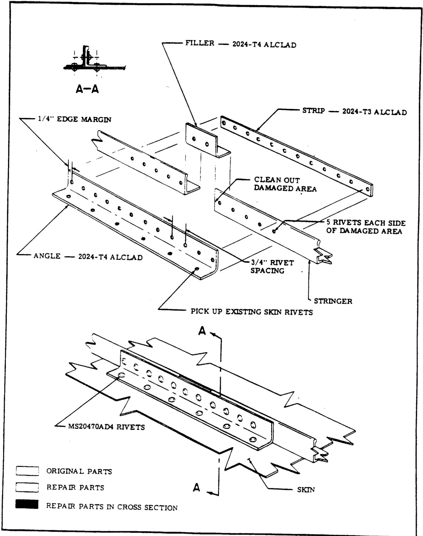
Figure 18-5. Stringer and Channel Repair (Sheet 2 of 4)
