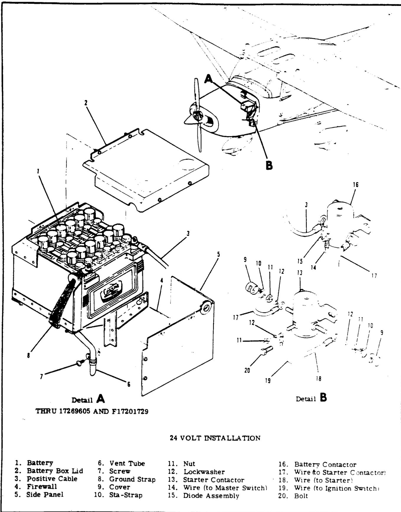
Figure 16-2. Battery and Electrical Equipment Installation (Sheet 2 of 7)
