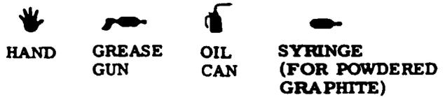
WHERE NO INTERVAL IS SPECIFIED, LUBRICATE AS REQUIRED AND WHEN ASSEMBLED OR INSTALLED.
