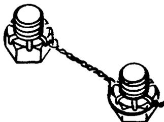
CASTELLATED NUTS ON DRILLED STUDS DOUBLE-TWIST METHOD
