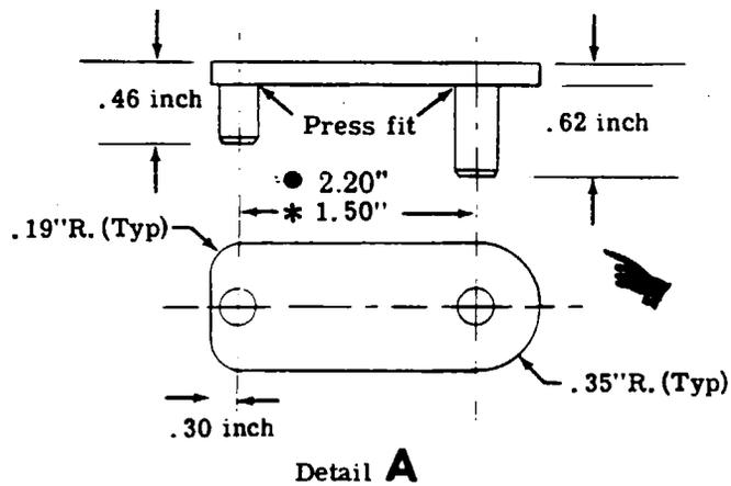
Fabricate from .125 inch steel plate and
