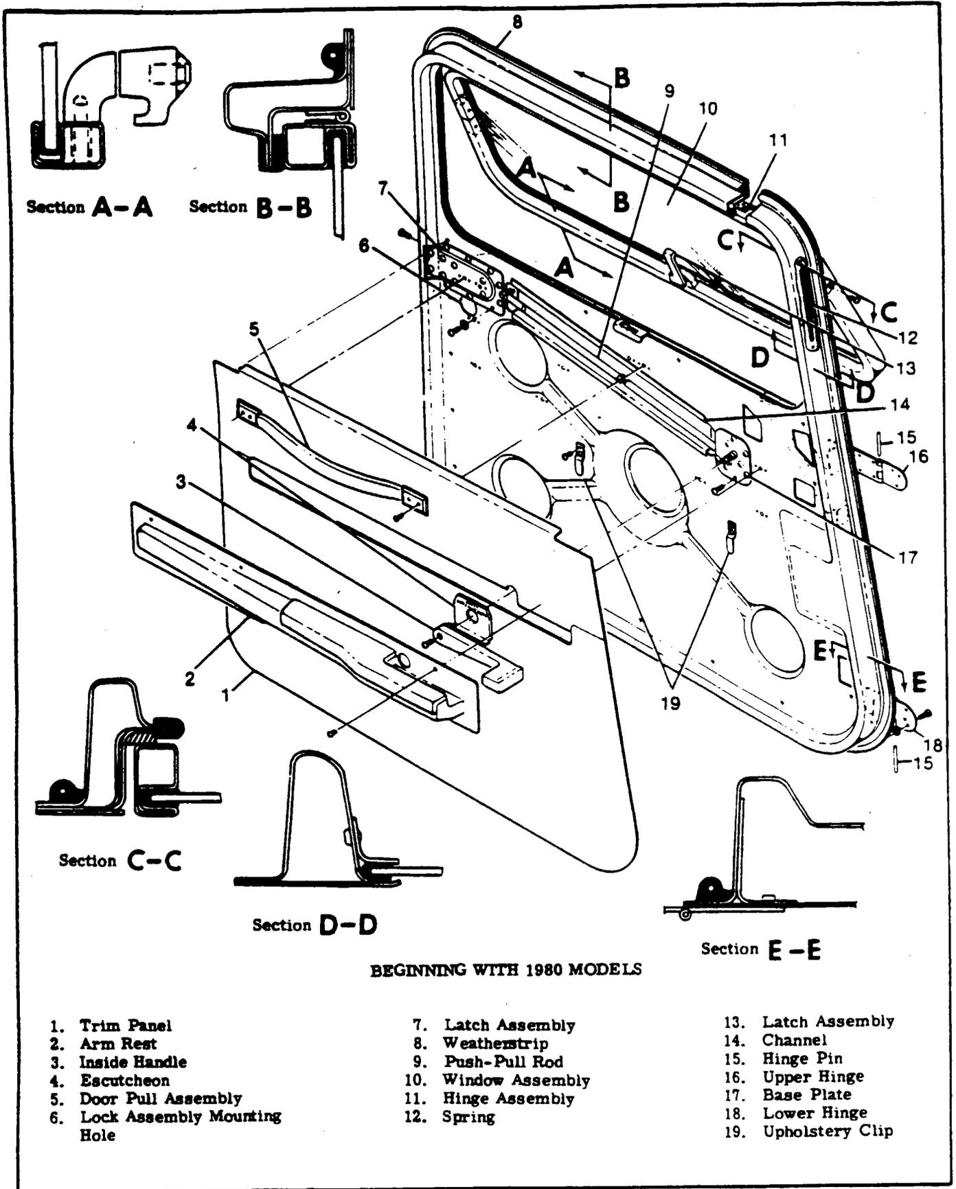
Figure 3-3. Cabin Door Installation (Sheet 2 of 2)
