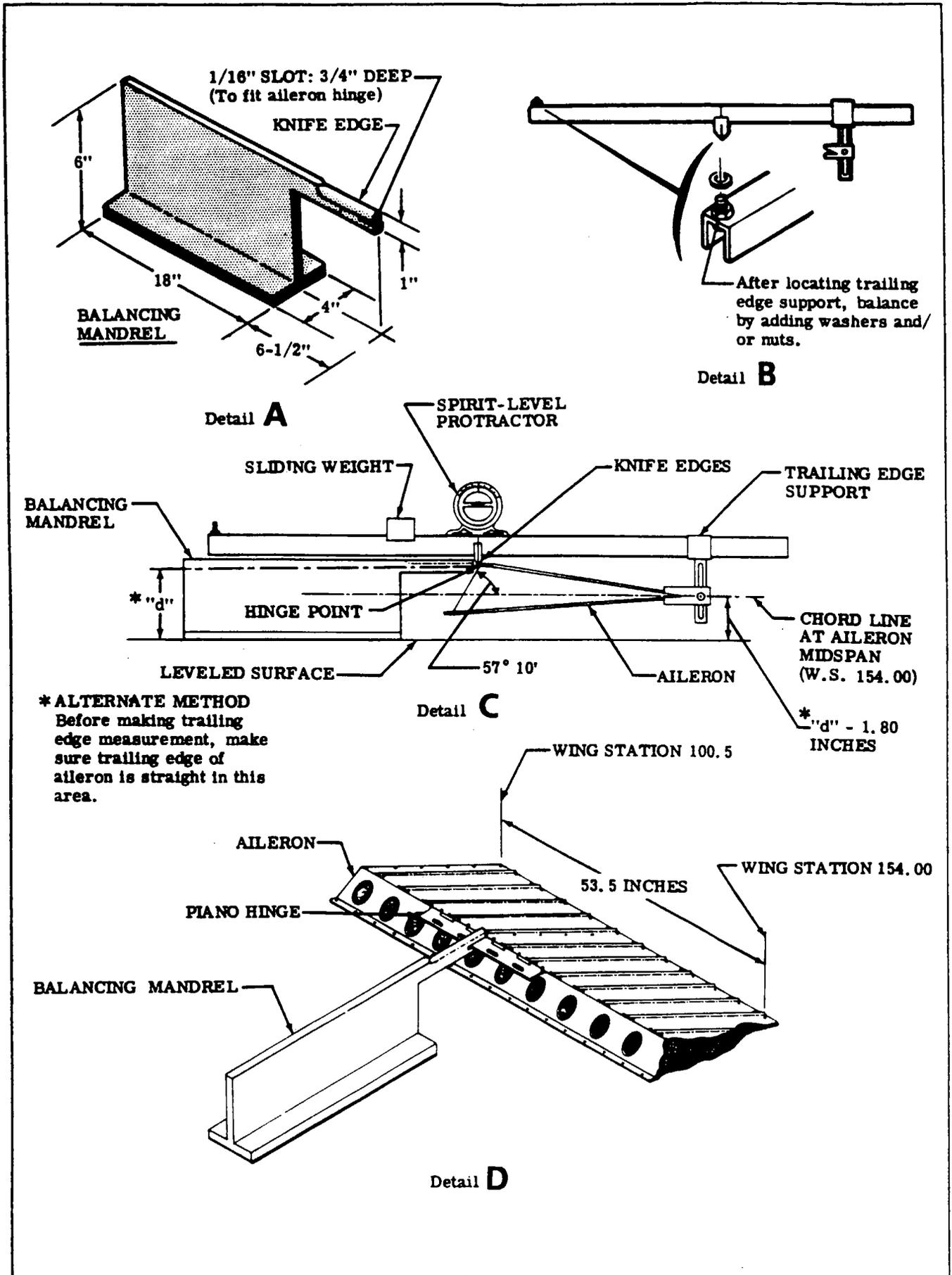
Figure 18-3. Control Surface Balancing (Sheet 4 of 5)
