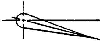
**OVERBALANCE** is defined as the condition that exists when surface is leading edge heavy and is defined by a symbol (-). If the balance beam sliding weight must be on the trailing edge side of the hinge line (to balance the control surface), the control surface is considered to be overbalanced.
