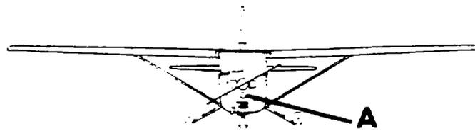
Park the aircraft 3 feet from a wall or any suitable light reflecting surface (distance is measured between landing light and wall). With the nose gear shock strut extended 2 inches, the center of the landing light beam on the wall should be 35 3/4 inches above the floor.
