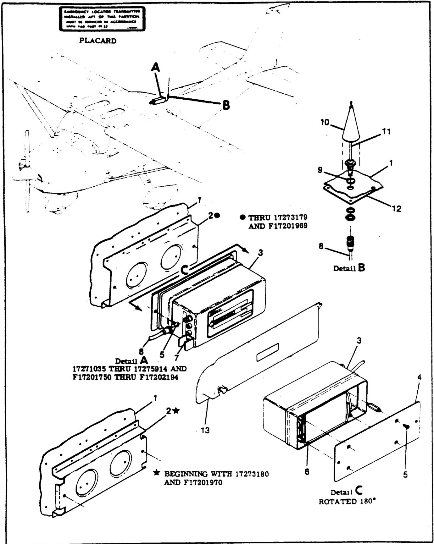
Figure 16-17. Emergency Locator Transmitter Installation (Sheet 2 of 3)
