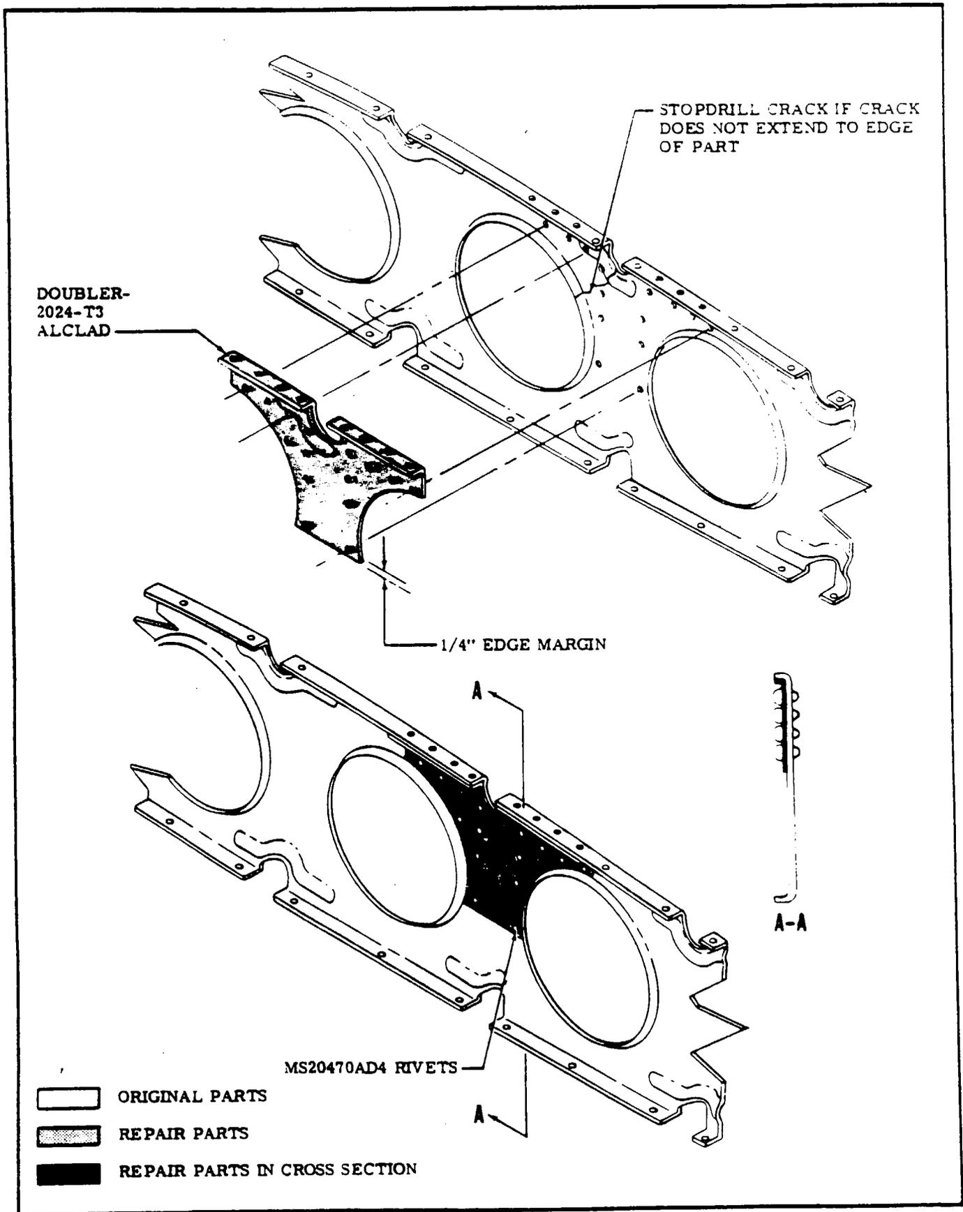
Figure 18-6. Rib Repair (Sheet 1 of 2)
