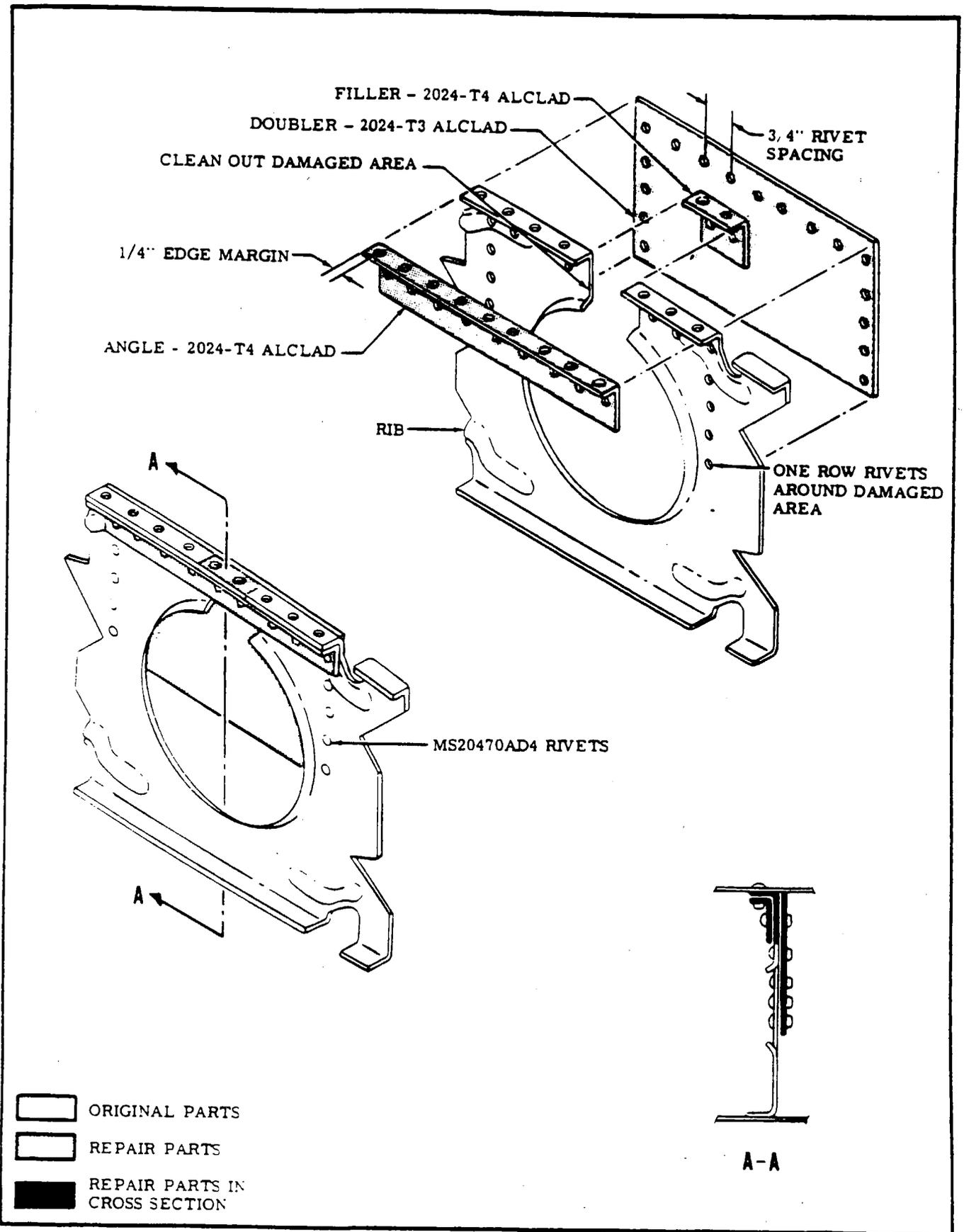
Figure 18-6. Rib Repair (Sheet 2 of 2)
