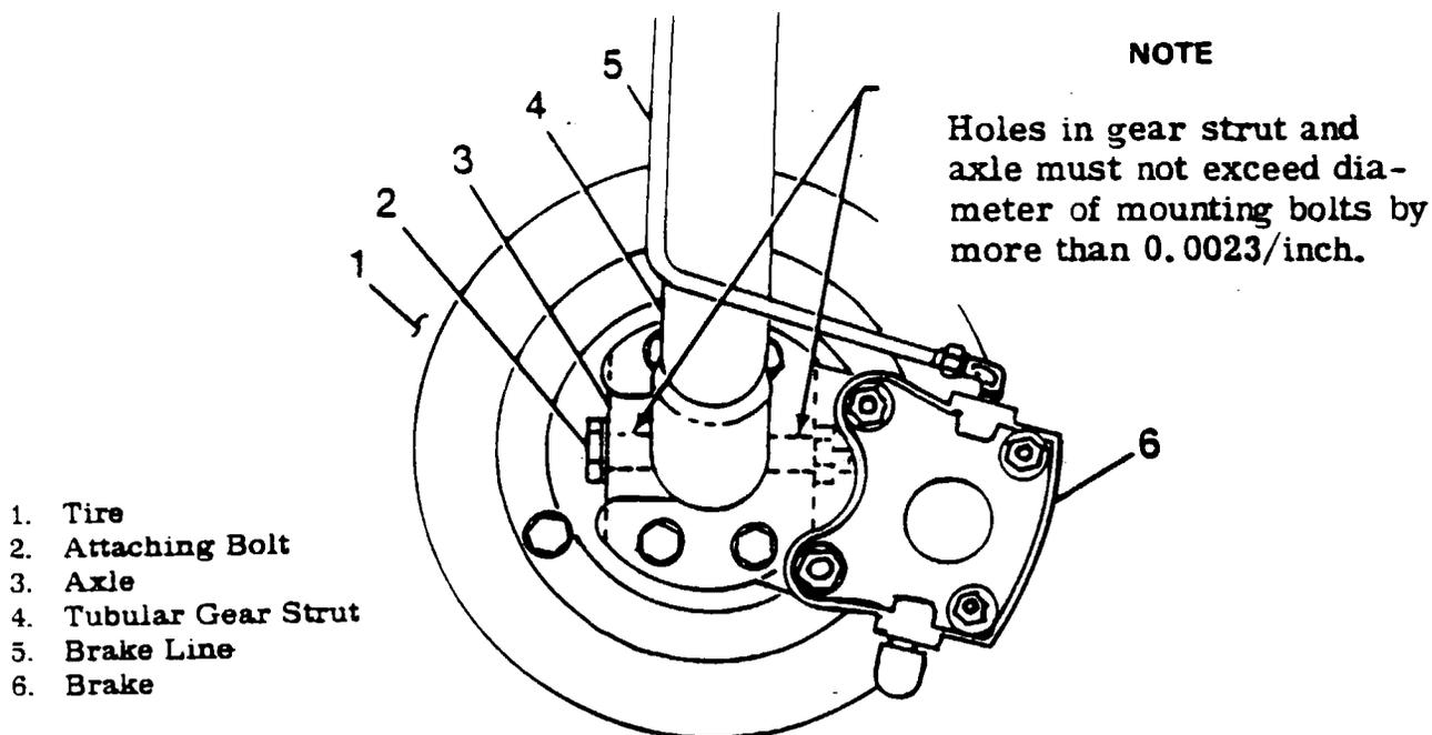
Figure 5-5. Installation of Main Wheel Strut to Axle Mounting Bolts.
