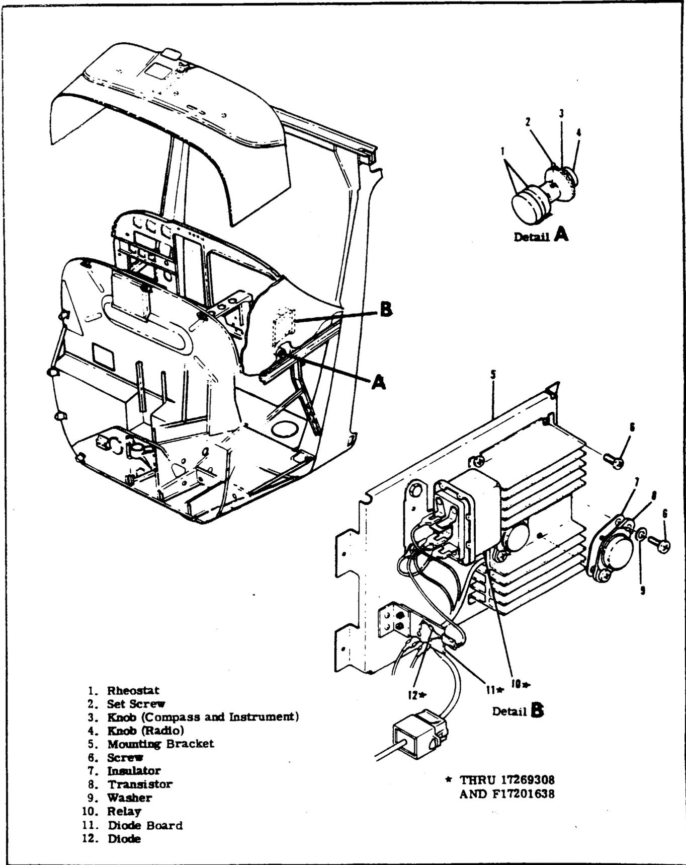
Figure 16-10. Transistorized Dimming
