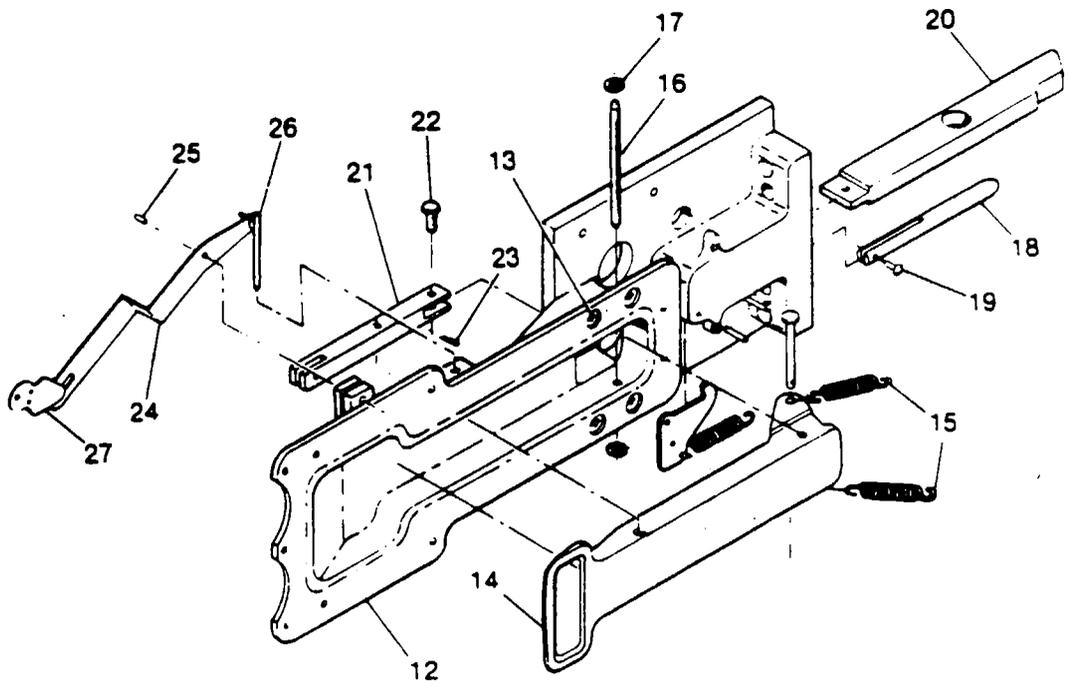
Figure 3-4A. Door Latch Installation
