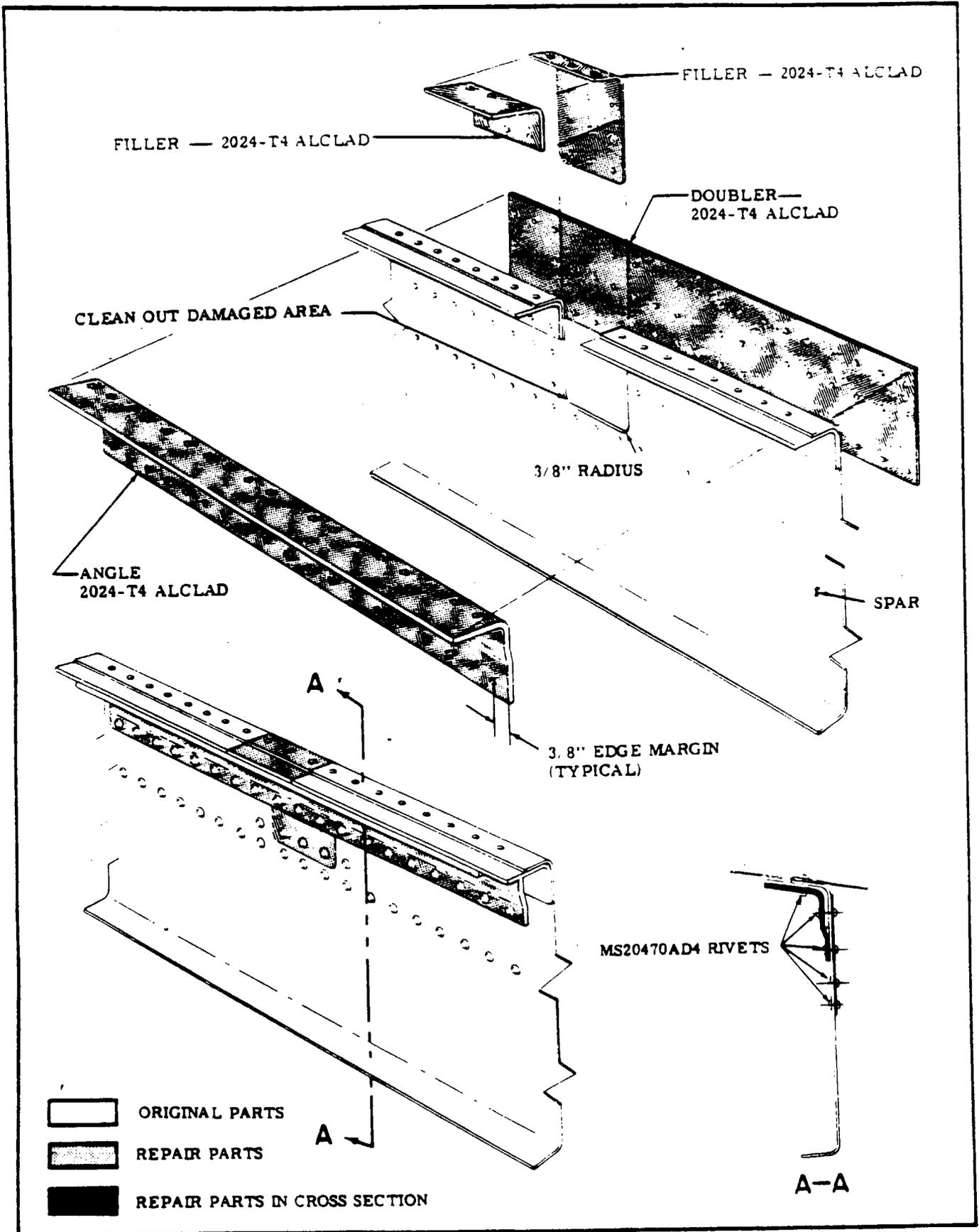
Figure 18-7. Wing Spar Repair (Sheet 1 of 3)
