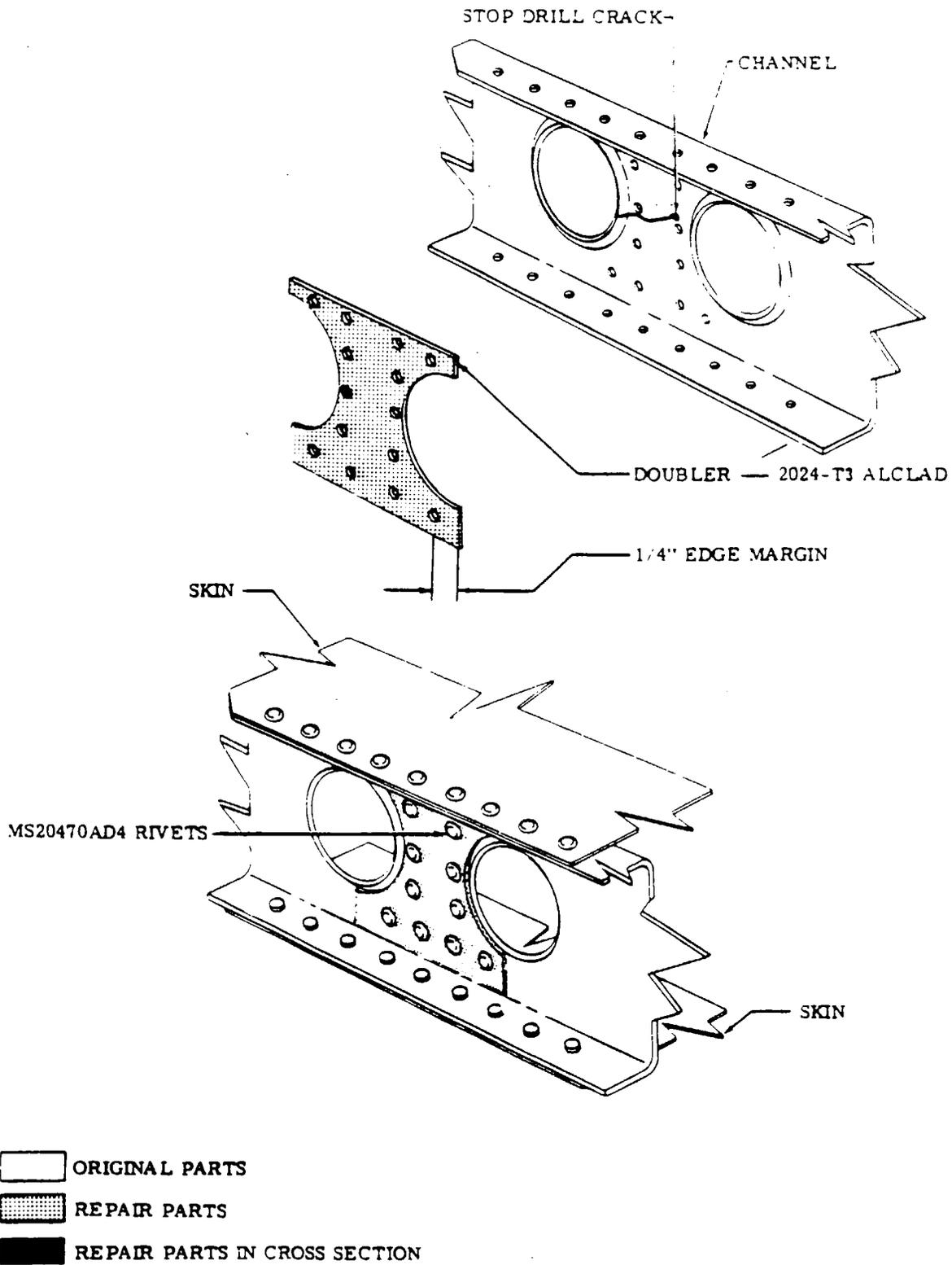
Figure 18-5. Stringer and Channel Repair (Sheet 3 of 4)
