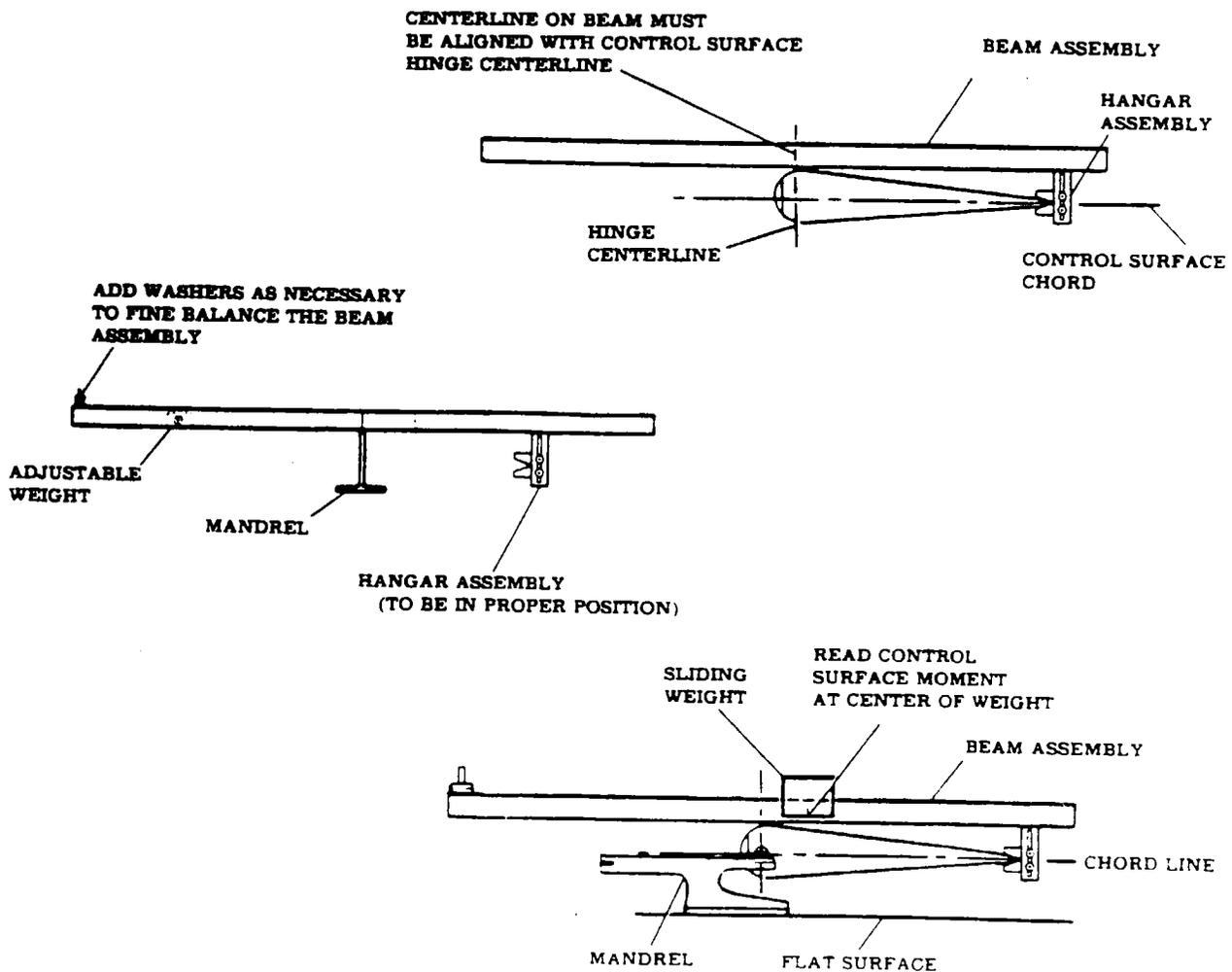
Figure 18-3. Control Surface Balancing (Sheet 2 of 5)
