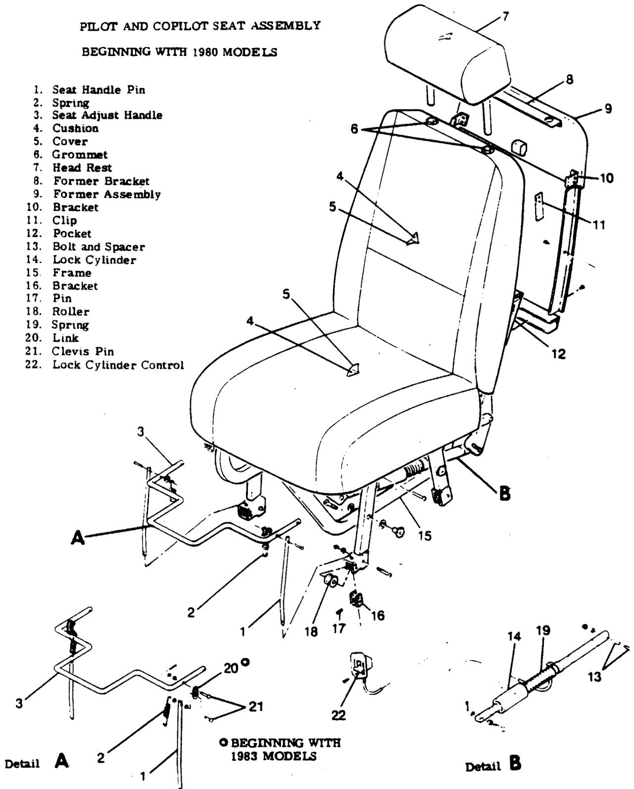
Figure 3-8. Seat Installation (Sheet 7 of 11)
