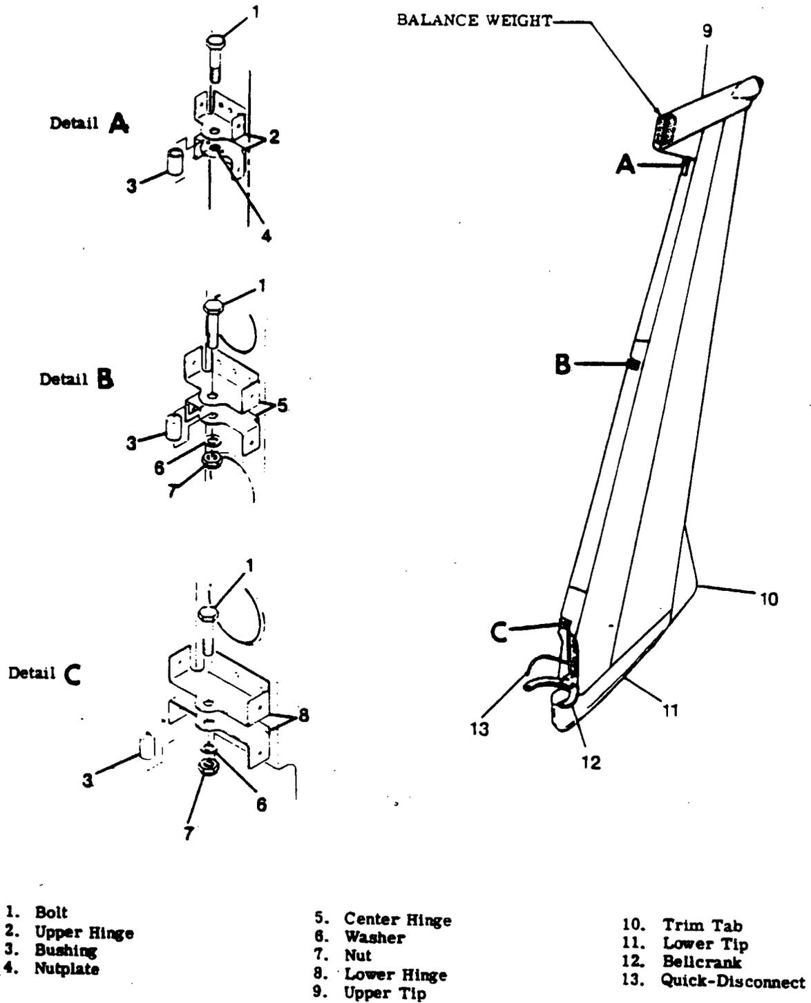
Figure 10-3. Rudder Assembly
