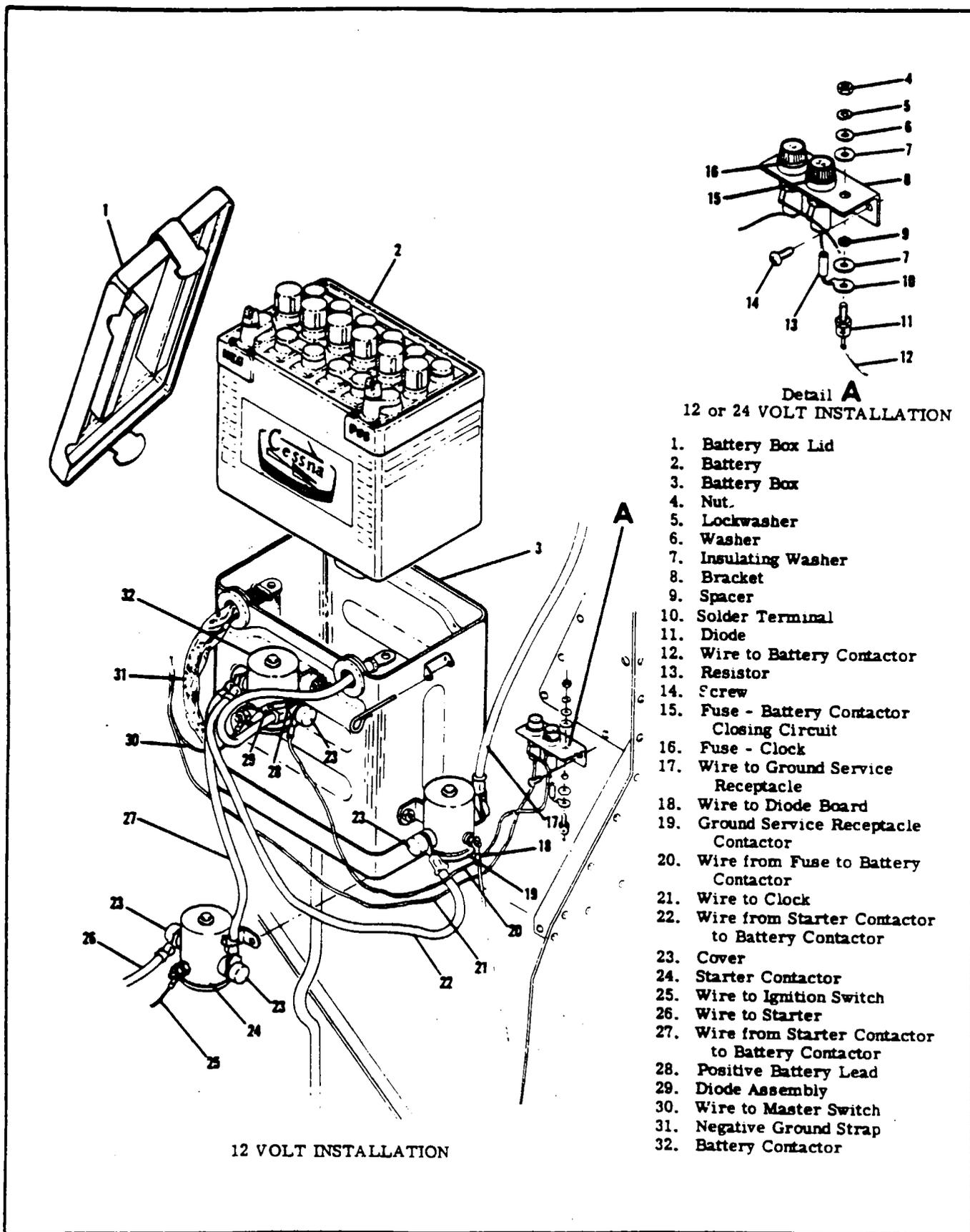
Figure 16-2. Battery and Electrical Equipment Installation (Sheet 1 of 7)
