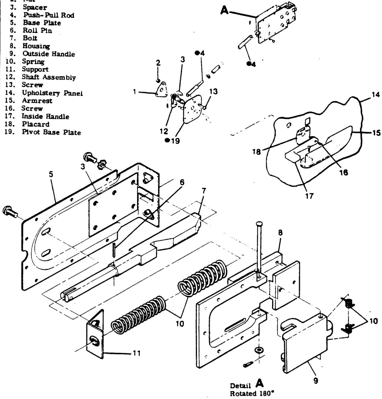
Figure 3-4. Door Latch Installation
