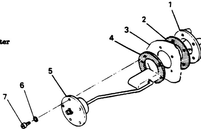
Beginning with Serial 17267585 thru 17276330, 17276331, nutring (1) is bonded to root rib (2). Order sealant kits SK210-56, or SK210-101, from Cessna Supply Division.
