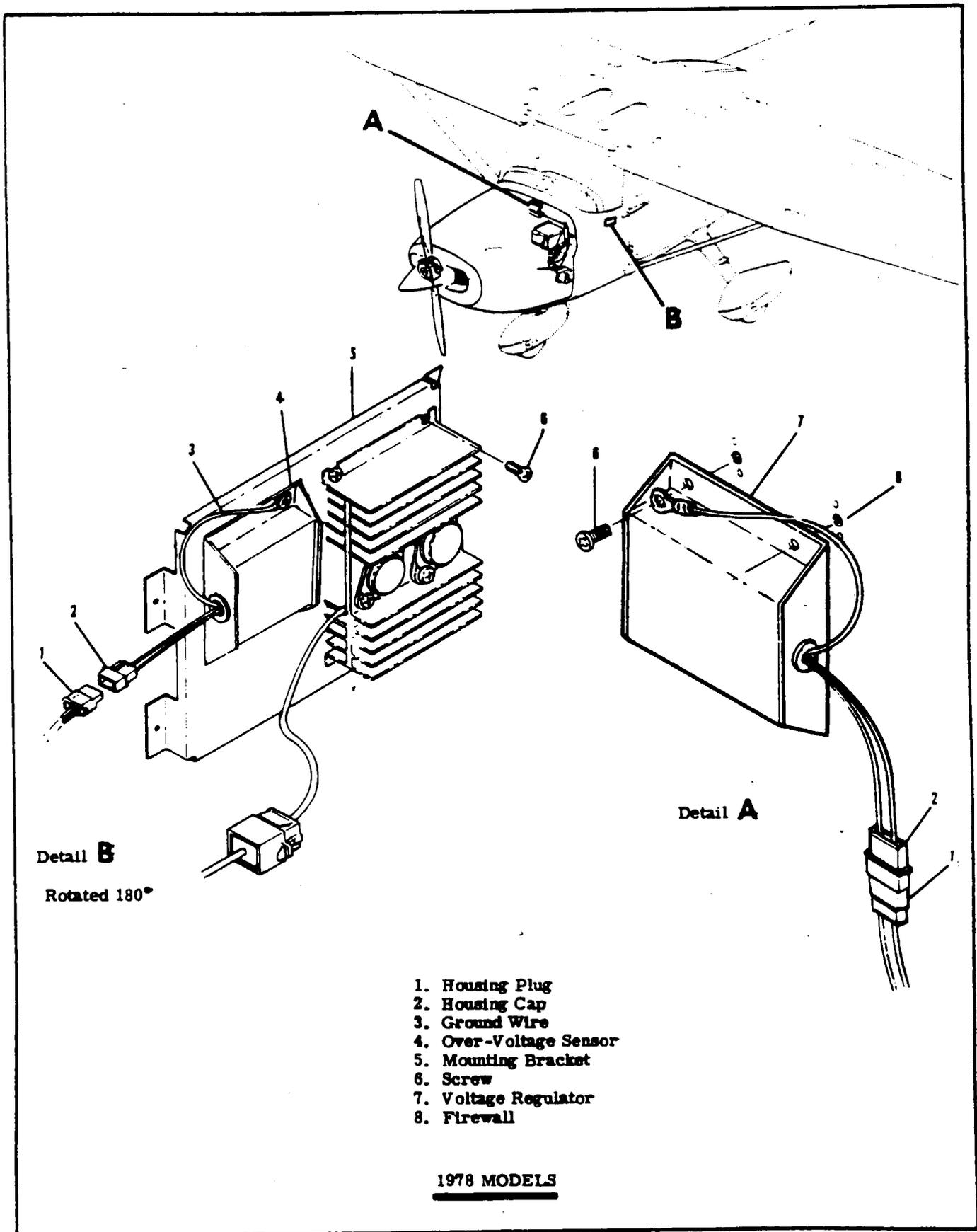
Figure 16-5. Voltage Regulator Installation (Sheet 2 of 5)
