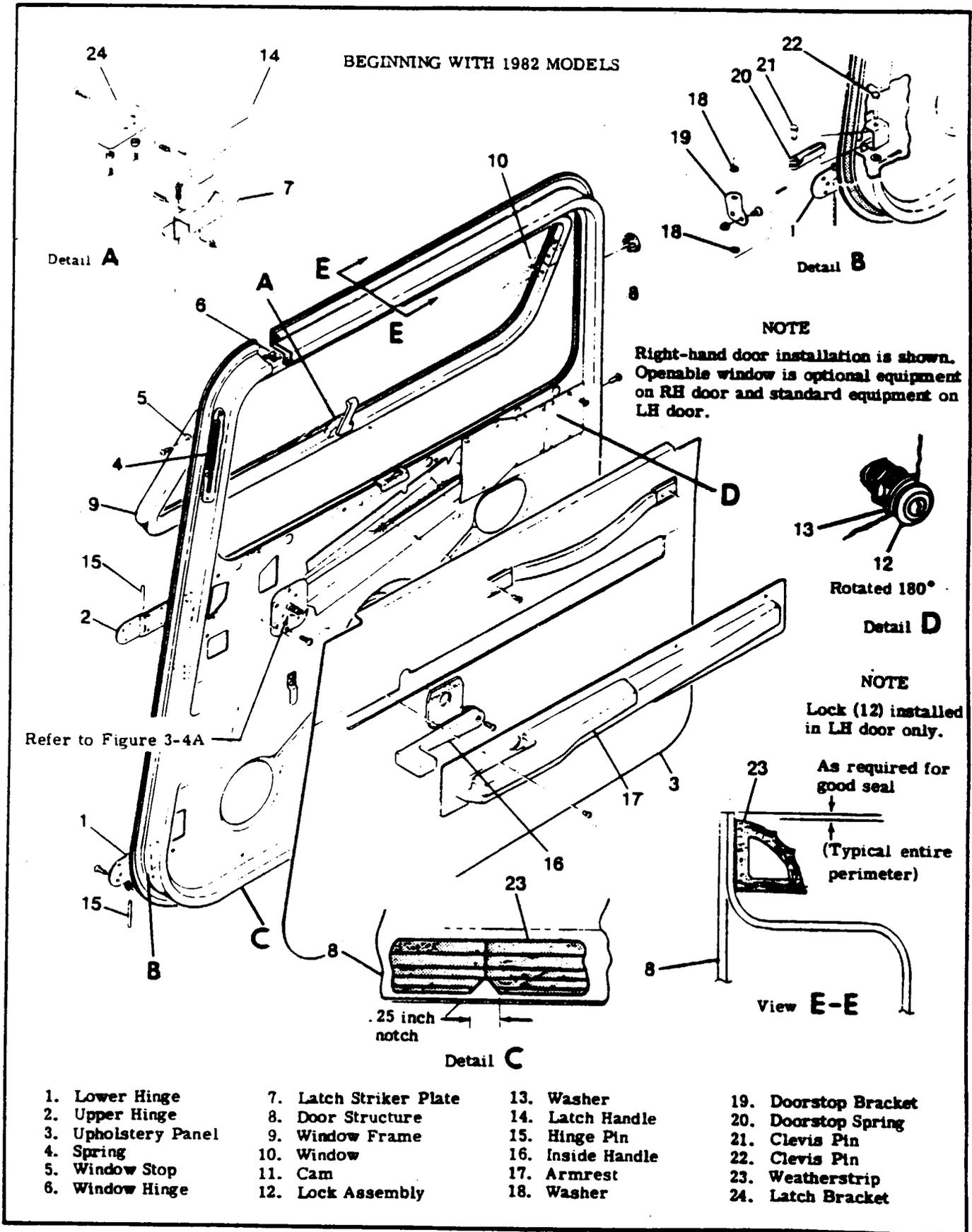
Figure 3-3. Cabin Door Installation (Sheet 3 of 3)
