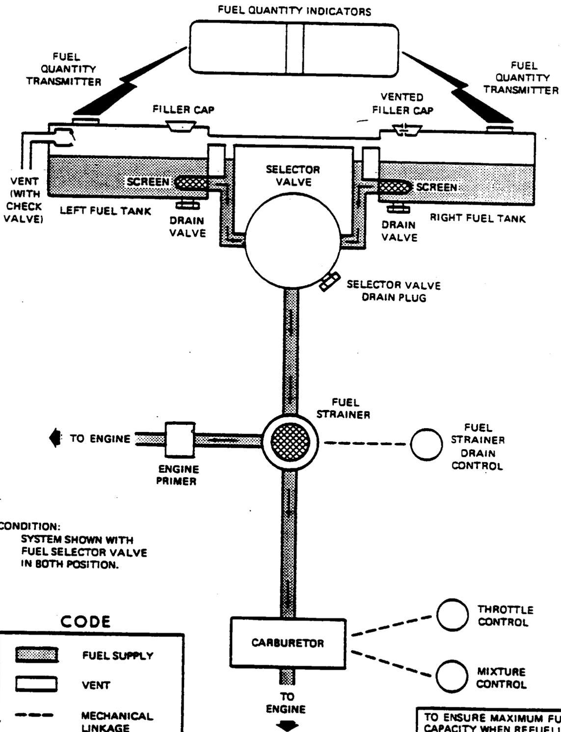
Figure 12-1. 172 Fuel System Schematic (Sheet 1 of 2)
