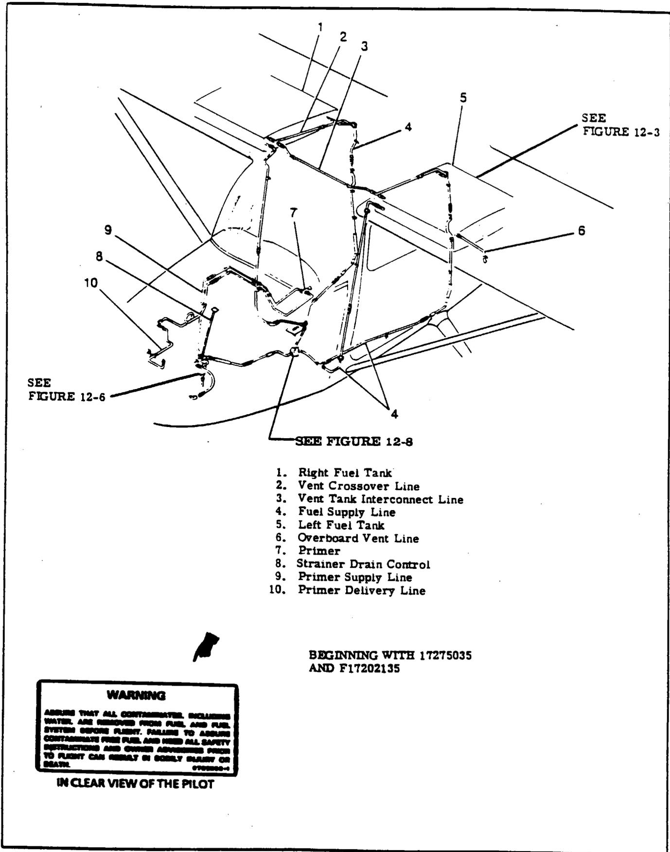
Figure 12-2. Fuel System (Sheet 2 of 2)
