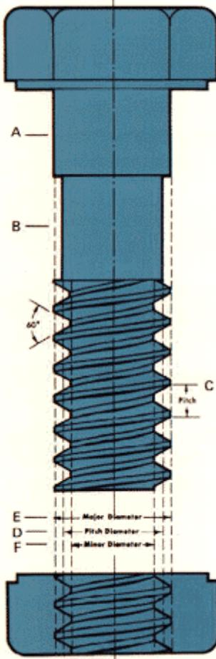
Used principally for studs and their mating tapped holes. A force fit requiring the application of high torque for semi-permanent assembly.
