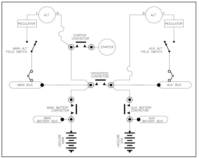
Figure 17-5. Dual Alternator, Dual Battery Electrical systems.
