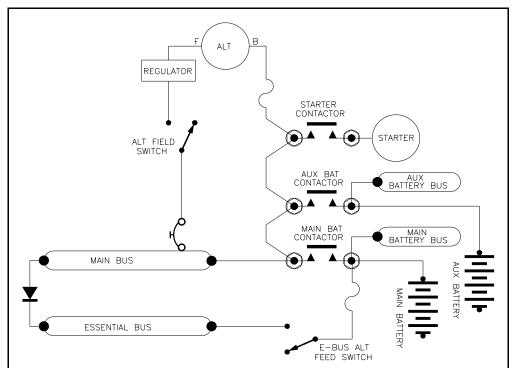
Figure 17-6. Dual Battery Installation
