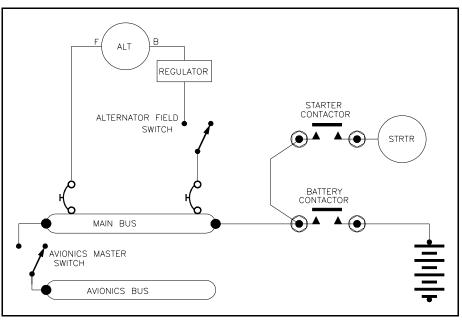
Figure 17-1. Rudimentary Single Battery, Single Alternator Power Distribution System.
