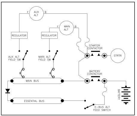
Figure 17-8 Auxiliary Alternator with Autoswitching.
