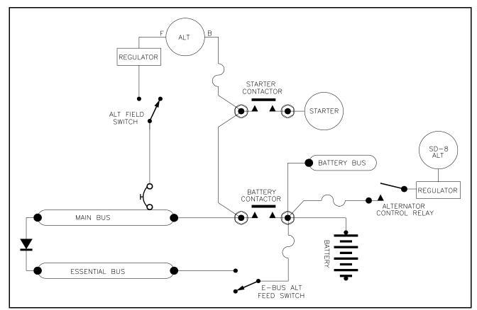
Figure 17-4. Adding the SD-8 Auxiliary Alternator
