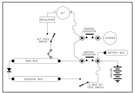
Figure 17-3... Addition of an Always Hot Battery Bus.
