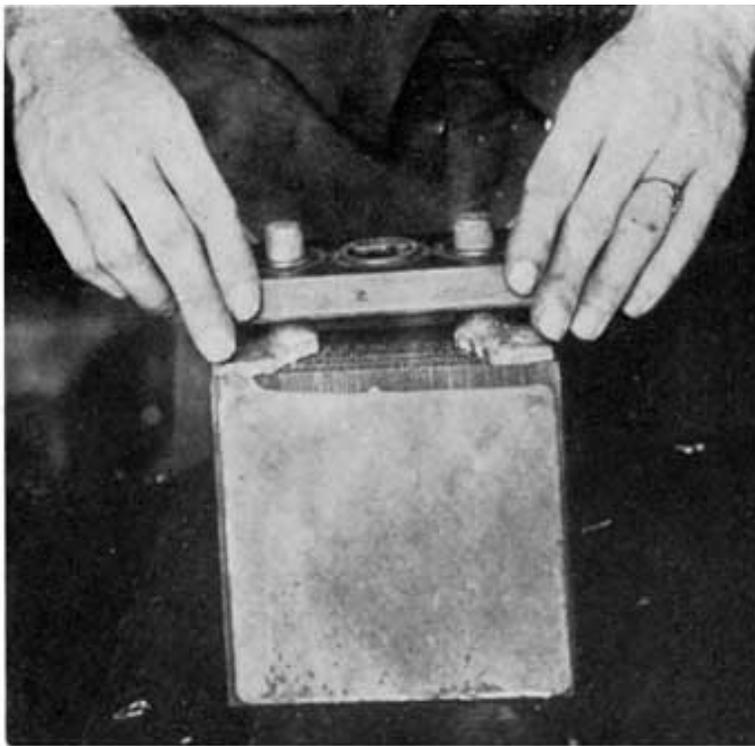
Fig. 258. Replacing Cover of Philadelphia Diamond Grid Battery
