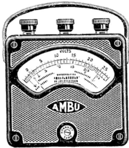
Fig. 121. Special Cadmium Test Voltmeter
