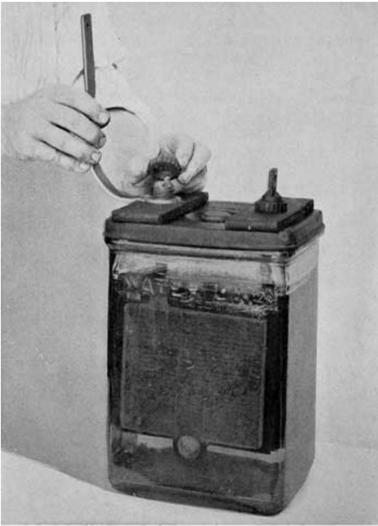
Fig. 321. Fastening Auxiliary Strap. Delco-Light Cell
