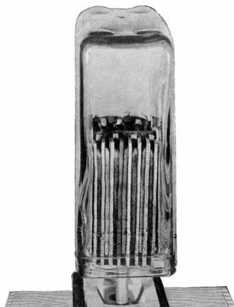
Turn the element upside down and place over a block of wood so that the weight is supported by the cover. (See Fig. 332.)
