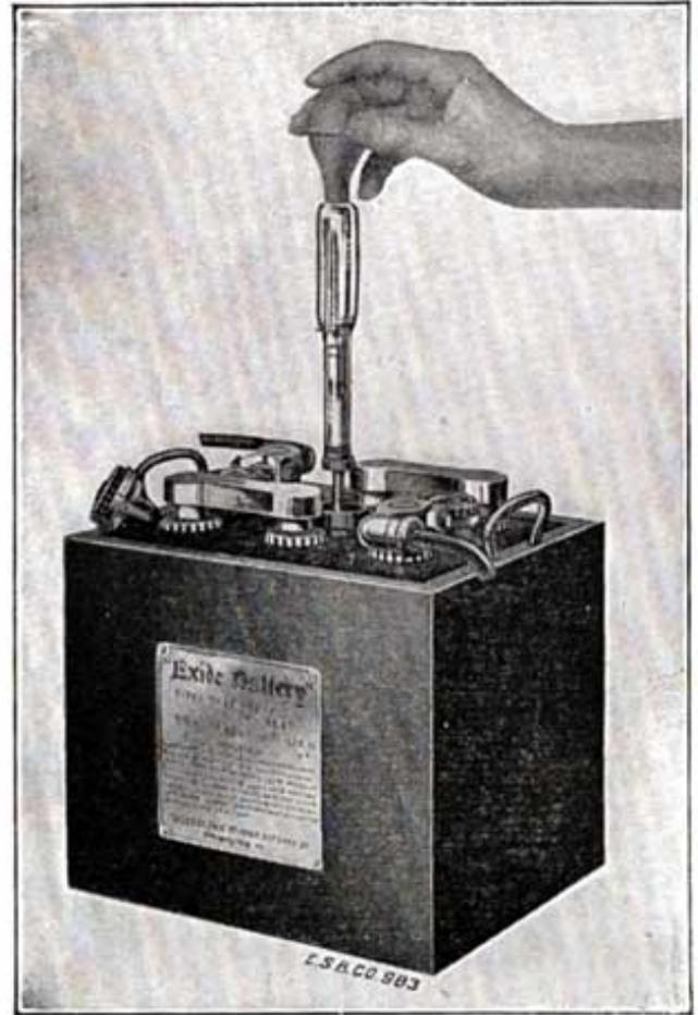
Fig. 35. Taking a Specific Gravity Reading
