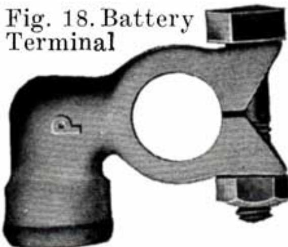
Many types of terminals are in two parts, one being permanently attached to the car circuit and the other mounted permanently on the battery by welding it to the terminal post, the two parts being detachably joined by means of a bolted connection.
