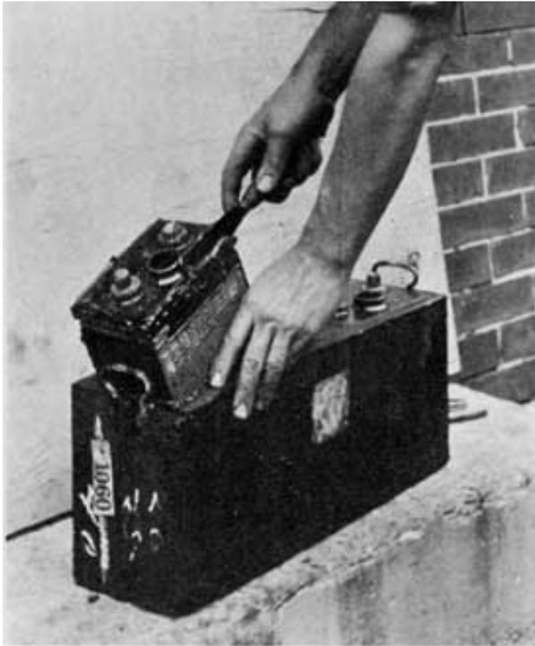
Fig. 198. Removing Compound from Cover
