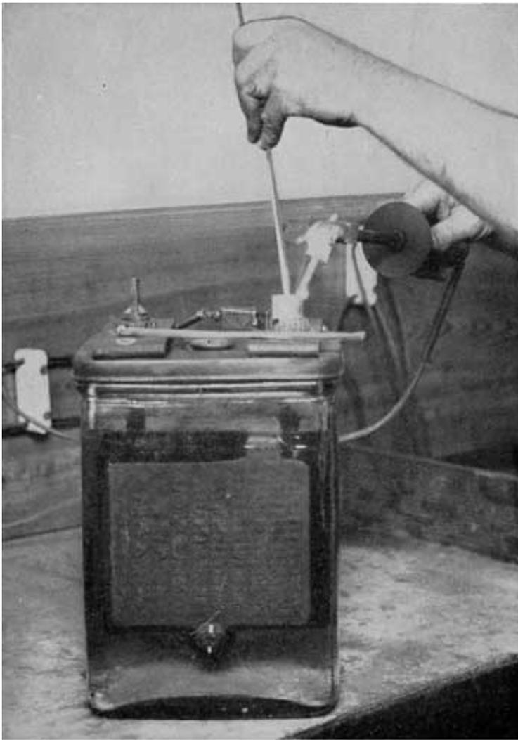
Fig. 319. Burning on Negative Strap. Delco-Light Cell
