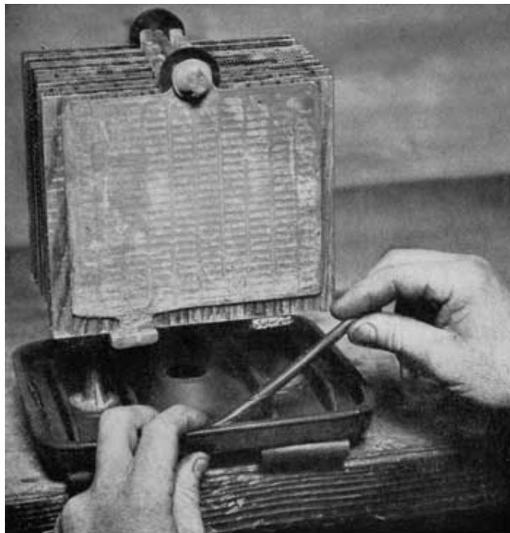
Fig. 314. Preparing Cover for Sealing. Delco-Light Cell
