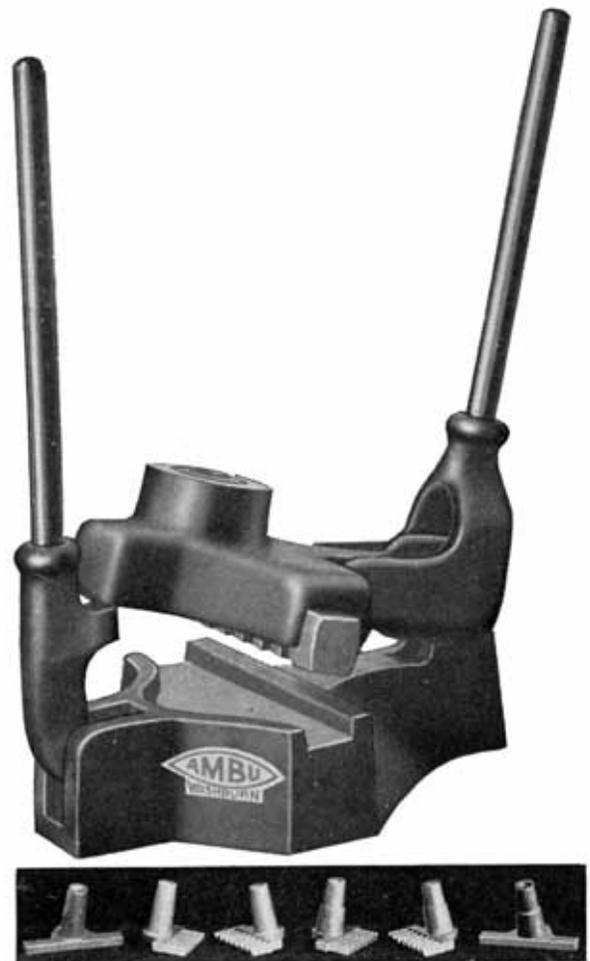
Fig. 102. Plate Strap Mould
