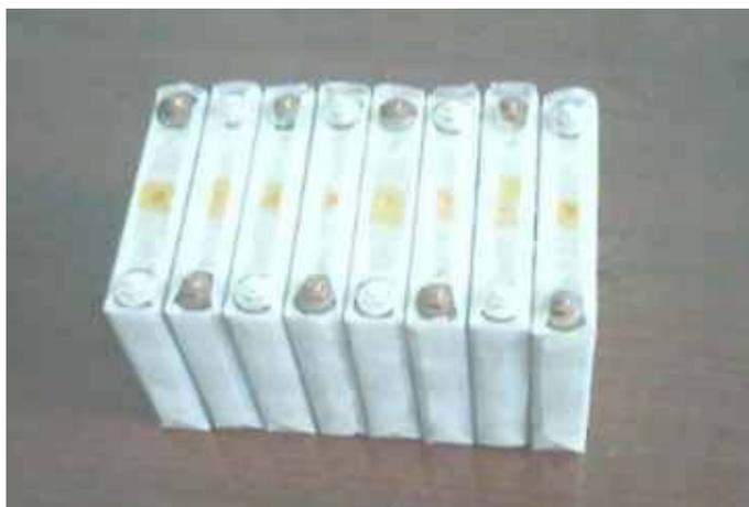
Lithium Iron phosphate batteries are safer than Lithium-ion cells, and are available in 10 and 20 AH packs with much longer life.
