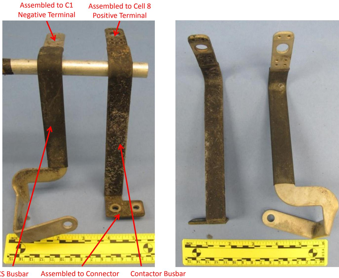
Figure 40. Two photos of the C1-J3 and C8-contactor busbars.
