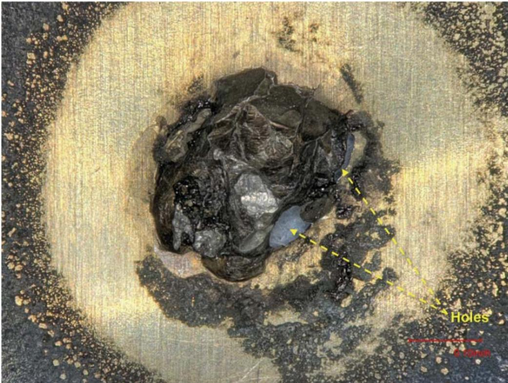
Figure 53. The protrusion on the exterior of the battery box, after cleaning (~200X). The largest holes (arrows) are labeled and exhibit a light-blue color from the backing paper used during photographing.
