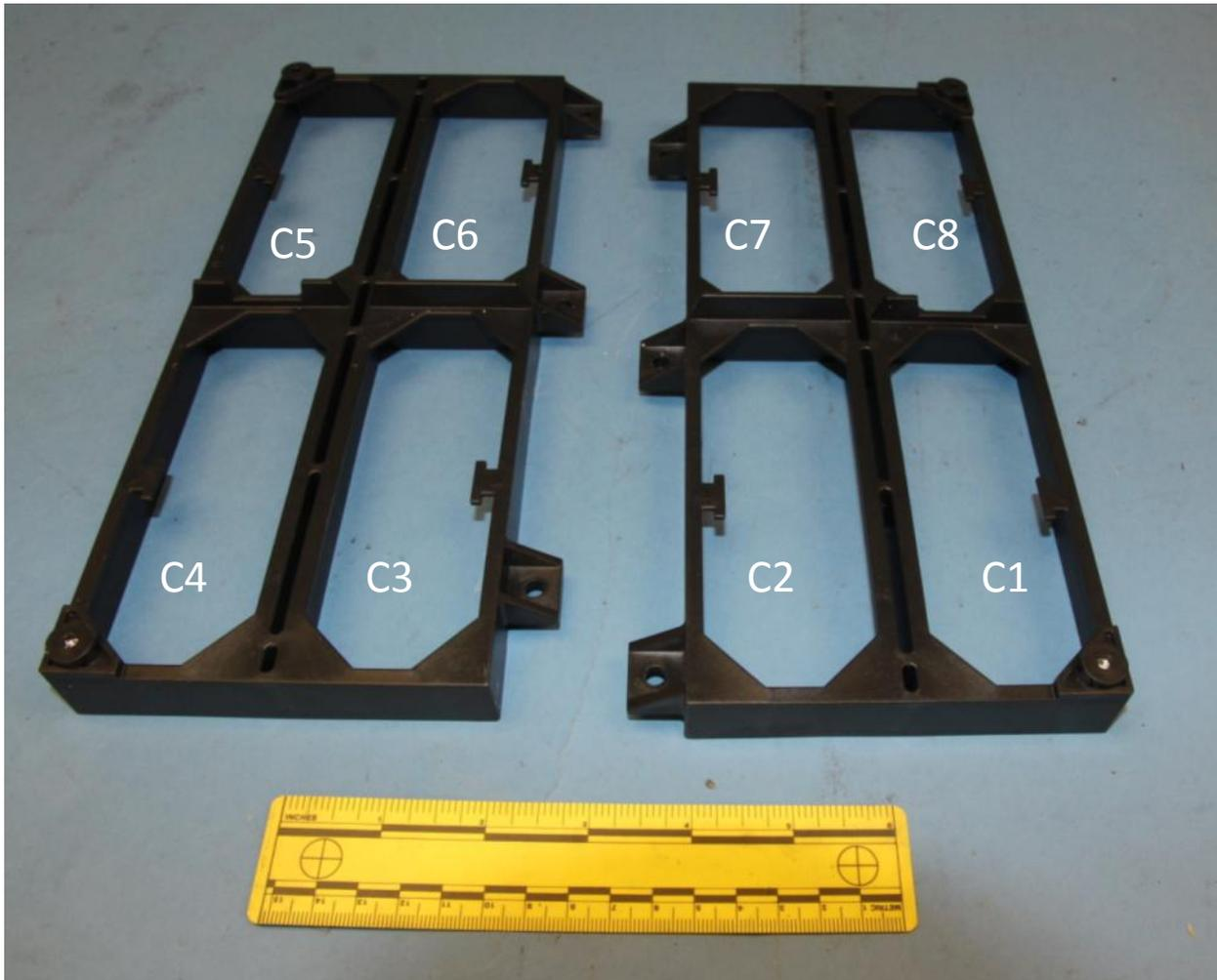
Figure 81. Upper fixation trays (top down view) of the JAL exemplar, main battery.
