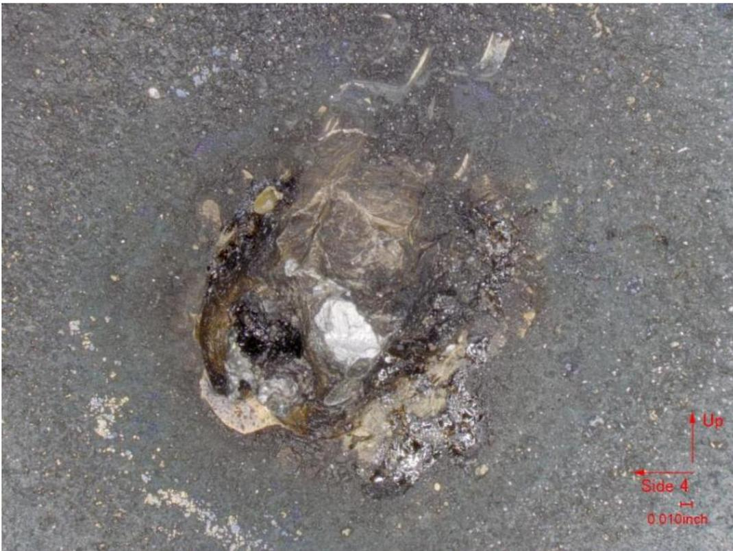
Figure 50. Close-up view of the protrusion on the battery box exterior, as received (~200X).
