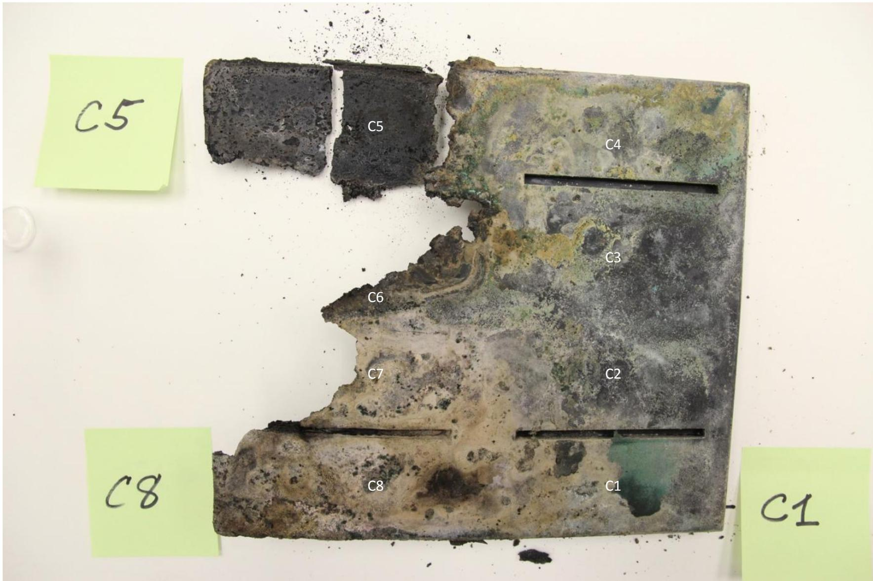
Figure 89. Bottom view of lower fixation tray, which is made of thermoplastic polyester.
