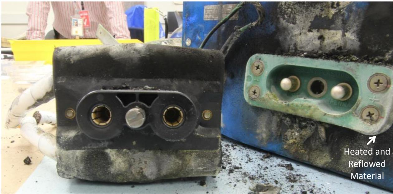
Figure 99. Close-up view of both the J3 power connector and the power receptacle.
