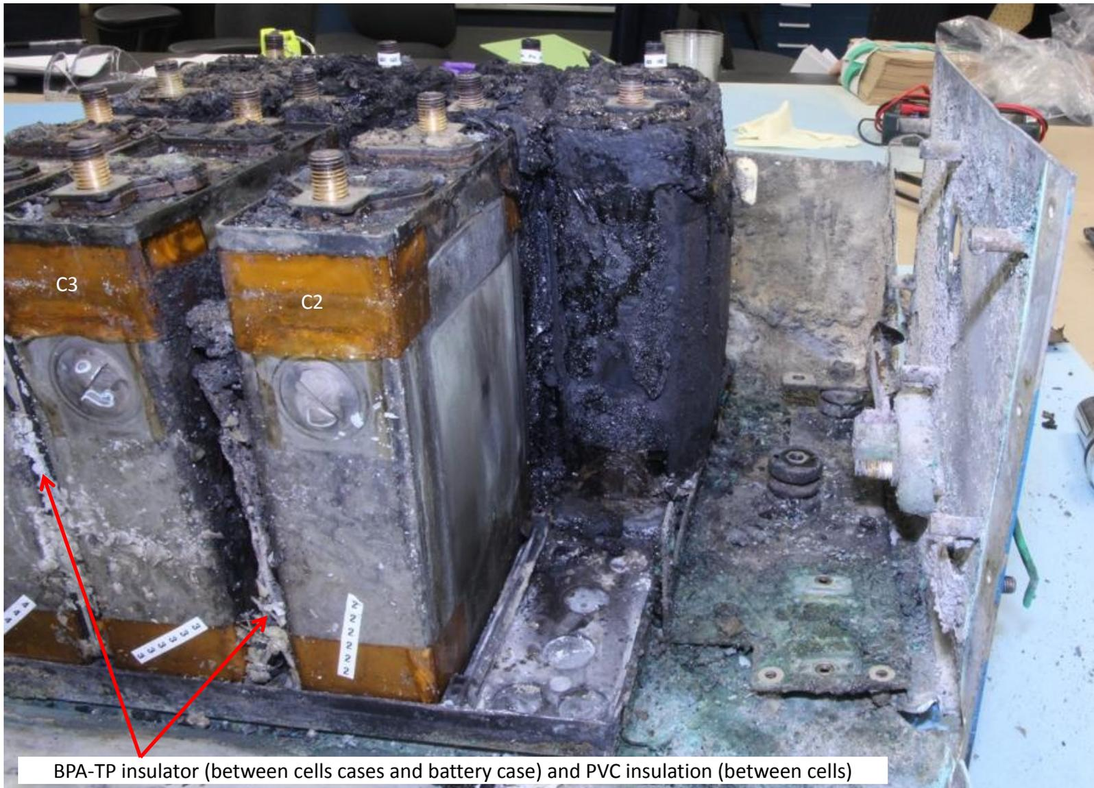
BPA-TP insulator (between cells cases and battery case) and PVC insulation (between cells)
