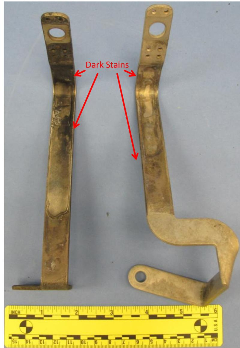
Figure 44. Two views of the C1-J3 and C8-contactor busbars.
