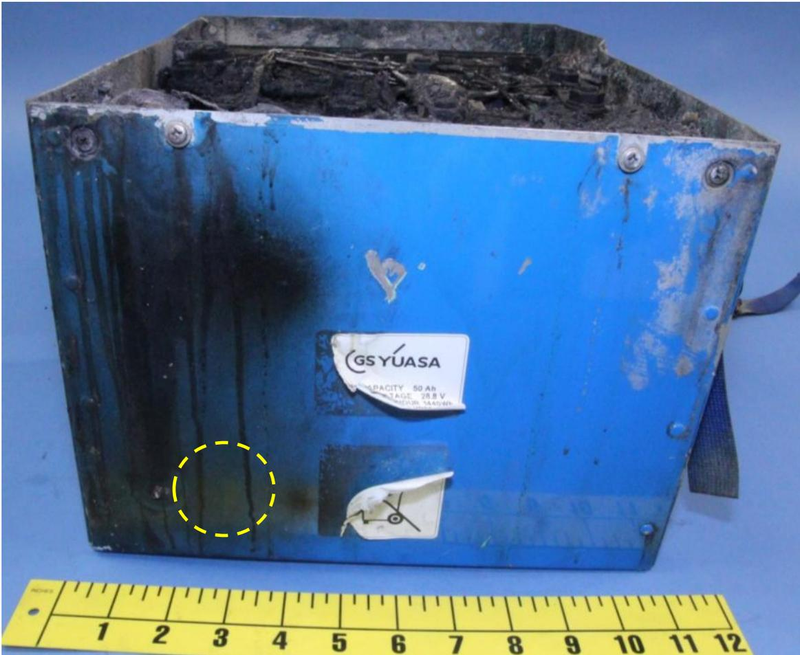
Figure 48. S3 of the exterior of the battery box. The highlighted area shows the small protrusion on the lower left side. This area is magnified in Figure 49.
