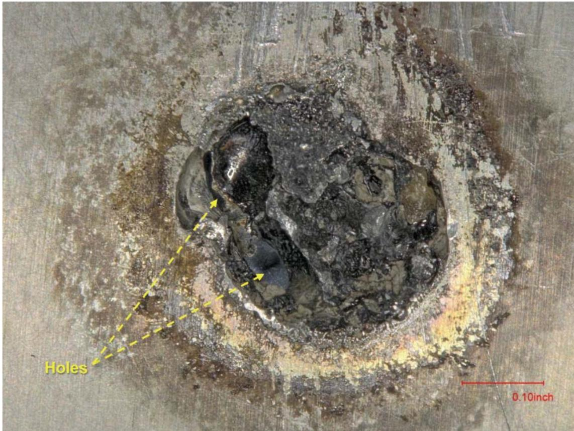
Figure 55. The protrusion on the interior of the battery box, after cleaning (~200X). The largest holes (arrows) are labeled and exhibit a light-blue color from the backing paper used during photographing.
