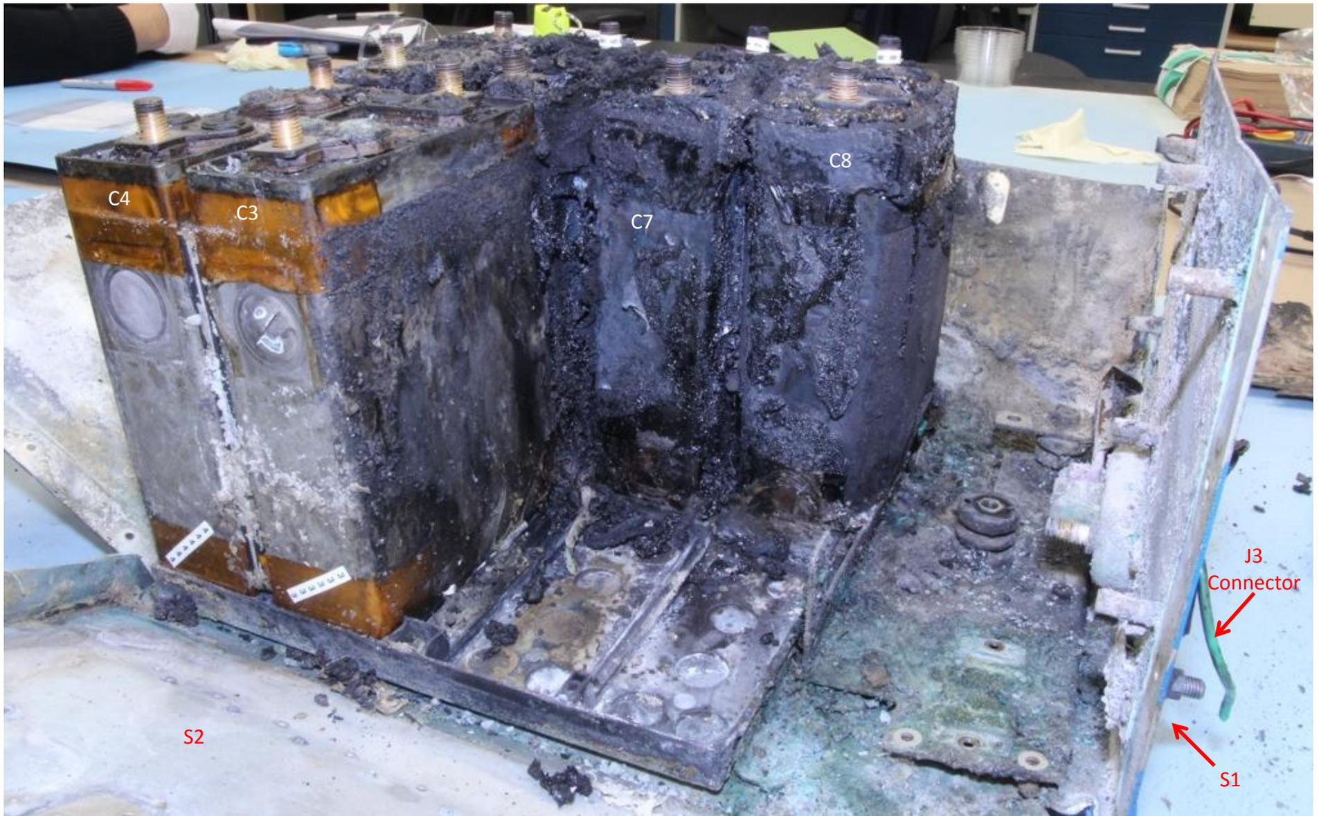
Figure 87. Battery box with C2 removed (viewed from S2).
