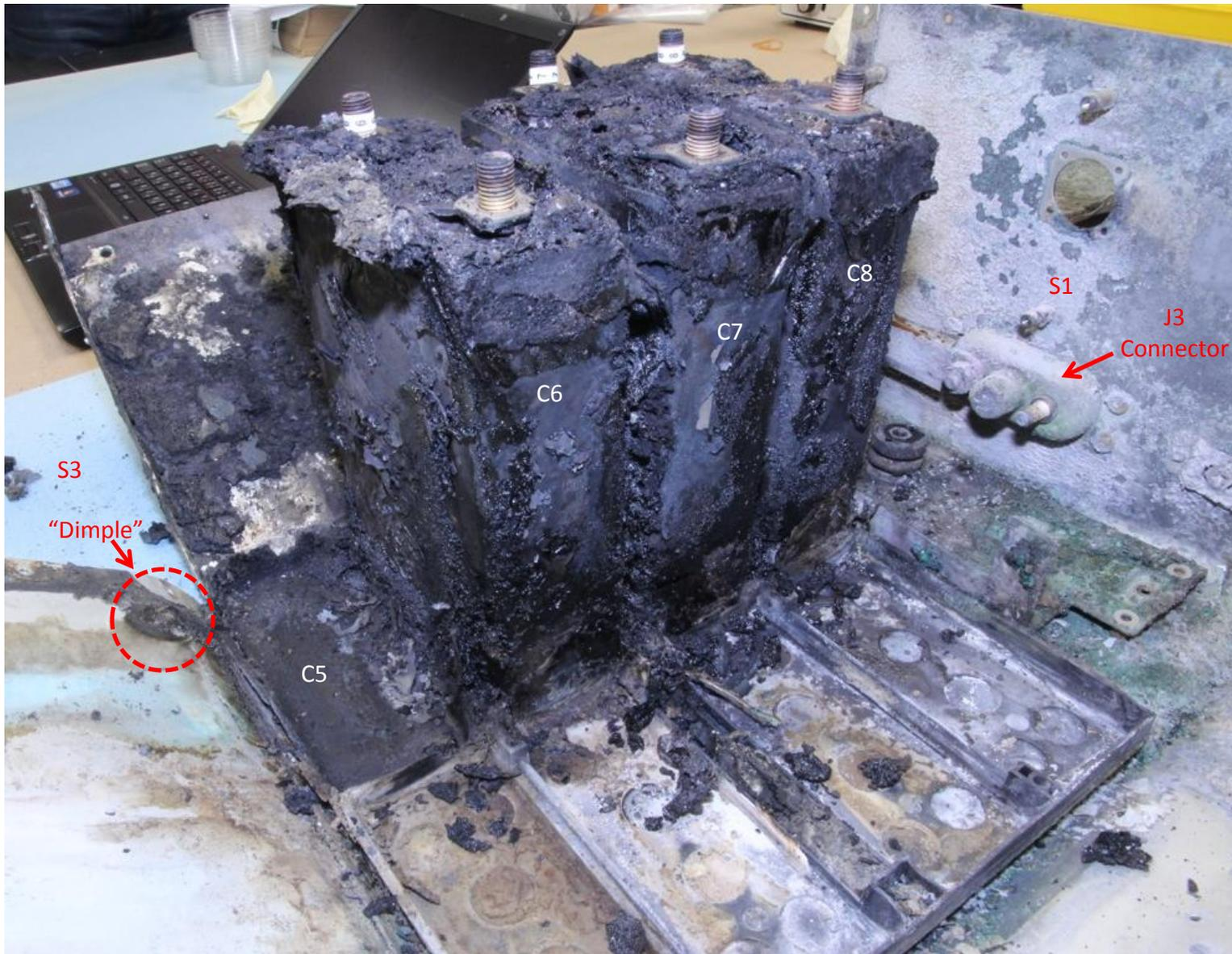
Figure 96. Battery box with C1 through C5 removed (viewed from S2).
