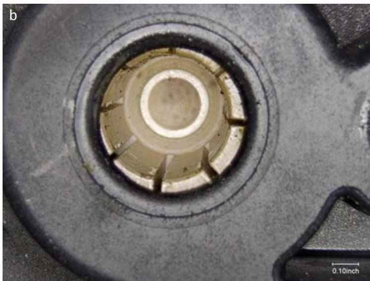
Figure 102. Close-up views of the power connector.
