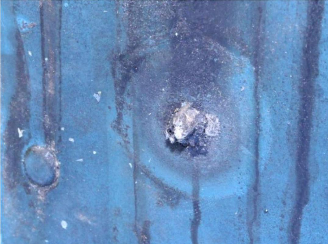
Figure 49. The protrusion from the exterior of S3 of the battery box, as received.
