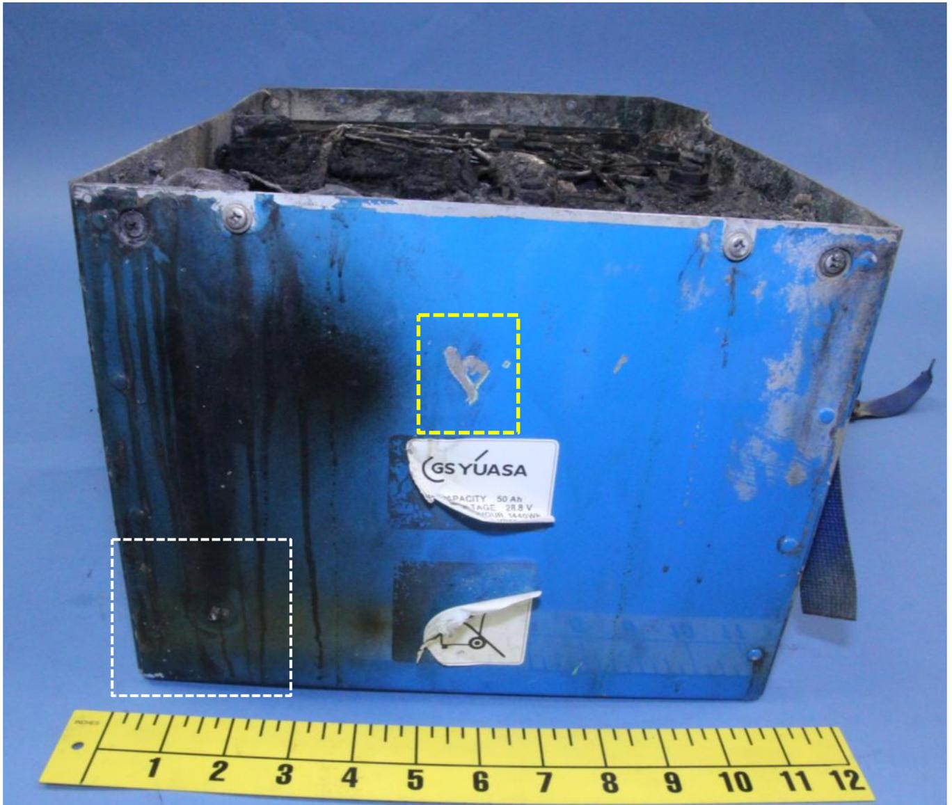
Figure 13. View of S3 exterior damage. The white highlighted area is a nodular protrusion. The yellow highlighted area shows a gouge.
