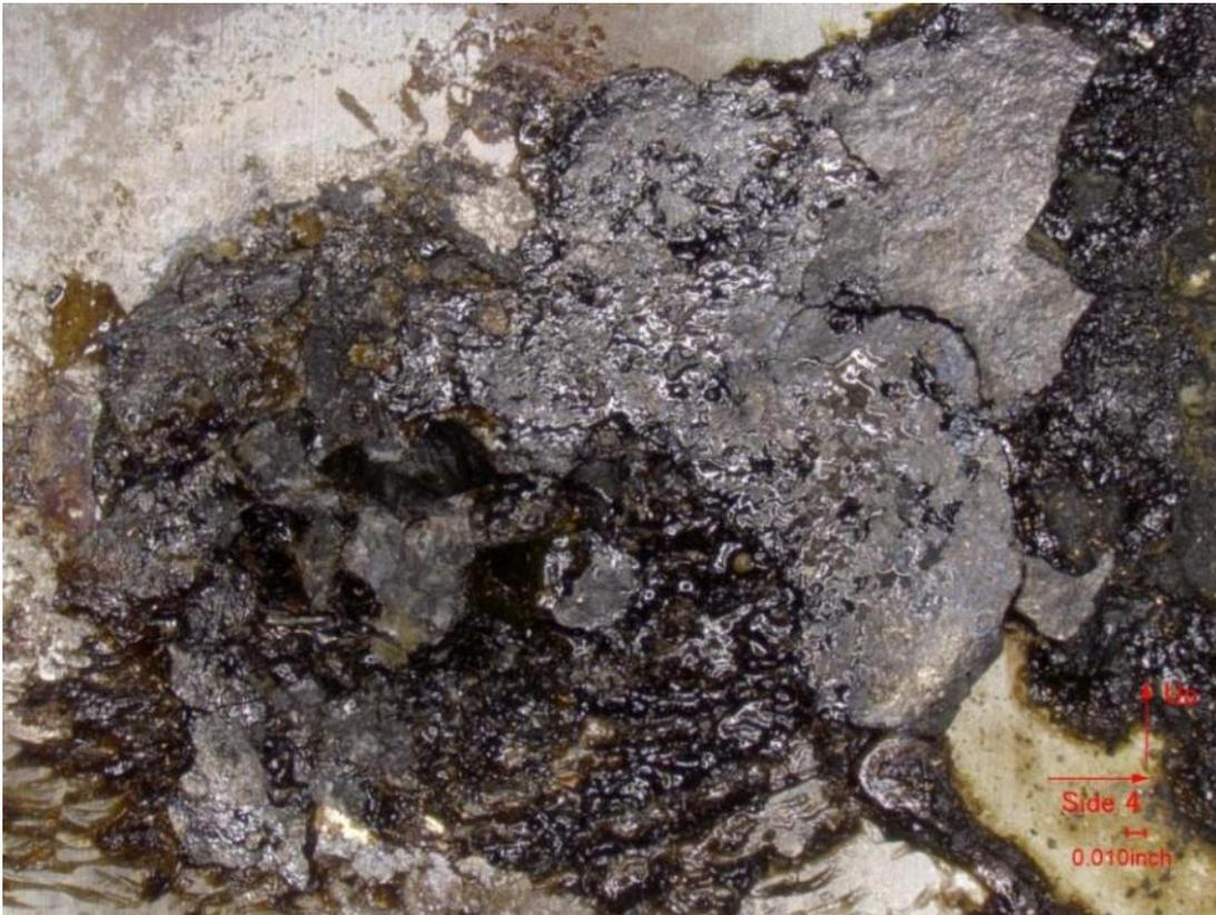
Figure 51. Close-up view of the protrusion on the battery box interior, as received (~200X).
