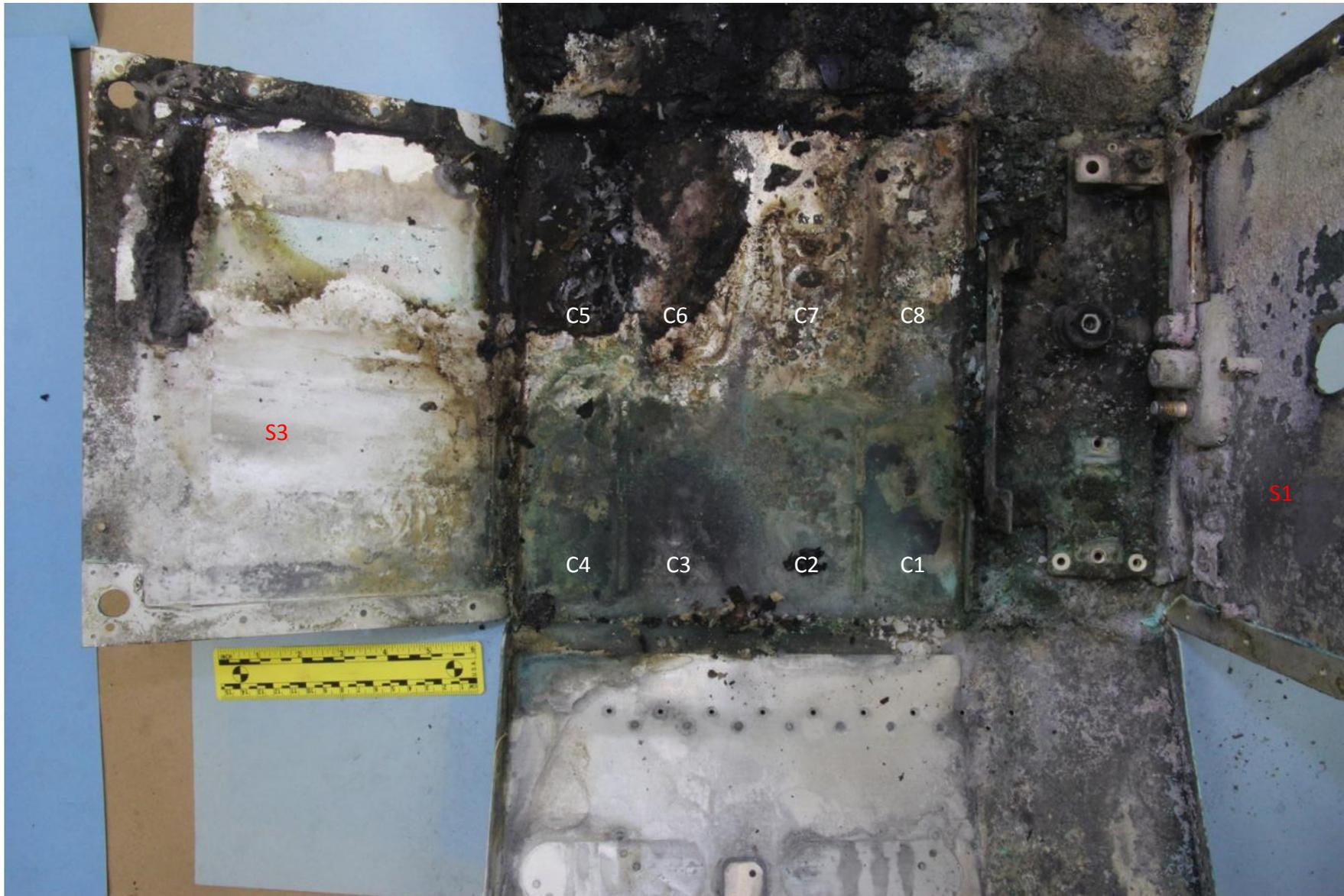
Figure 80. Battery box with all cells removed (another view from the top of the battery box).
