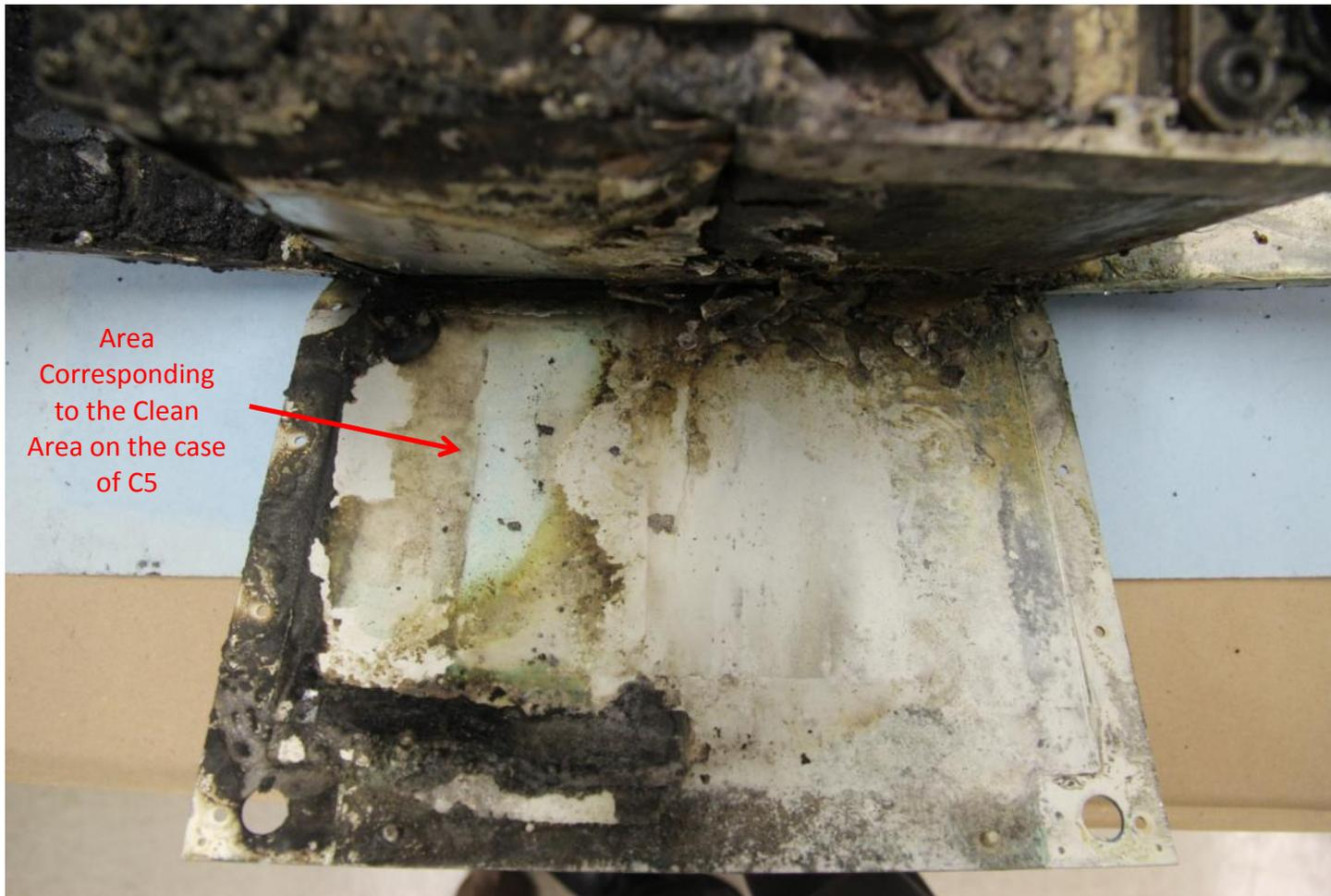
Figure 29. S3 battery box side interior.
