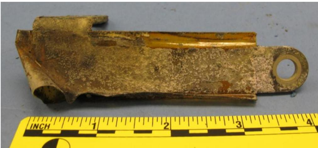
Figure 43. Two views of the contactor-J3 busbar.
