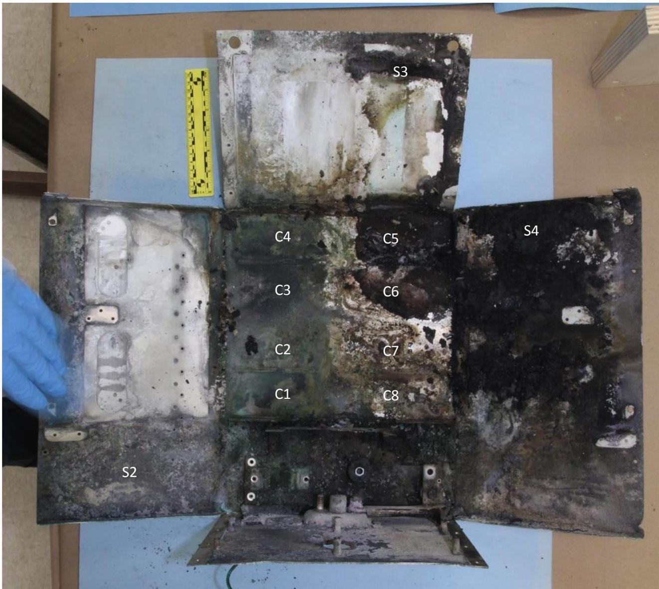
Figure 78. Battery box with all cells removed (viewed from the top of the battery box).
