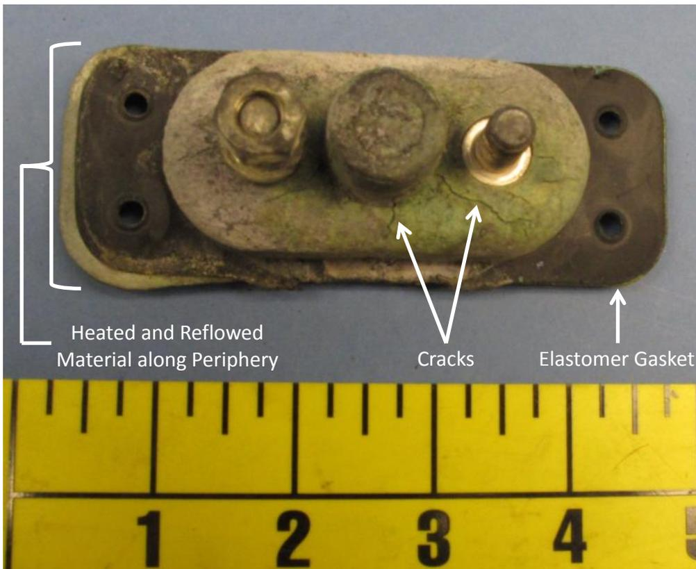
Figure 100. Close-up view of the J3 power receptacle showing heated and reflowed material.
