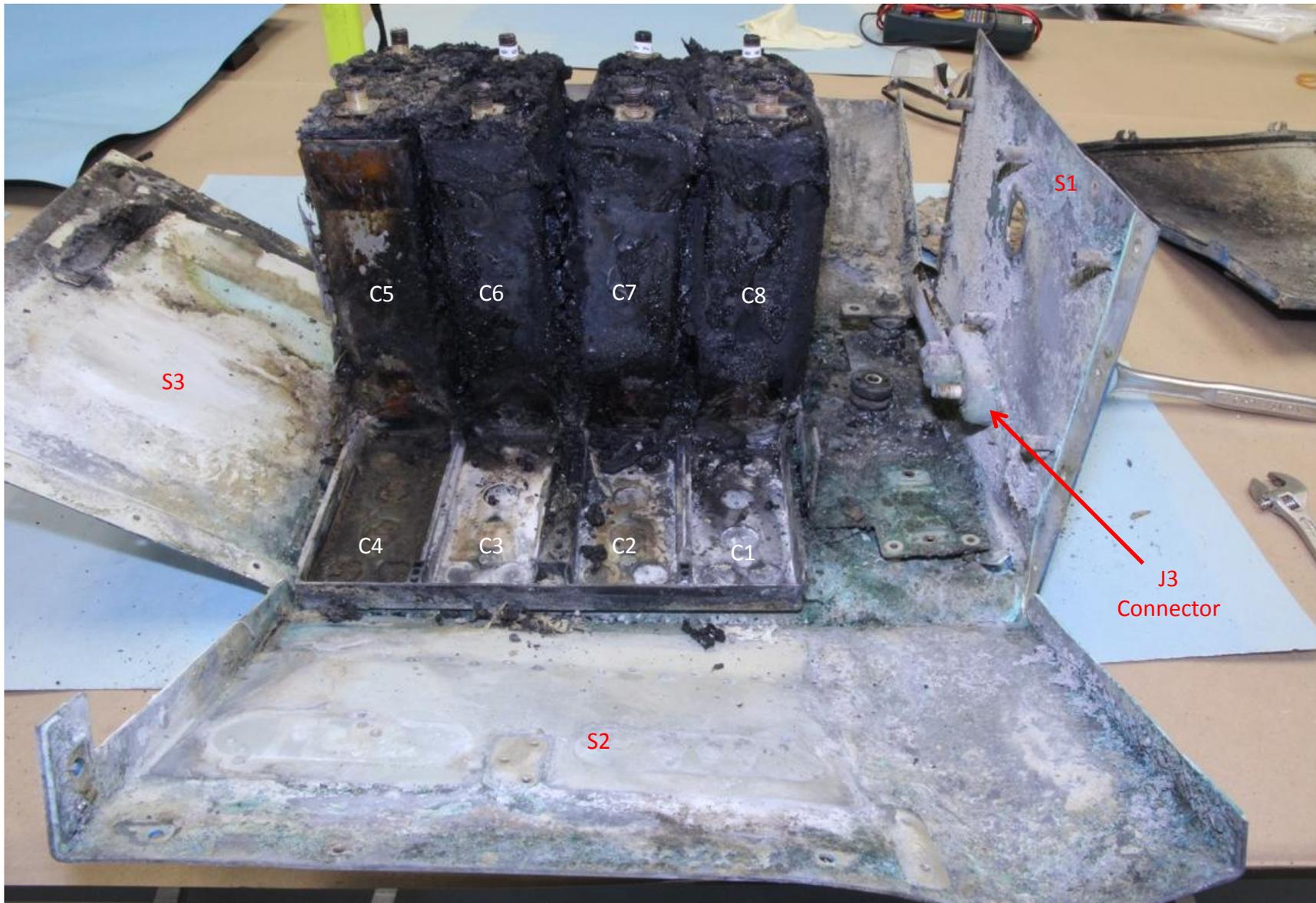
Figure 88. Battery box with C1 through C4 removed (viewed from S2).
