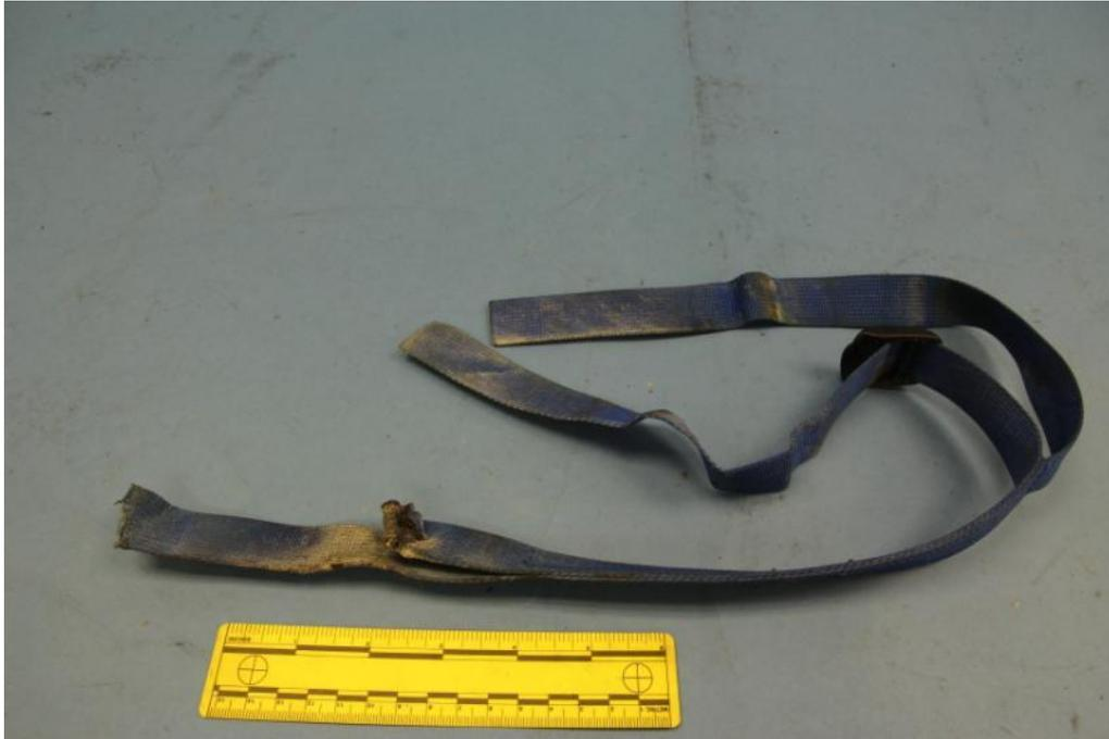
Figure 9. Battery box carrying strap.
