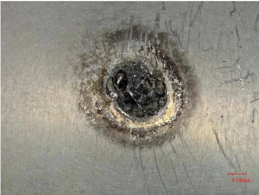
Figure 54. The protrusion on the interior of the battery box, after cleaning (~200X).
