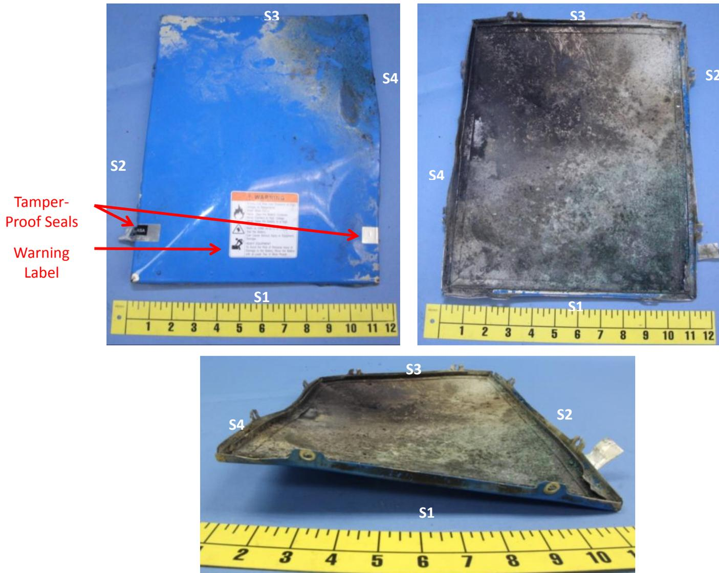
Figure 8. Top and bottom views of the battery box lid showing warning label and seals.
