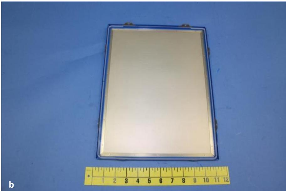
Figure 7. Exemplar, main battery with the battery box lid removed. Photo (a) is a view with the battery box lid removed. Photo (b) is a view of the inside of the battery box lid surface.
