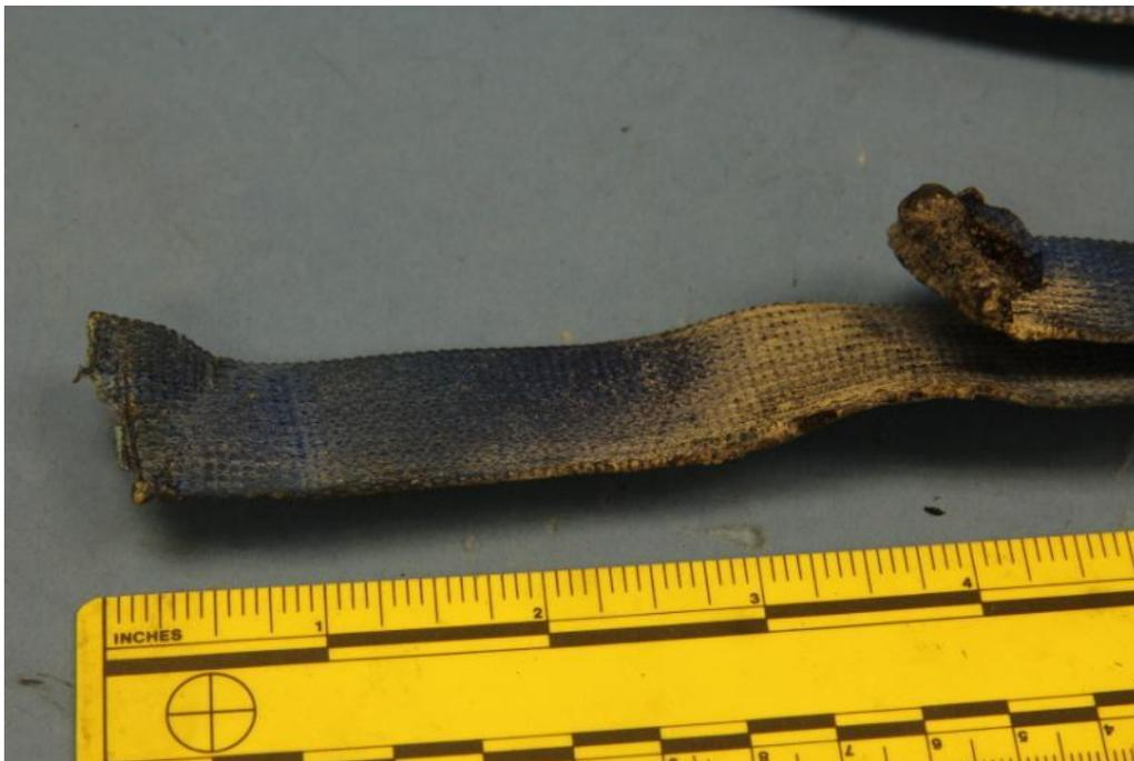
Figure 10. S4 end of the battery box carrying strap.
