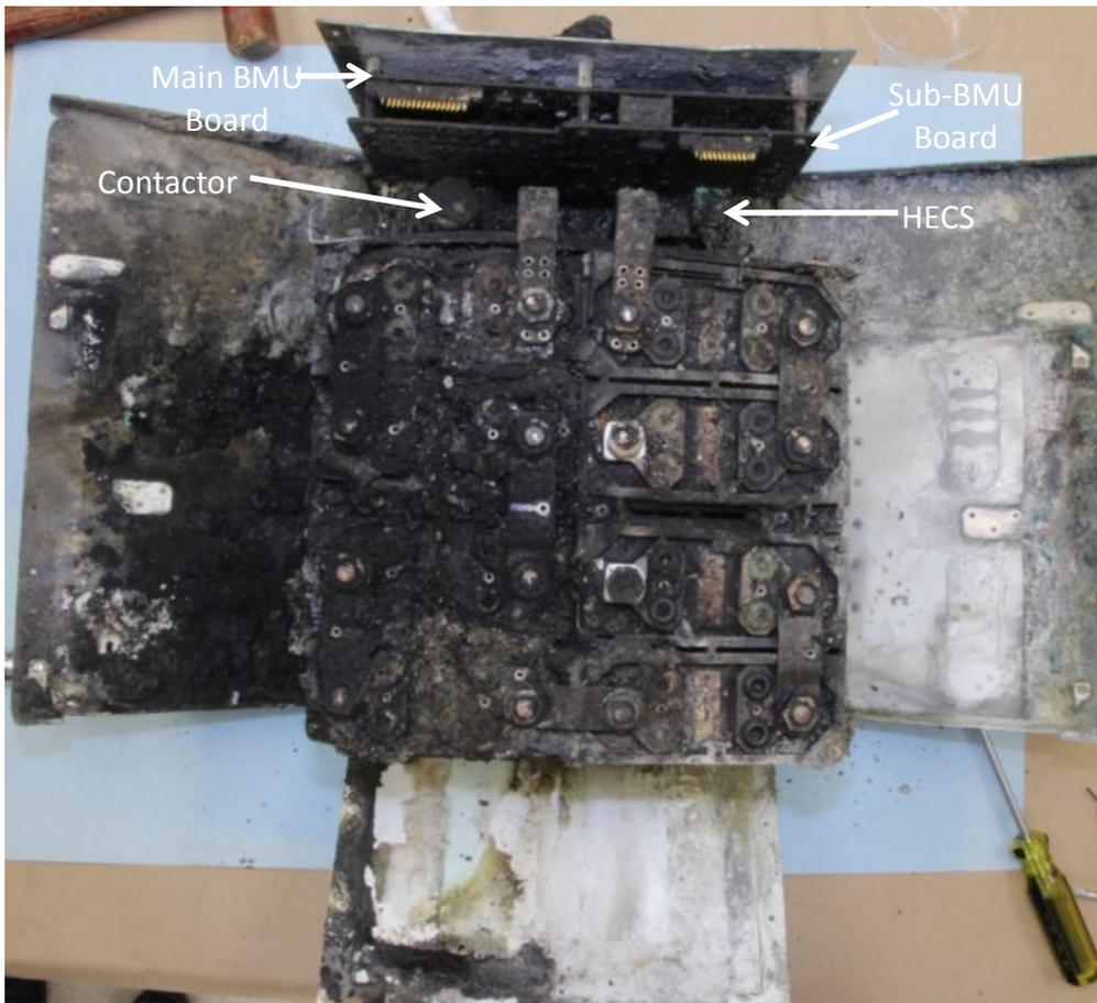
Figure 32. Top view showing the BMU, HECS, and contactor locations.
