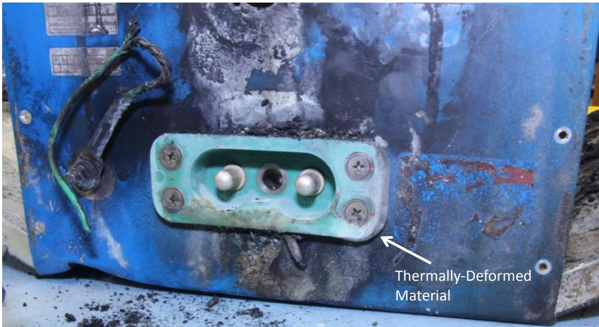
Figure 98. Close-up view of the J3 power receptacle showing thermally-deformed material.
