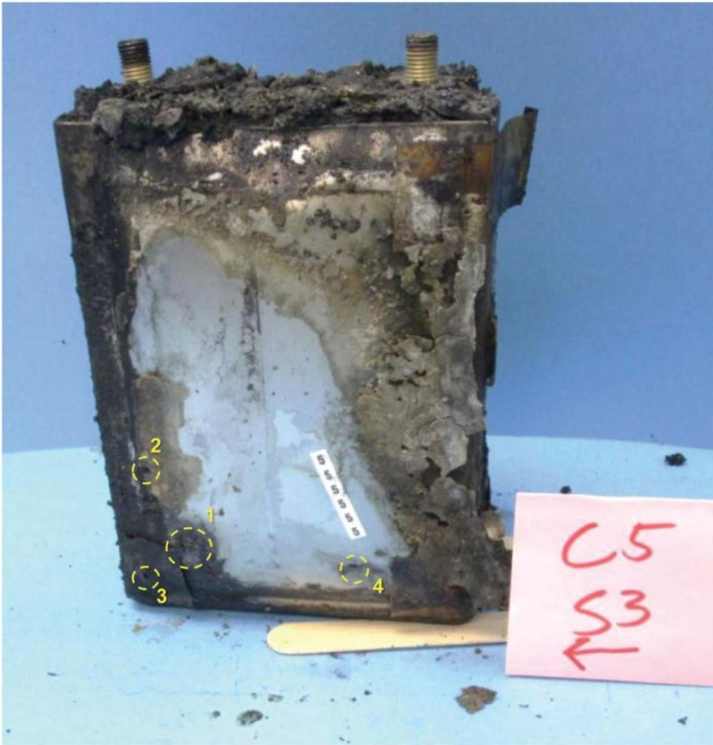
Figure 62. The cell case of C5, facing the interior of S3 of the battery box. Four areas were found that exhibited heavy decomposition deposits about a round hole—these areas are labeled 1 through 4 (circles).
