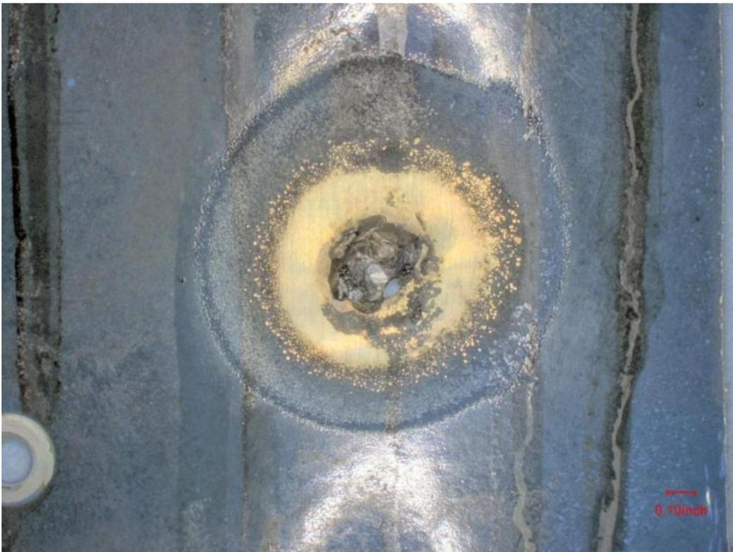
Figure 52. The protrusion on the exterior of the battery box, after cleaning (~50X).
