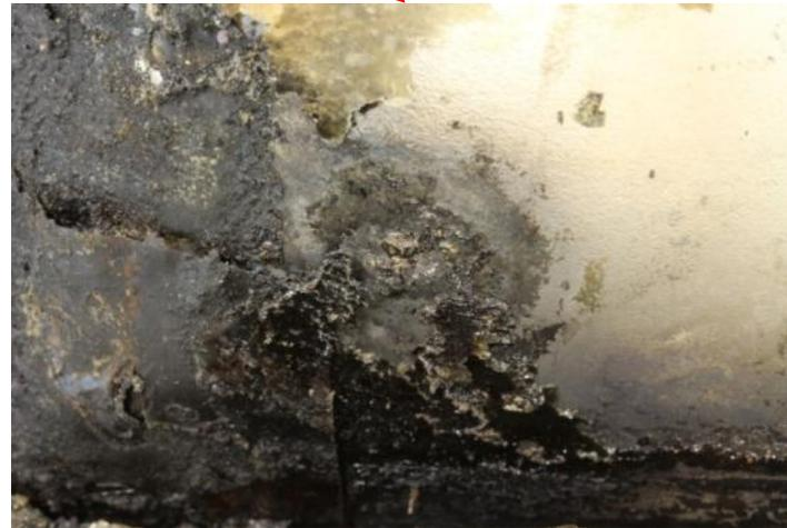
Figure 31. Closer views of a higher-temperature spot consistent with arc damage between C5 and the inside of S3 of the battery box.
