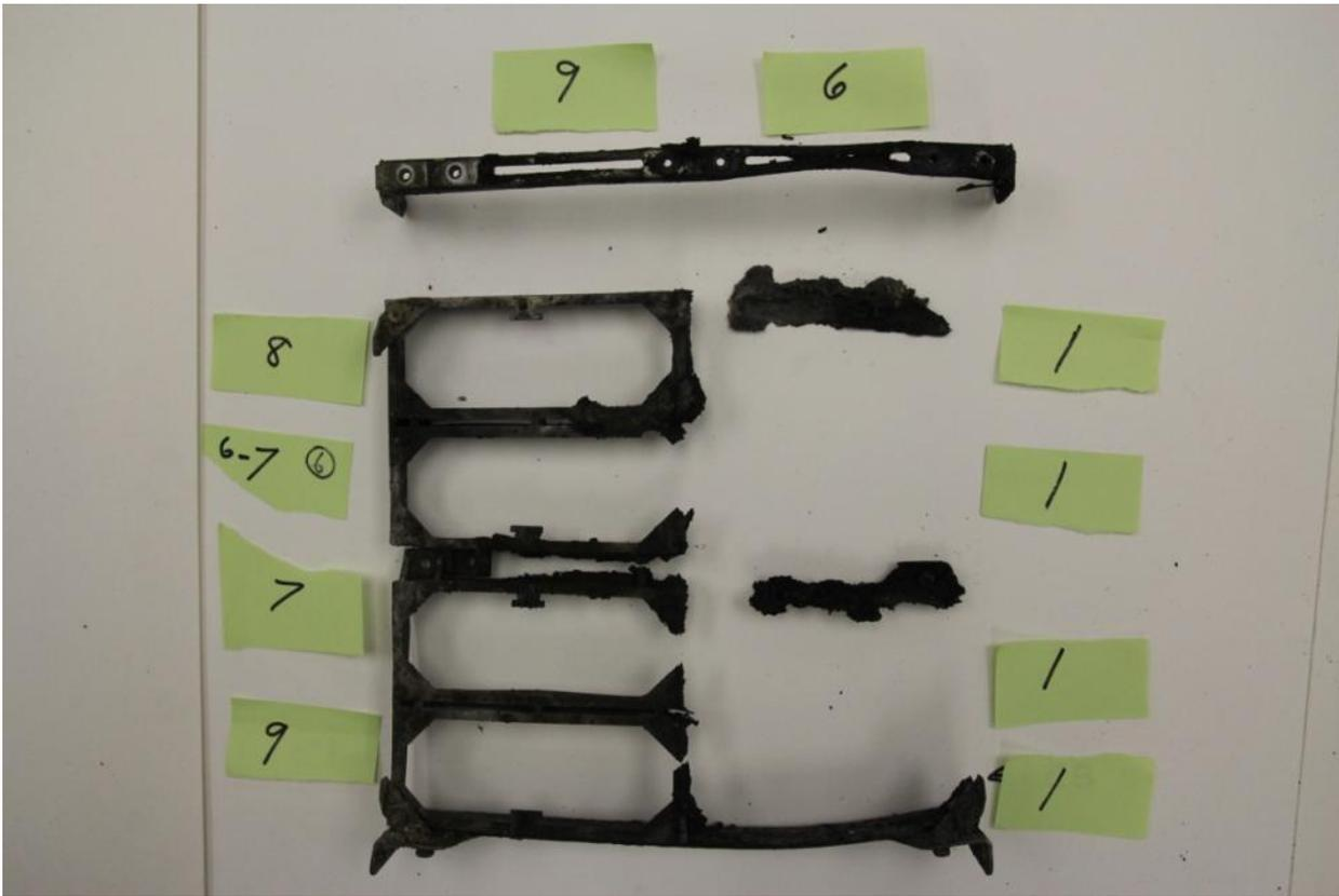
Figure 93. Upper fixation tray and brace bar damage assessment (10 = least damaged, 1 = most damaged).
