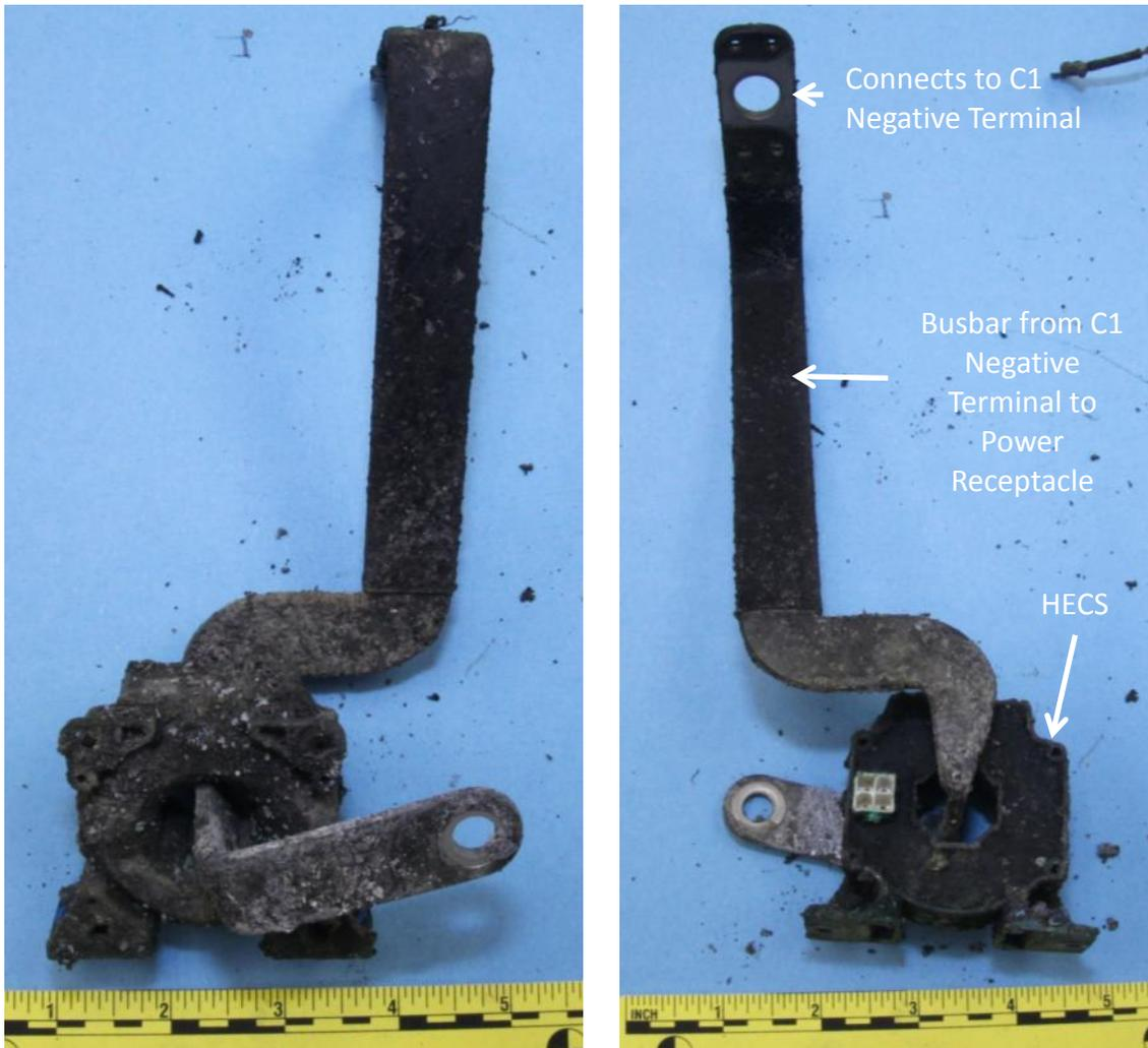
Figure 38. Busbar from C1 negative terminal to power receptacle. The photo on the left shows the side facing the sub-BMU circuit board. The photo on the right shows the side facing C1.
