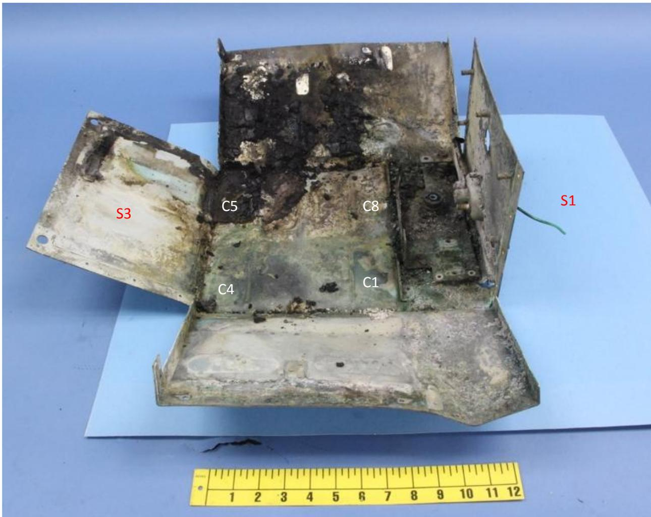
Figure 79. Battery box with all cells removed (viewed from S2).
