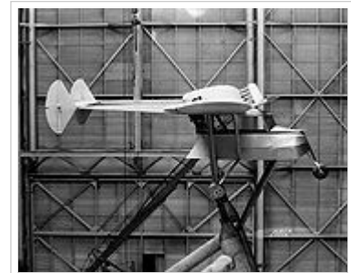
Fred Weick designed the W-1 with tricycle landing gear. It is shown in March 1934.
