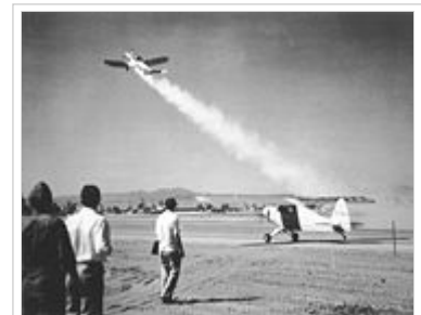
Take-off of America's first "rocket-assisted" fixed-wing aircraft, an Ercoupe fitted with a GALCIT developed solid propellant JATO booster with a thrust of 28 pounds force (125 N). The Ercoupe took off from March Field, California and was piloted by Captain Homer A. Boushey Jr.
