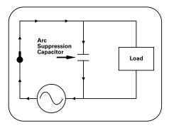
The discharge surge current may be hundreds of amperes for a few nanoseconds or more. To limit such discharge currents, an arc-suppression capacitor should have a certain amount of resistance in series with it. In circuits where there is no dedicated capacitance, however, there still may be sufficient stray capacitance to cause a momentary overcurrent upon contact make. This fact is often overlooked by many circuit designers.
