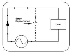
Also, if an arc-suppression capacitor is used across the contacts, this capacitance will discharge itself through the relay contacts.
