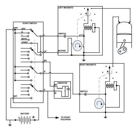
Figure 1. Magneto Circuit OFF
