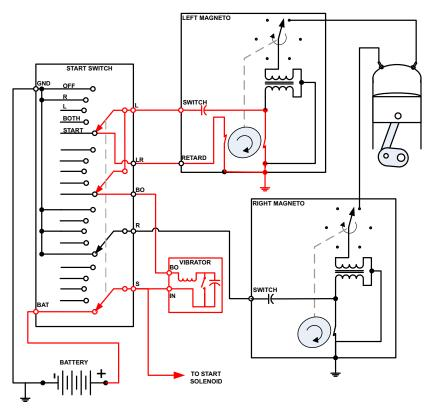
Figure 2. Vibrator Energized
