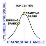
Ignition timing must be advanced to get maximum power output from a combustion engine at high RPM. If we try to start the engine with advanced ignition timing, combustion occurs too early and the engine kicks back and fails to start. Starting ignition can be improved by retarding (delaying) ignition timing until the piston is close to the top of the cylinder on the compression stroke. If ignition occurs too late, the engine won't develop momentum after ignition.
