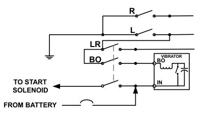
Some switches feature a spring loaded start function while others are designed with a "PUSH-TO-START" feature. Many combinations are available, limited only by the demand for possible start and run combinations.
