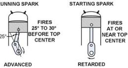
RPM may not turn the magneto fast enough to generate a spark to ignite the fuel in the combustion chamber. That's why impulse couplings or vibrators are used.
