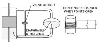
In the ignition system, we use this same principle to generate a surge or "kick" of electrical force (current) across the coil. The current in the coil wants to keep flowing so it builds up voltage across the ends of the coil.
