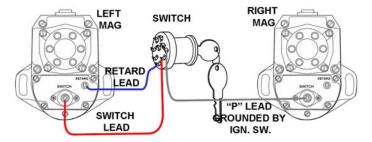
To get a retarded or late spark for starting, the LEFT magneto is assembled with two contact assemblies in it. The "ADVANCE" or "MAIN" contacts are synchronized to the crankshaft timing mark before piston top dead center. The "RETARD" or "START" contacts open a few degrees after the "ADVANCE" or "MAIN" contacts open, depending on engine requirements.
