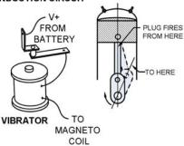
By starting at top center, and throwing a continuous stream, or "shower" of sparks across the spark plug, we increase the likelihood of igniting the fuel mixture in the cylinder. The induction vibrator does exactly this. It is a special form of buzzer which provides about 200 sparking pulses per second!
