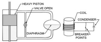
Start the heavy piston down the cylinder and slam the valve shut. The piston wants to keep moving and the pressure built up would burst the valve if the fluid did not have another path to travel into the box containing the rubber diaphragm. The momentum of the piston is converted into a force which bends the diaphragm upward.
