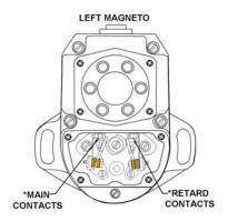
NOTE: \*MAIN AND RETARD BREAKERS MAY BE REVERSED DUE TO MAGNETO ROTATION.
