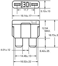
Catalog Symbol: ATC Fast-Acting Ampere Rating: 1 to 40 Amperes Voltage Rating: 32 Volts DC (or less) Interrupting Rating: 1,000 Amperes Agency Approvals: U.L. Recognized, (3-40A) Guide JFHR2, File E56412
