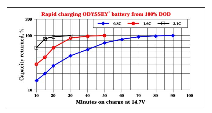
$<sup>^6</sup>$  The magnitude of the inrush is defined in terms of the rated capacity ( $C_{10}$ ) of the battery. Thus, a  $0.8C_{10}$  inrush implies a current that is 80% of the rated capacity, or 80A for a 100Ah battery. Similarly, a  $1.6C_{10}$  inrush on a 100Ah battery means that the charge current inrush is 160A ( $1.6 \times 100$ ).
