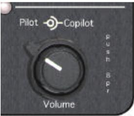
The pilot volume control knob adjusts the loudness of intercom and music in the pilot’s head-phones only. It has no effect on selected radio audio levels. The copilot volume control adjusts the loudness of the intercom and music in the copilot headset. The passenger volume is also adjusted by the copilot volume control. Most general aviation headsets have a built-in volume
