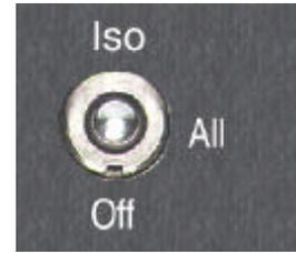
Unit power is turned on and off by the mode selector switch. In the OFF or “FAIL-SAFE” position, the pilot is connected directly to Com 1 allowing transmit and receive capability regardless of unit condition. Any time power is removed or turned OFF, the audio selector will be placed in the fail-safe mode. The switch is a 3-position mode switch that allows the pilot to tailor the
