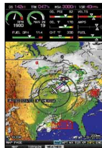
How far can you go? Graphical range rings are based on real-time fuel flow calculations
