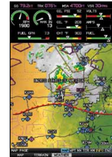
Available XM WX® data includes NEXRAD, satellite mosaic, Airmets, Sigmet and frontal boundaries 2
