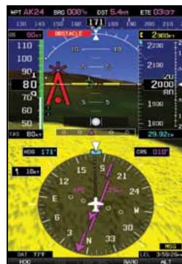
As traffic or towers get closer, their symbols grow larger on SVX display
