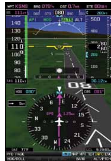
SVX shows runway surfaces, numbers and thresholds in virtual 3-D
