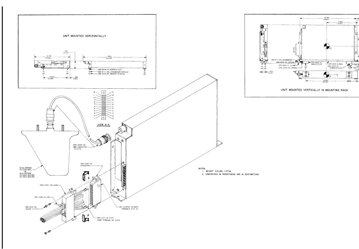
FIGURE 2-1 KN 63 OUTLINE AND MOUNTING DRAWING Dwg. No. 155-05315-0000, R-AA
