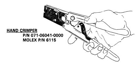
Close crimpers until ratchet begins to engage. Then insert terminal into jaws from the back side. (See the following; Figure 2-1). For 24 to 30 AWG wire, it will be necessary to start the crimp in jaw A and then complete in jaw B.
