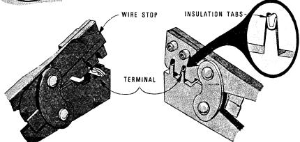
Terminal is in the correct position when insulation tabs are flush with outside face of crimp jaws.
