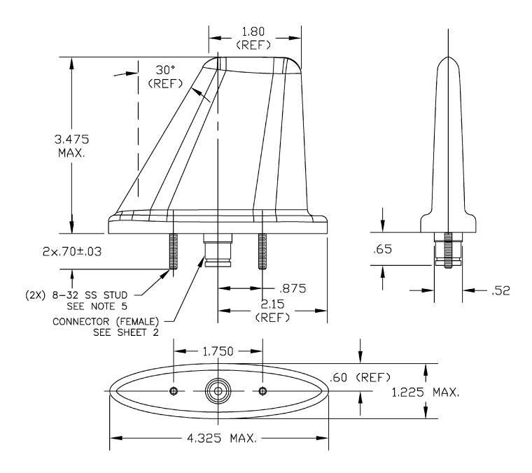
FIGURE 2-7 KA 61 INSTALLATION DRAWING (Page 1 of 2)
