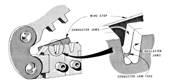
Squeeze the handles until the crimp jaws close and the ratchet releases.
