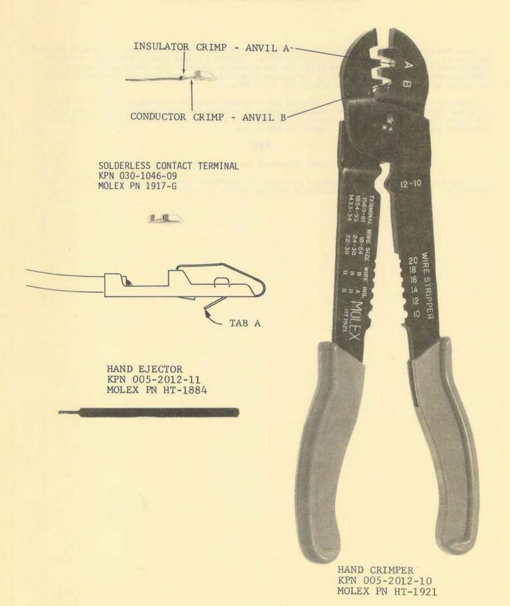
FIGURE 2-1 CRIMPING TOOL (Dwg. No. 696-2151-00, R-0)
