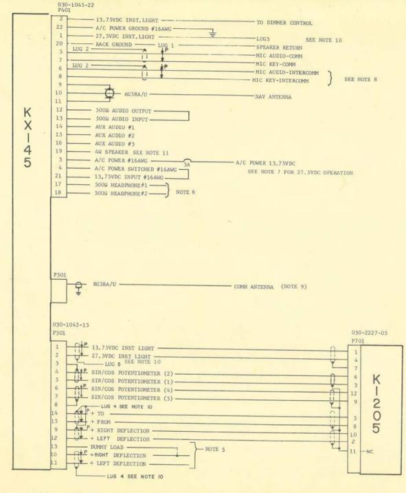
NOTE 1. UNLESS NOTED, ALL WIRES TO BE #24AWG MINIMUM.
