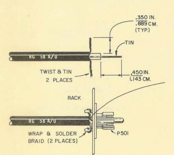
Separate braid into two equal parts and fold out to sides of coax. Strip center conductor and trim braid as shown.
