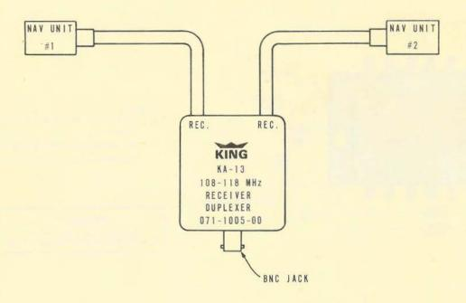
17 IN. IS % WAVELENGTH OF COAX CORRECTED FOR POLYETHYLENE DIELECTRIC
