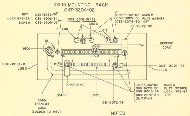
LTHE FOLLOWING TOOLS ARE REQUIRED FOR CONSTRUC CABLE HARNESS FOR CONN. P301 AND P401. HAND CRIMPING TOOL - MOLEX HT - 1921 TERMINAL EXTRACTOR TOOL - MOLEX HT - 1884
