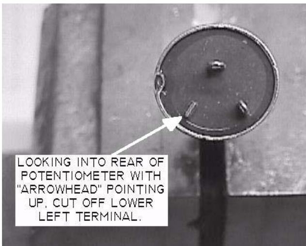
5. Use electronic grade solder (60/40 or 63/37 tin-lead, rosin core) to attach wires to terminals on the control potentiometer. Hook wires over the terminals and solder.
