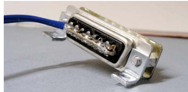
Figure 18-15. DIY D-Sub Ground Block, Rear View
