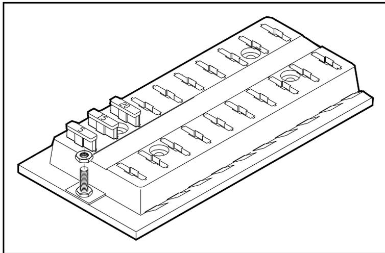
Figure 10-1. Multi-Slot Plastic Fuseblock.
