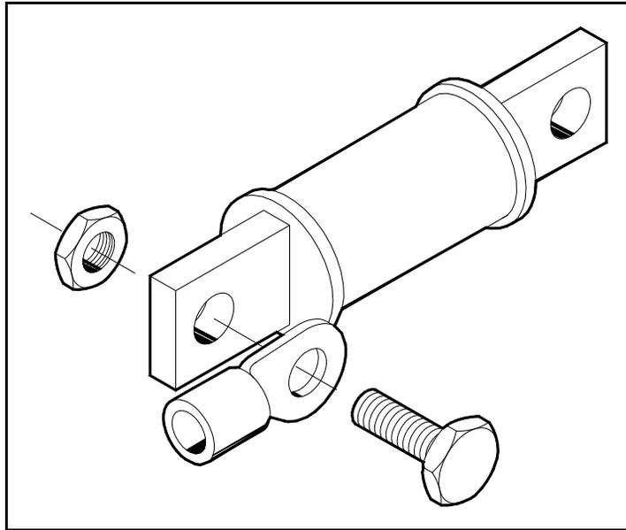
Figure 10-2. In-Line Fuse Adaptation of the JJJ/JJS Series Cartridge Fuses.
