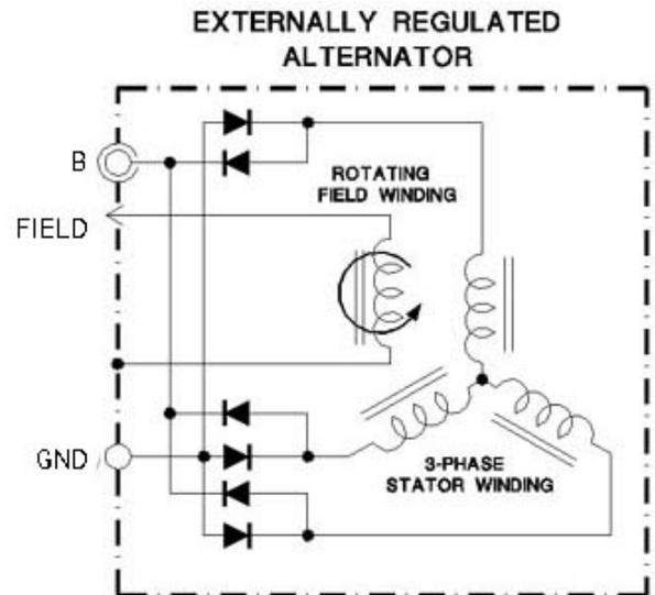
Figure 3-5. Schematic of Externally Regulated Alternator
