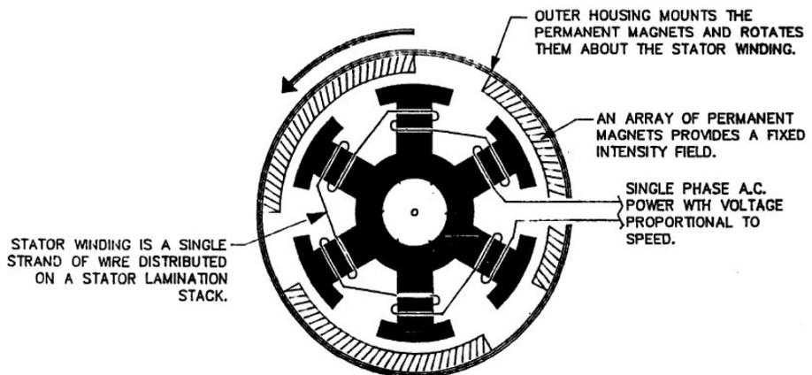
Figure 3-11. Major Components of the PM Alternator
